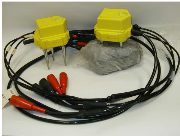
Figure 3: 3C geophones. Geophone coupling to hard surfaces like the Edwards limestone is a concern with spiked geophones. As a solution, when solid limestone is encountered, a block of modeler's clay is used as a base.
