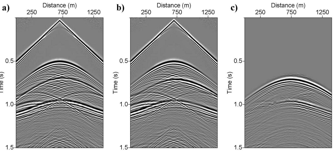
a) Difference data with 70% randomly missing traces. b) Reconstructed difference data. c) The reconstruction error section.
