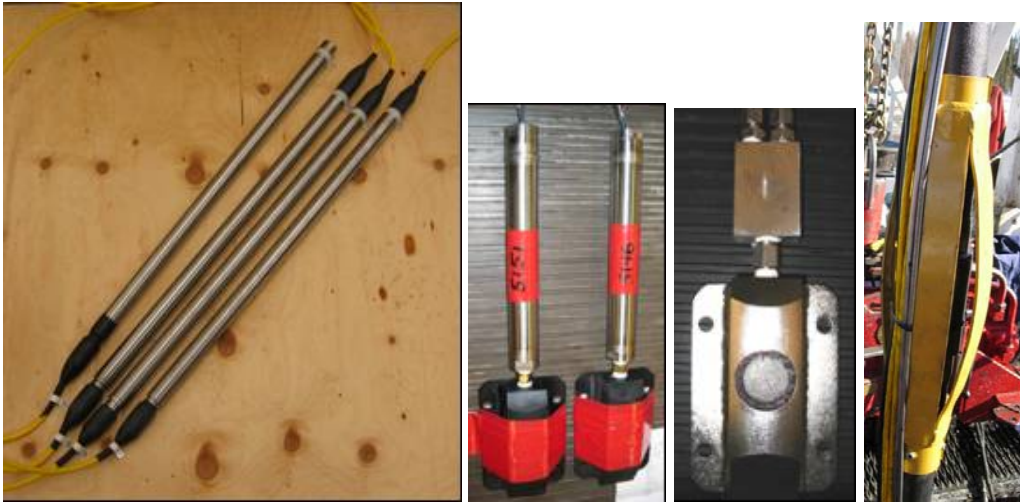
Figure 1. Left to right: geophone sondes, pressure/temperature gauges, downhole fluid sampling ports, a centralizer covering a joint tubing.
