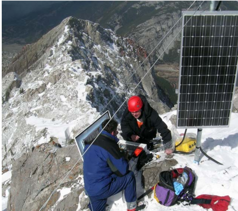
Fig. 2. Installing the seismic monitoring system on South Peak of Turtle Mt., Alberta.
