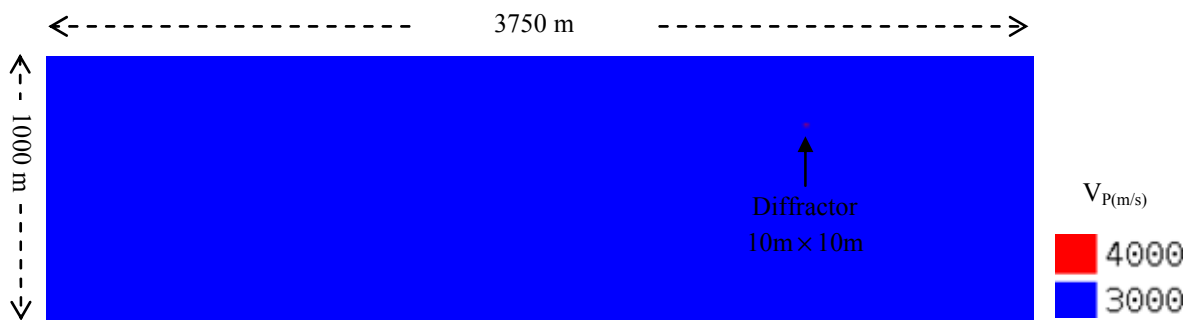
Figure 1: A scatter point in a homogenous medium. This shows the P-wave velocities.
