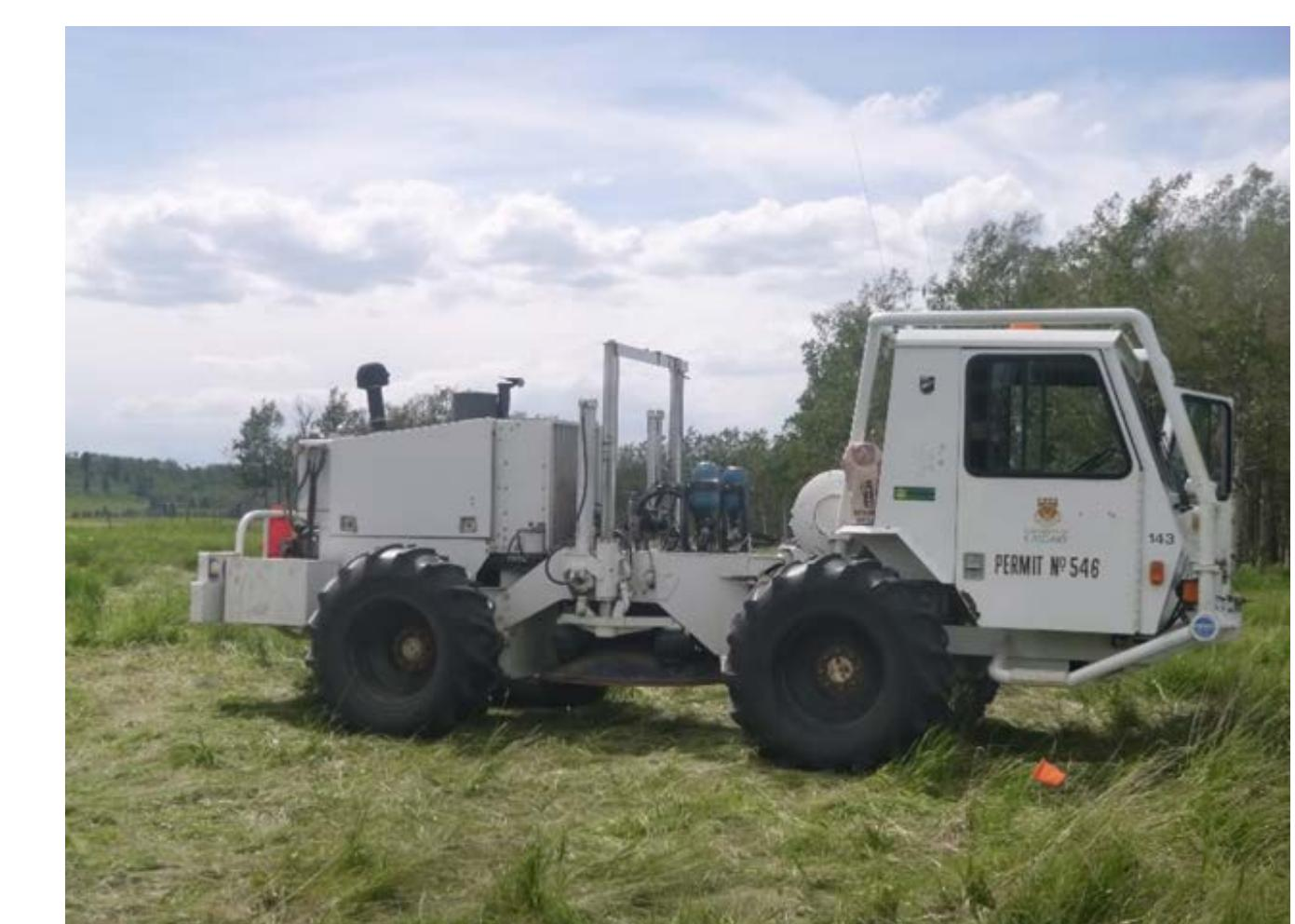
FIG. 5. IVI Envirovibe (sweep 10-200Hz over 16 seconds, two sweeps per source point).
