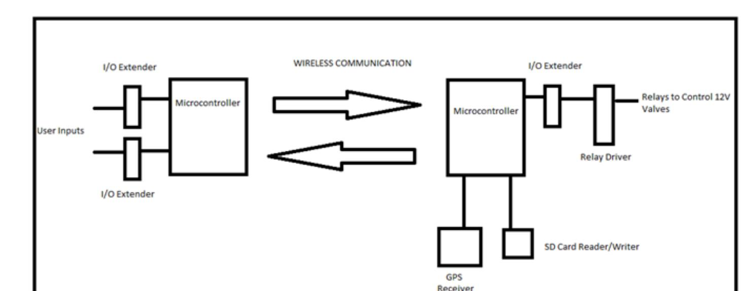
FIG. 7. Wireless thumper controller concept.
