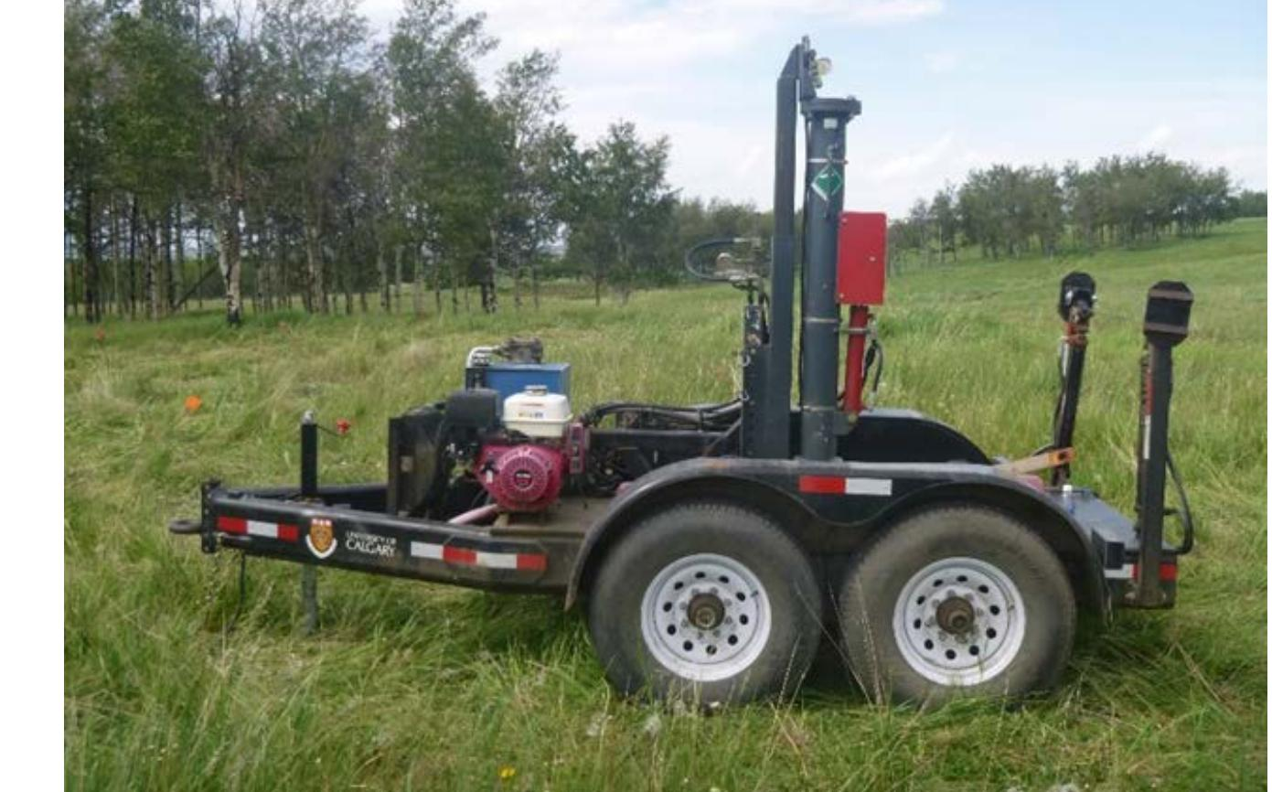
FIG. 6. Shear wave thumper.
