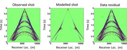
FIG. 3. The data residual is the difference between the observed and modelled shots.
