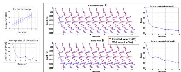
FIG. 7. Evolution of the inverted velocity in the calibration and blind wells. We increased the frequency range 1 Hz each iteration starting with 1-5 Hz.
