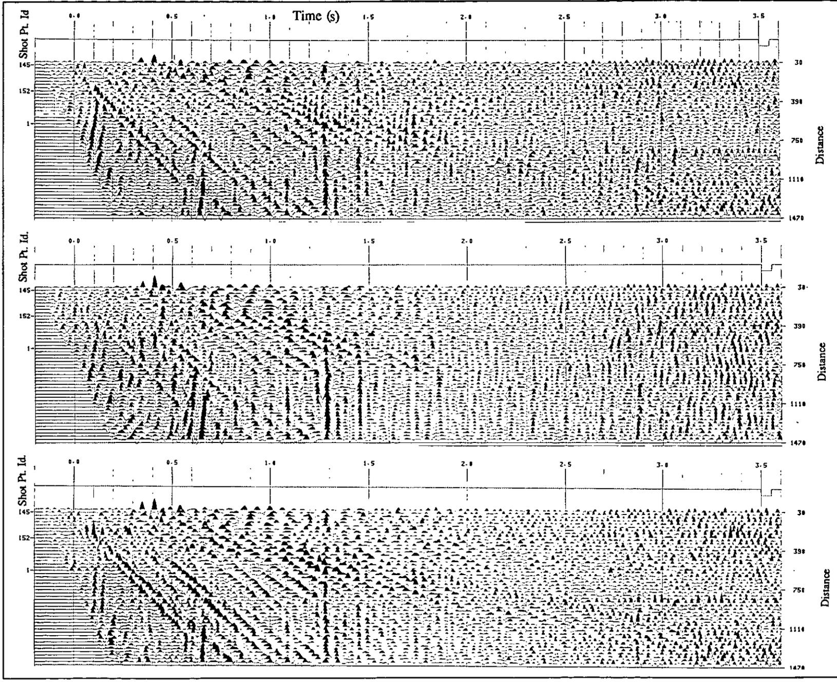
**Figure 12** Common offset stacks for Jumping Pound P-SV data a) no pre-stack spatial filtering b) f-k filtered c) weighted median filtered.
