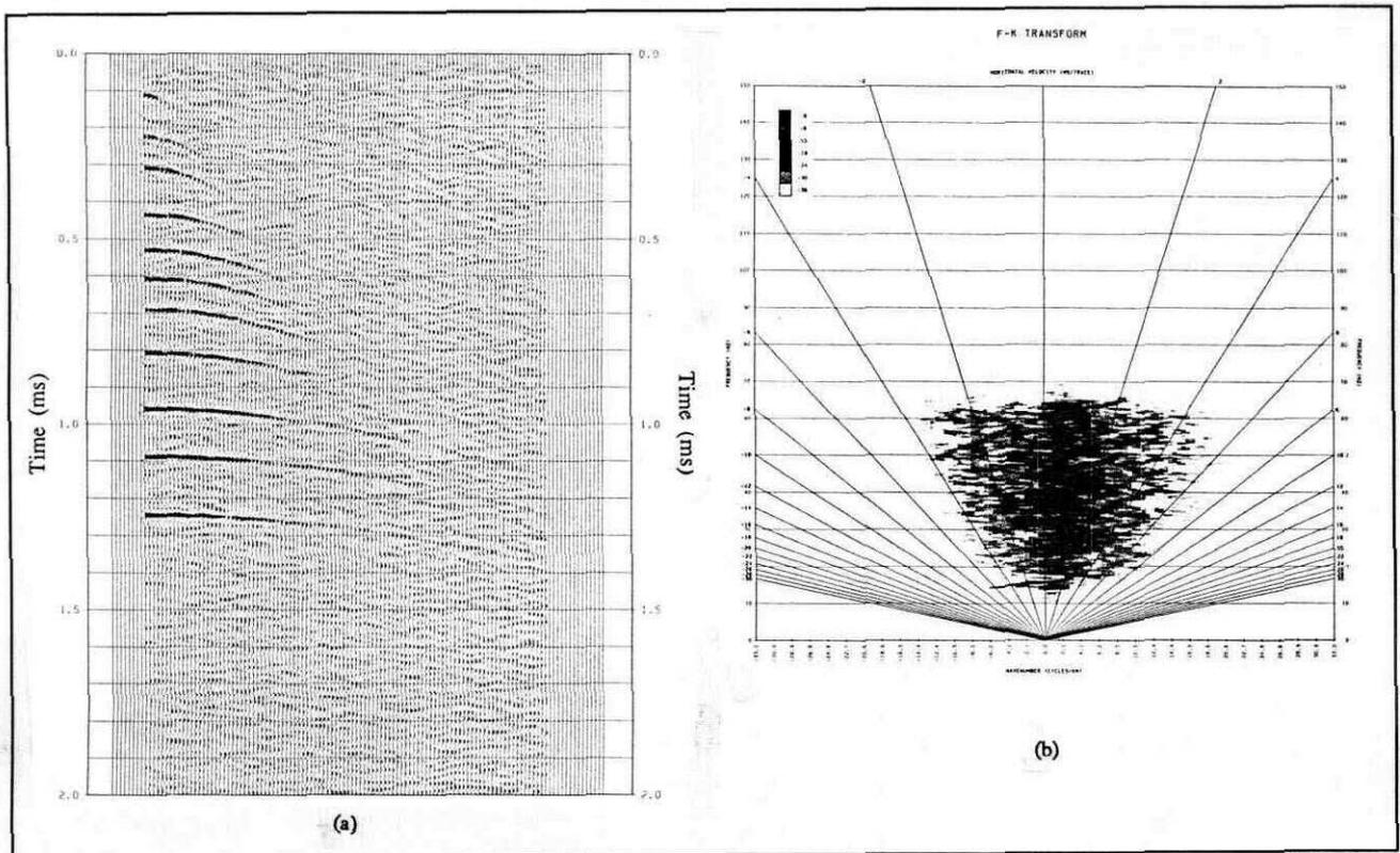
**Figure 7** Synthetic shot gather with random noise added after f-k weighted median with  $\pm 4$  ms/trace reject a) time domain b) f-k transform
