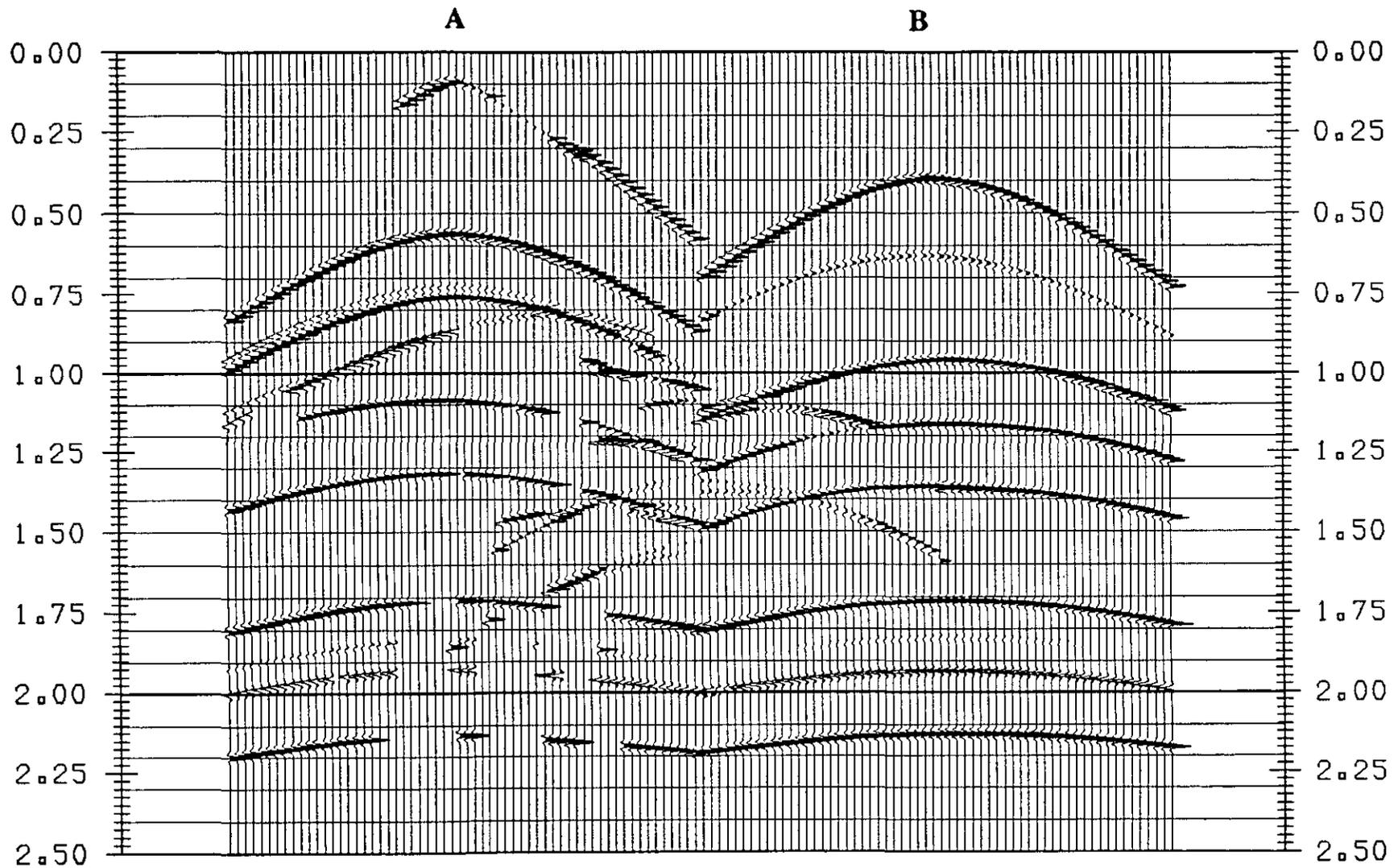
FIG. 13. Sample synthetic P-P shot records from the western(A) and the eastern(B) limbs of the Triangle Zone model in Figure 7.
