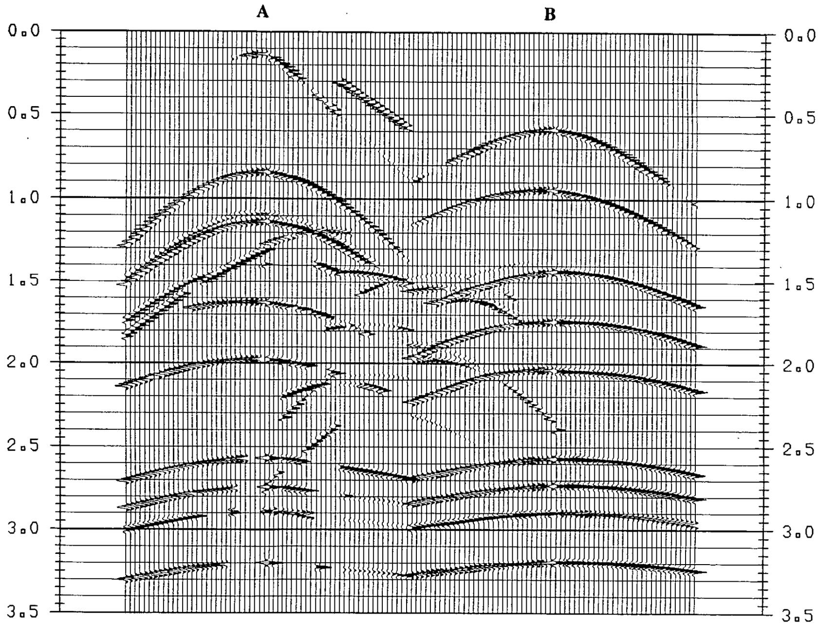
FIG. 16. Examples of the P-SV shot records from the western(A) and the eastern(B) limbs of the Triangle Zone model. Note polarity reversal on one side of the spread.
