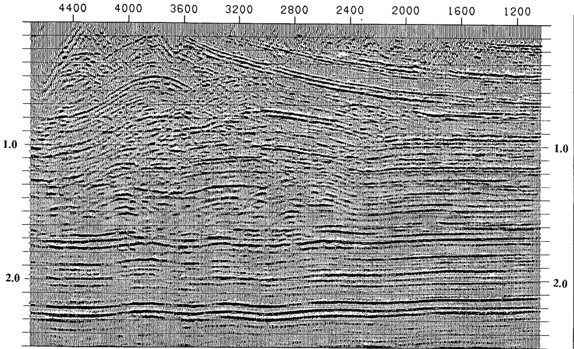
FIG. 5. The final section (DMO was not applied to this section).
