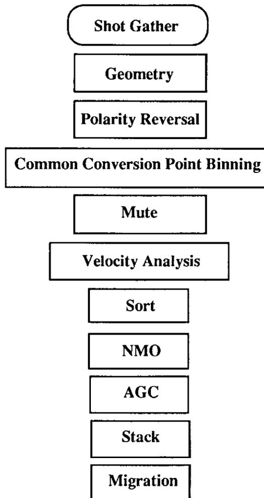
FIG. 15. Processing flow chart for the synthetic P-SV data
