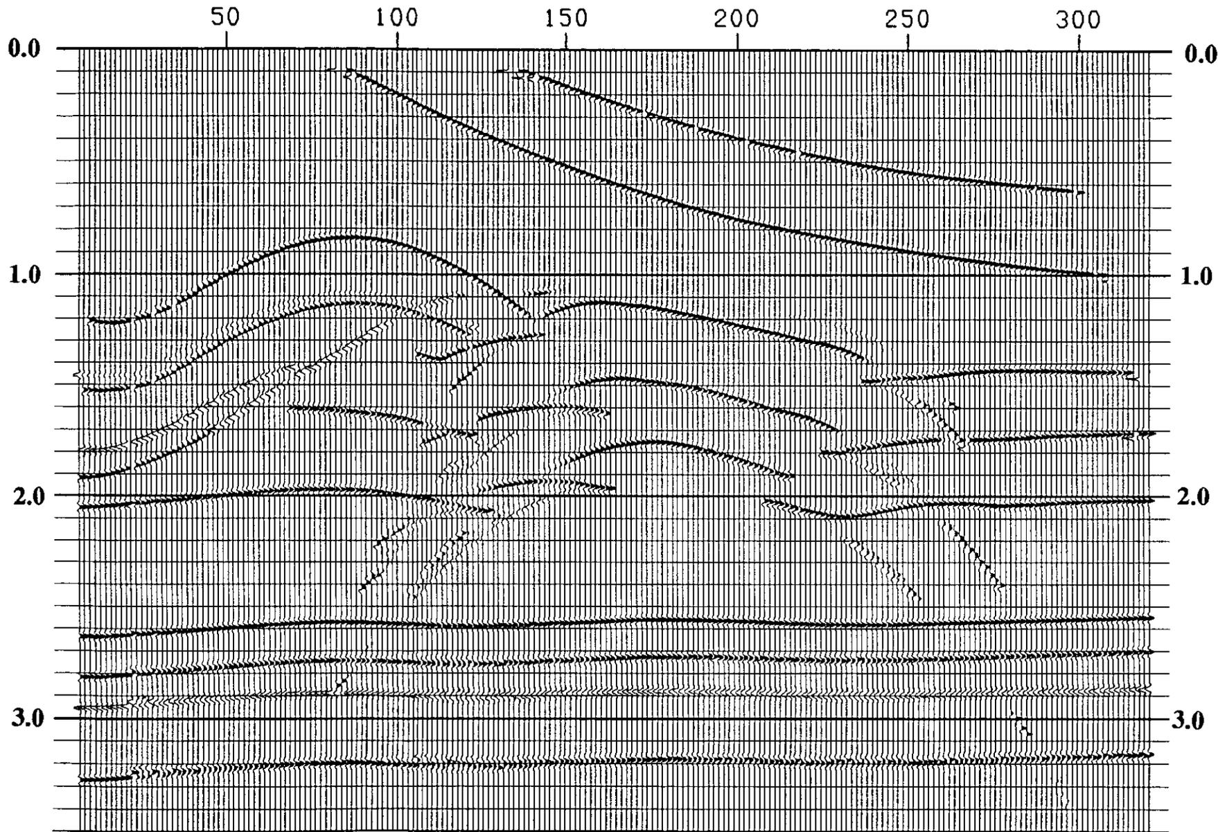
FIG. 17. A P-SV stack section using the processing flow in Figure 15.
