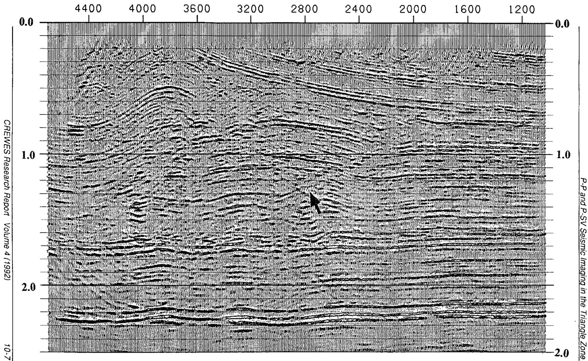
FIG. 4. A DMO corrected section after phaseshift migration, band pass filter and KLSTAK.
