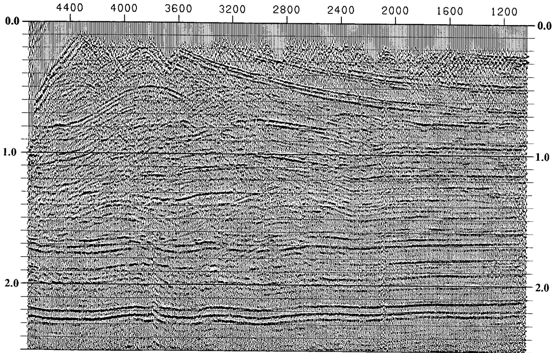
FIG. 3. A final stack section produced by the processing flow in Figure 2.
