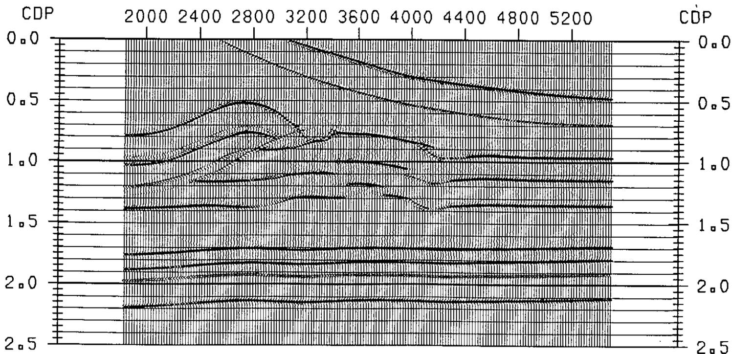
FIG. 9. A F-K migrated section of the zero-offset synthetic seismic section.
