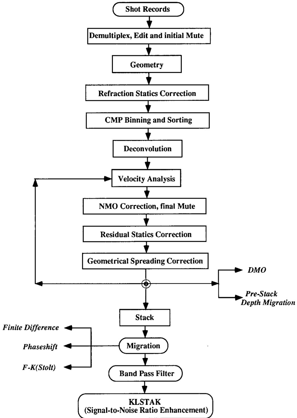
FIG. 2. Processing flow chart for the seismic line FTC-002B
