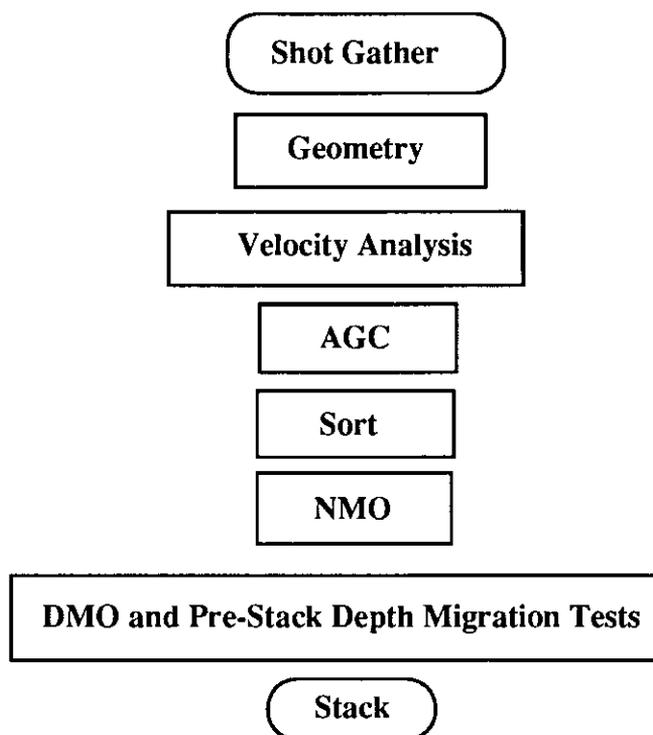
FIG. 12. Processing Flow Chart for the synthetic P-P data
