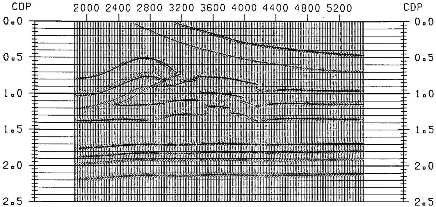
FIG. 10. A F-D migrated section of the zero-offset synthetic seismic section.
