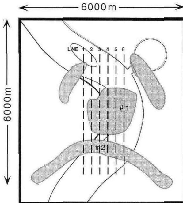
FIG. 9. Schematic diagram of the rugose model with shaded areas indicating rugosity. Area #1 is 10 m to 20 m deep and area #2 is 150 m deep.
