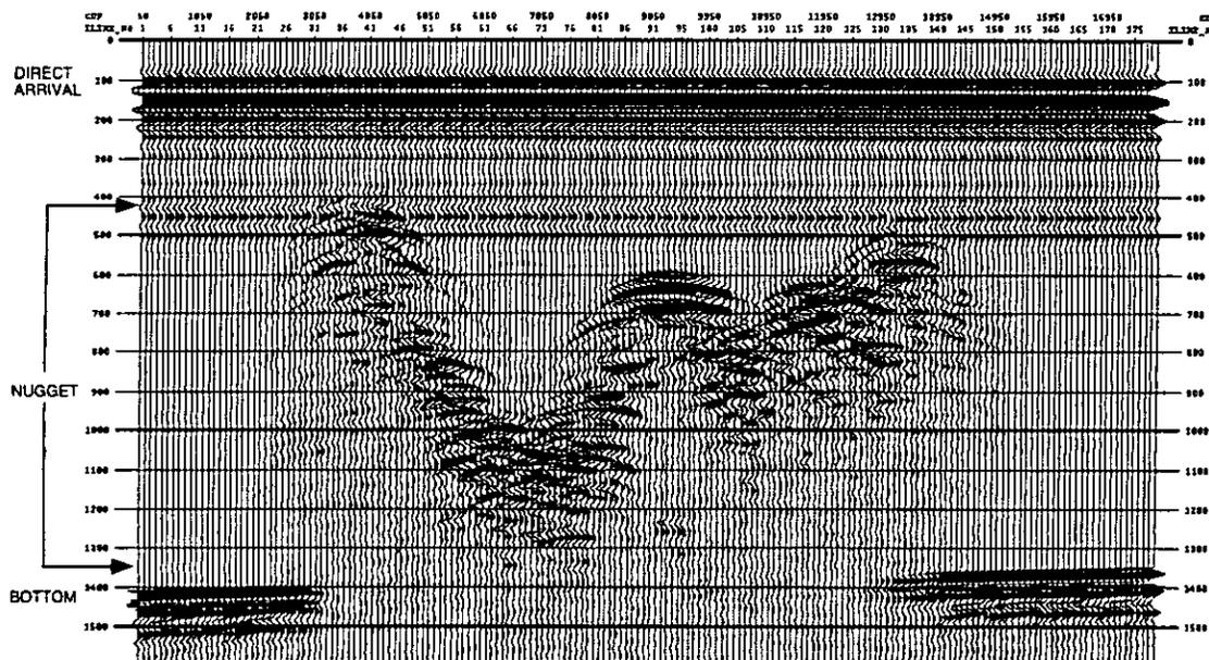
FIG. 6. P-P survey from line 50 over the center of the nugget.
