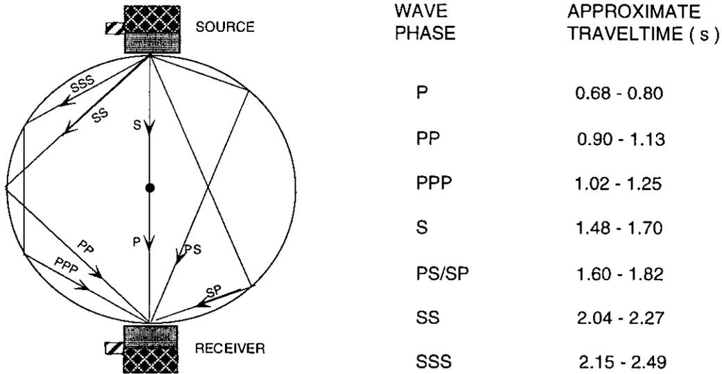
FIG. 3. The diagram on the left shows some of the possible ray paths through the phenolic sphere. The table on the right shows the approximate traveltimes for the various wave phases.
