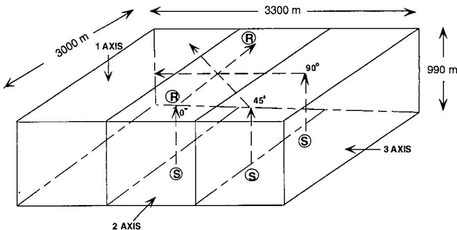
FIG. 13. Diagram of the azimuthal anisotropic model showing the experimental setup .
