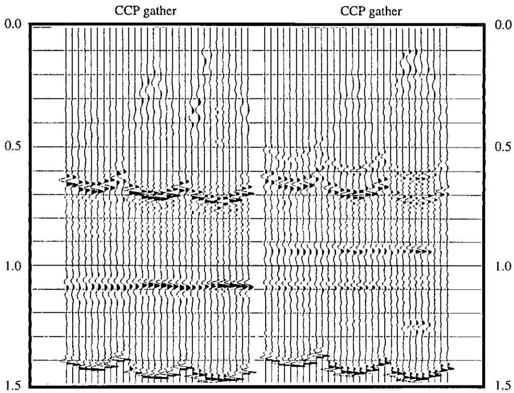
FIG. 12. Example of  $P$ - $SV$  normal moveout correction using standard hyperbolic equation
