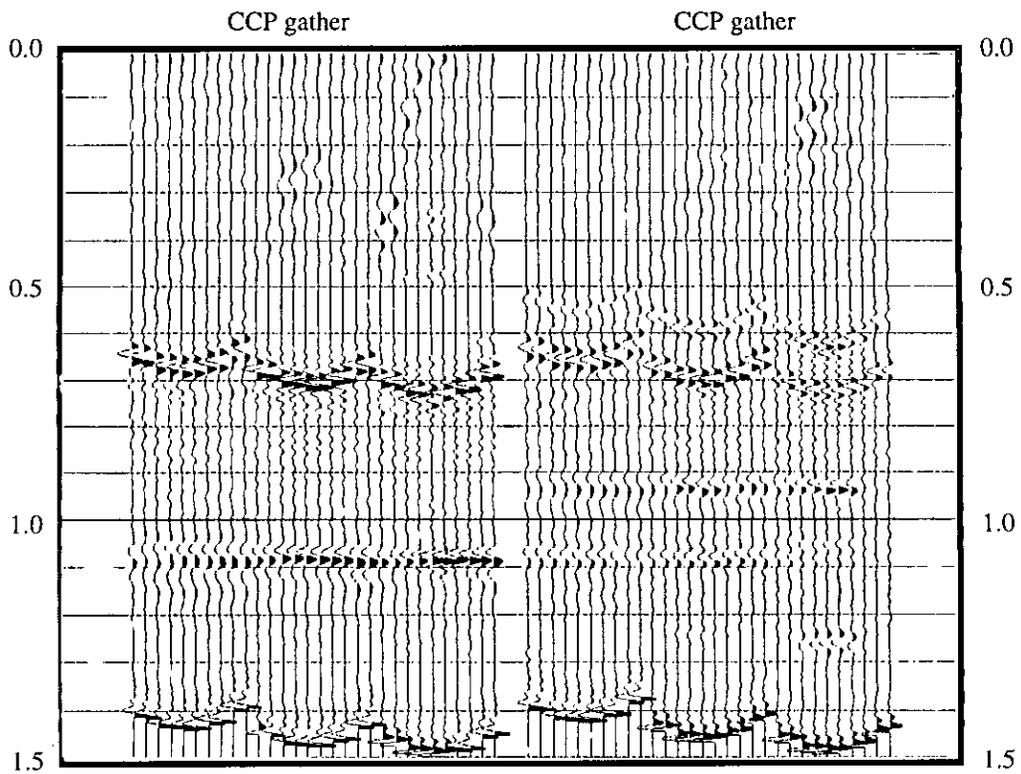
FIG. 13. Example of  $P$ - $SV$  normal moveout correction using time-shifted hyperbolic equation
