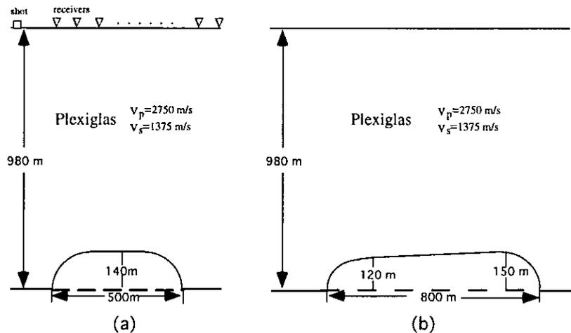
FIG. 2. Cross-sections of the model in receiver-line (a) and shot-line (b) directions across the center of the model.
