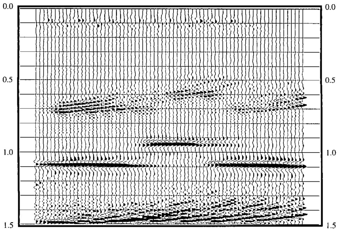
FIG. 19. Example section of *P-SV* migrated data in receiver-line direction after interpolation of the empty traces.
