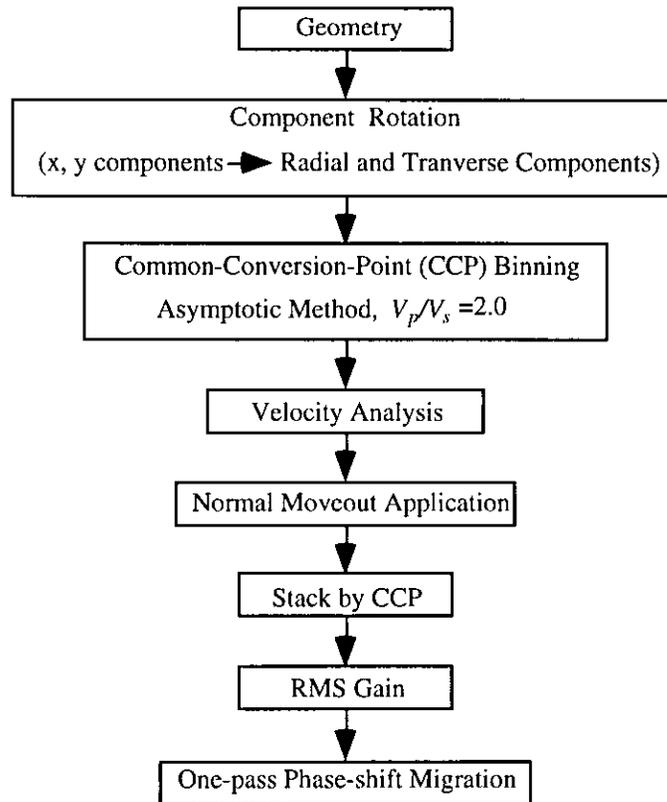
FIG. 5. Flow chat for 3-D isotropic *P-SV* processing.
