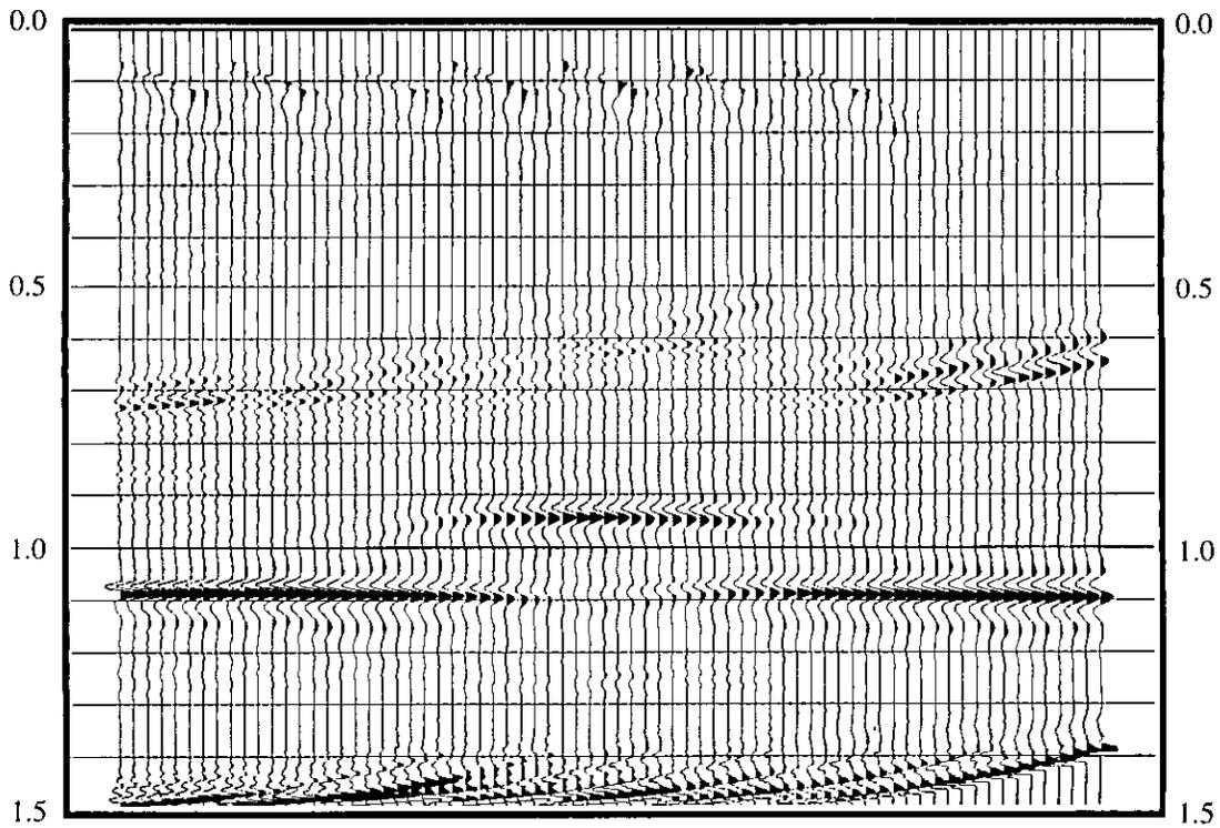
FIG. 17. Example section of *P-SV* stacked data in receiver-line direction with optimum bin size 33.3 m, then resample the data with bin size 25 m.
