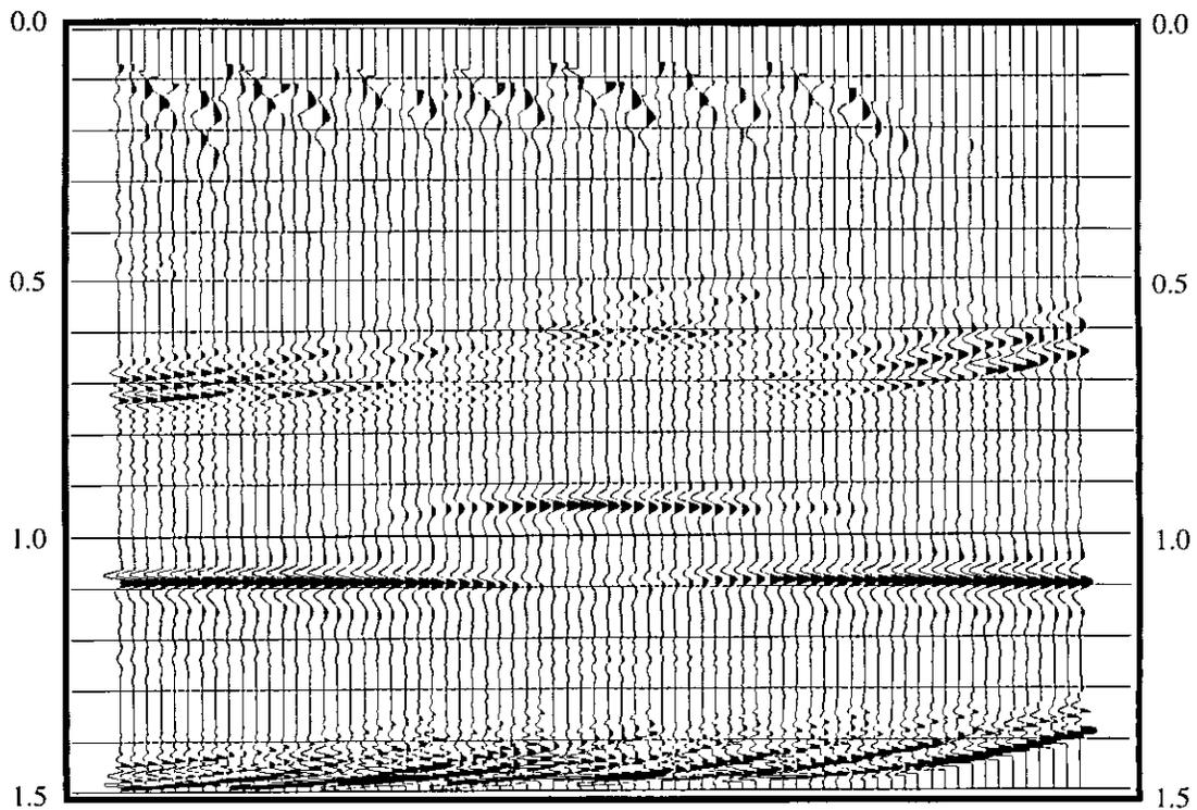
FIG. 15. Example section of  $P$ - $SV$  stacked data in receiver-line direction with bin size 25 m, after interpolation of the empty traces.
