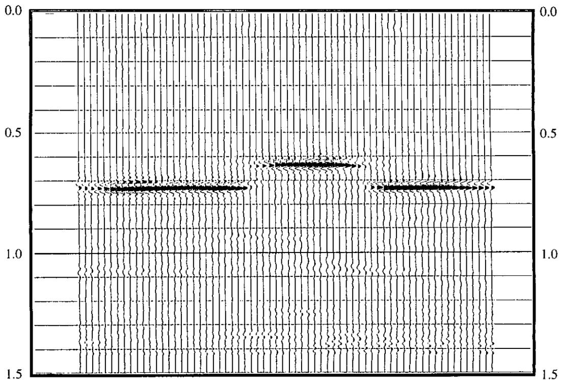
FIG. 23. Example section of  $P$ - $P$  migrated data in receiver-line direction with bin size of 25 m.
