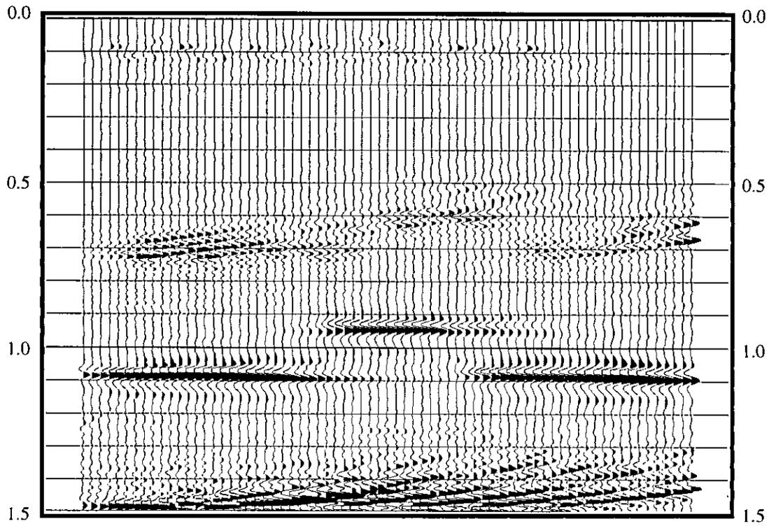
FIG. 20. Example section of *P-SV* migrated data in receiver-line direction with optimum bin size 33.3 m, after interpolating the data with bin size 25 m and migrating this data set.
