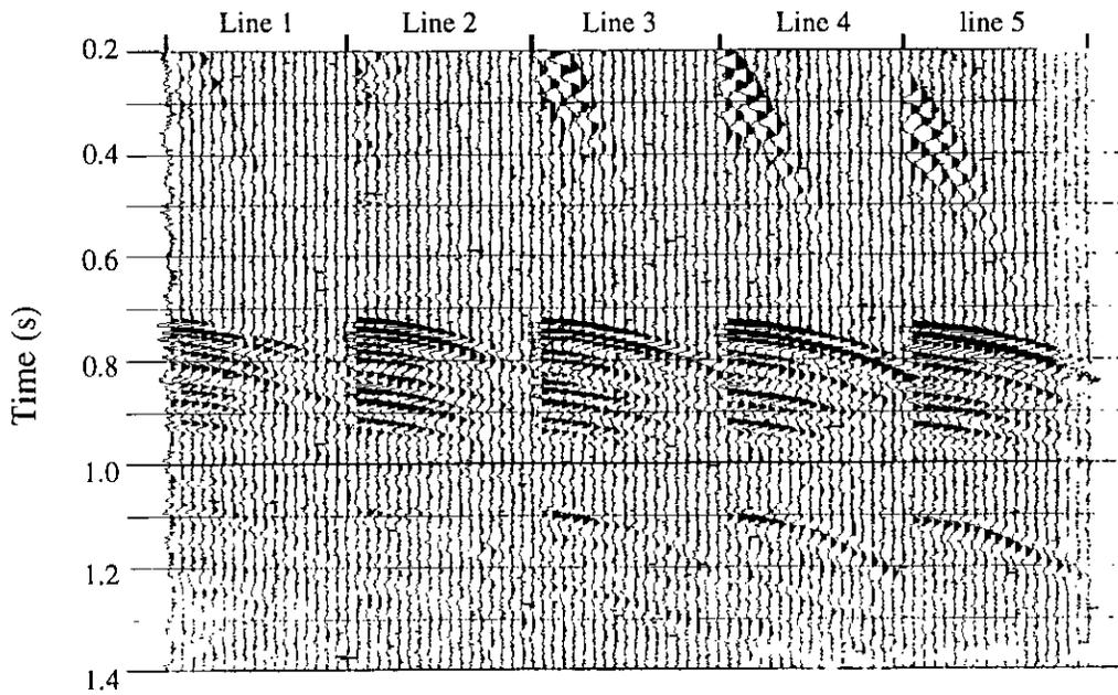
FIG. 7b. Example of cross-line component *P-SV* data. Shot was at station 1 on shot-line 1
