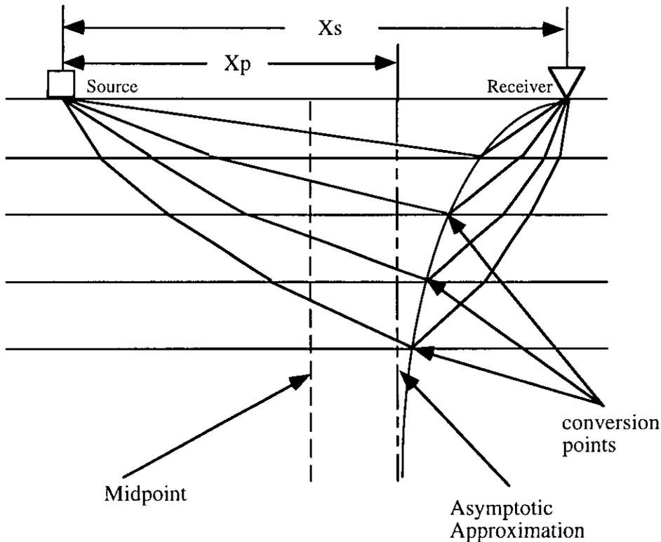
FIG. 9. Schematic diagram of asymptotic common conversion point (CCP) binning.
