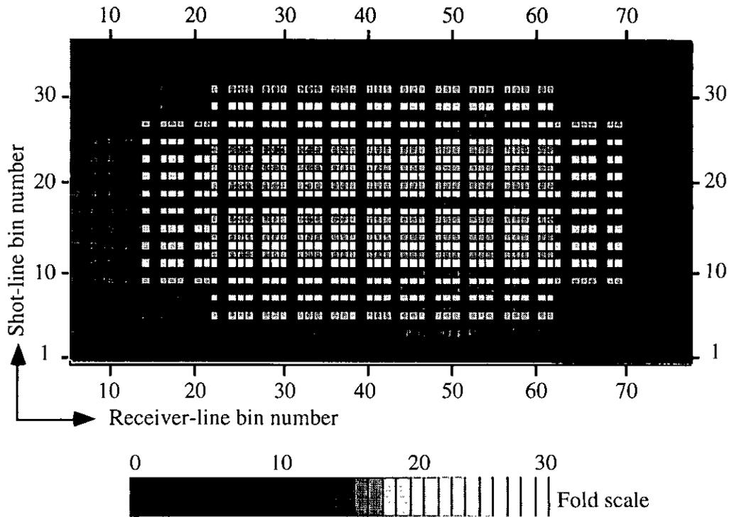
FIG. 10. Fold map of asymptotic common conversion point binning with bin size 25 m
