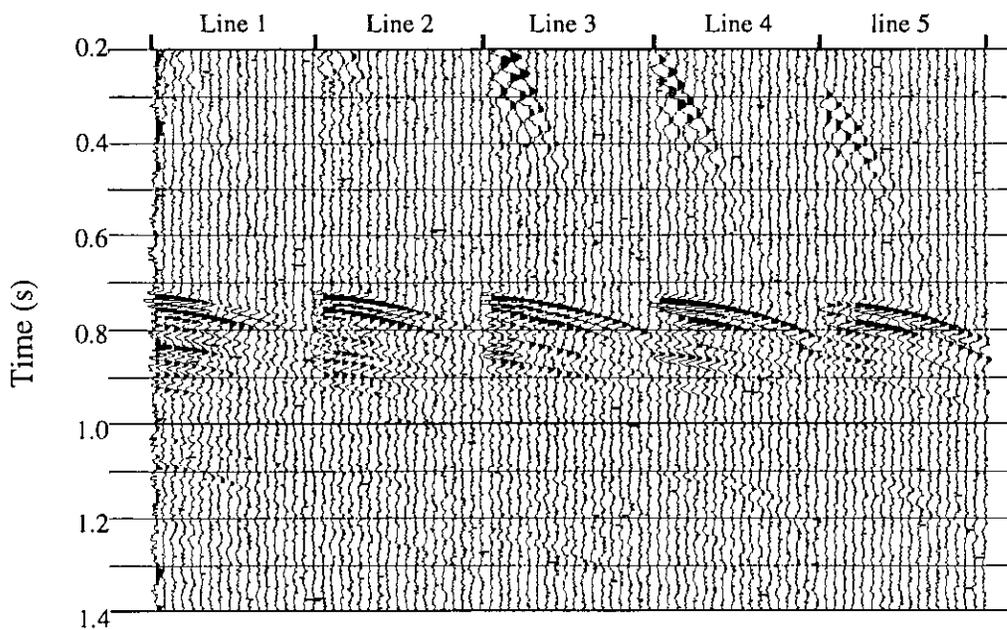
FIG. 8b. Example of transverse component  $P$ - $SV$  data. Shot was at station 1 on shot-line 1
