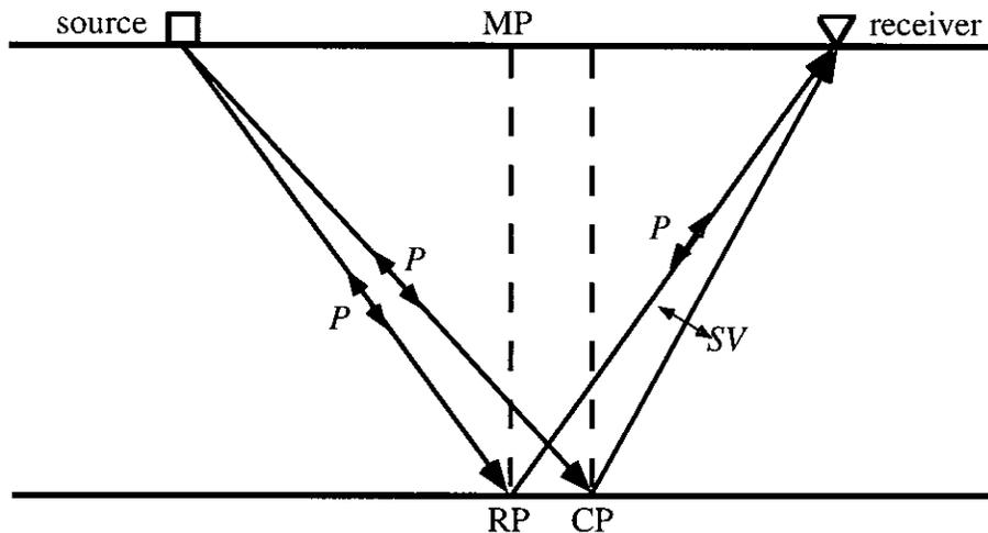
FIG. 1. Diagram of  $P$ - $P$  wave and  $P$ - $SV$  wave ray paths. RP:  $P$ - $P$  reflection point. CP:  $P$ - $SV$  conversion point.
