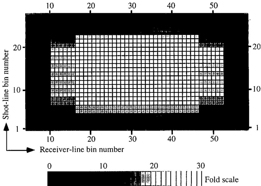
FIG. 11. Fold map of asymptotic common conversion point binning with optimum bin size 33.3 m
