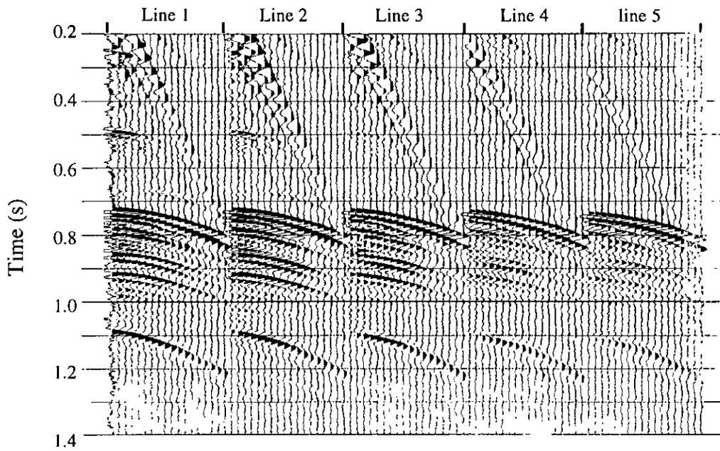
FIG. 7a. Example of in-line component *P-SV* data. Shot was at station 1 on shot-line 1.
