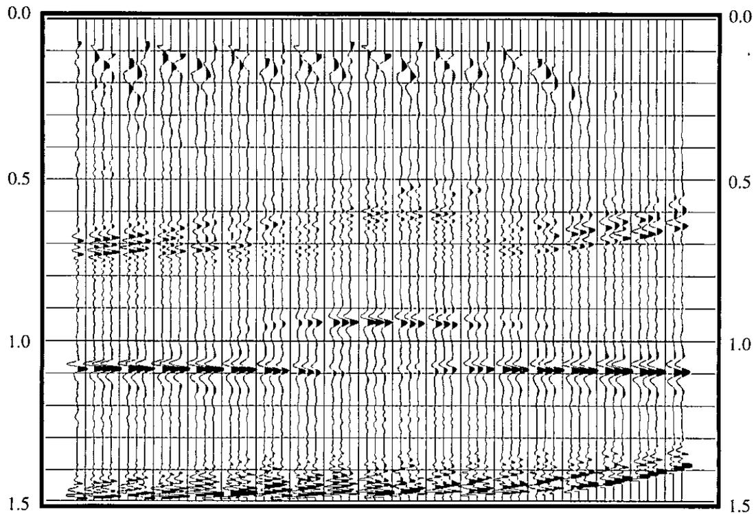
FIG. 14. Example section of  $P$ - $SV$  stacked data in receiver-line direction with bin size 25 m, without interpolation of the empty traces.
