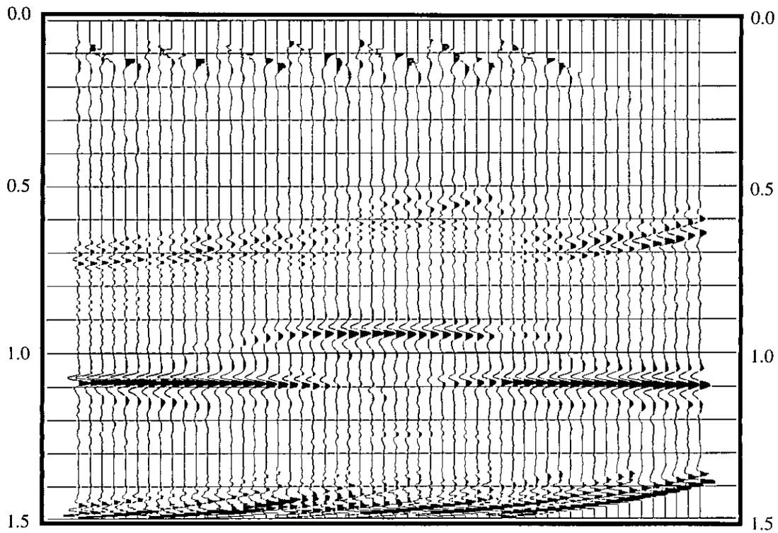
FIG. 16. Example section of *P-SV* stacked data in receiver-line direction with optimum bin size 33.3 m.
