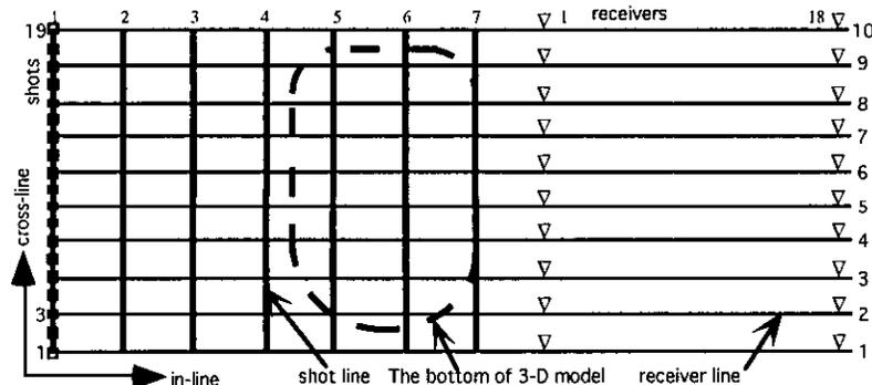
FIG. 3. Plan view of model showing acquisition geometry. Receiver locations are indicated for shot line 7.
