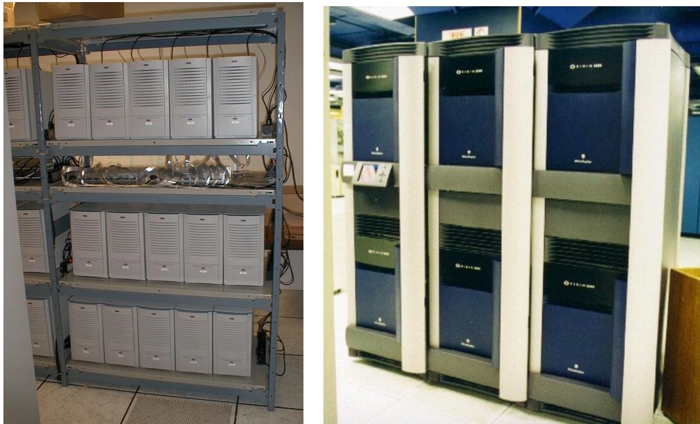
Figure 1. MACI systems: (left) A tightly networked cluster of 30 Compaq / DEC Alpha systems running at 500MHz installed at the University of Calgary. (right) A 42-processor SGI Origin 2000 installed at the University of Alberta.
