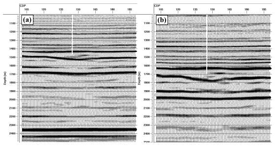
Figure 3: Migration images for Blackfoot vertical component data from (a) VTI v(z) f-k algorithm and (b) isotropic v(z) f-k algorithm. The white vertical lines indicate the well location.
