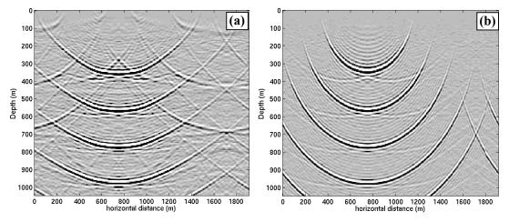
Figure 1: Migration impulse responses from v(z) f-k migration for VTI media, where (a) with non-zero anisotropic parameters and (b) with zero anisotropic parameters.
