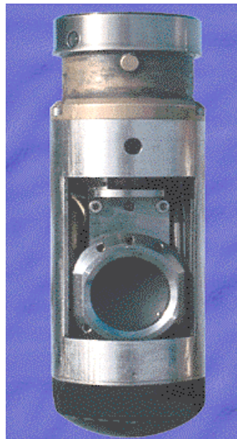
Figure 1. Schlumberger borehole imaging unit. The cylindrical ultrasonic transducer acts as a source and receiver. It rotates to provide complete circumferential coverage of the borehole wall (from www.slb.com ).
