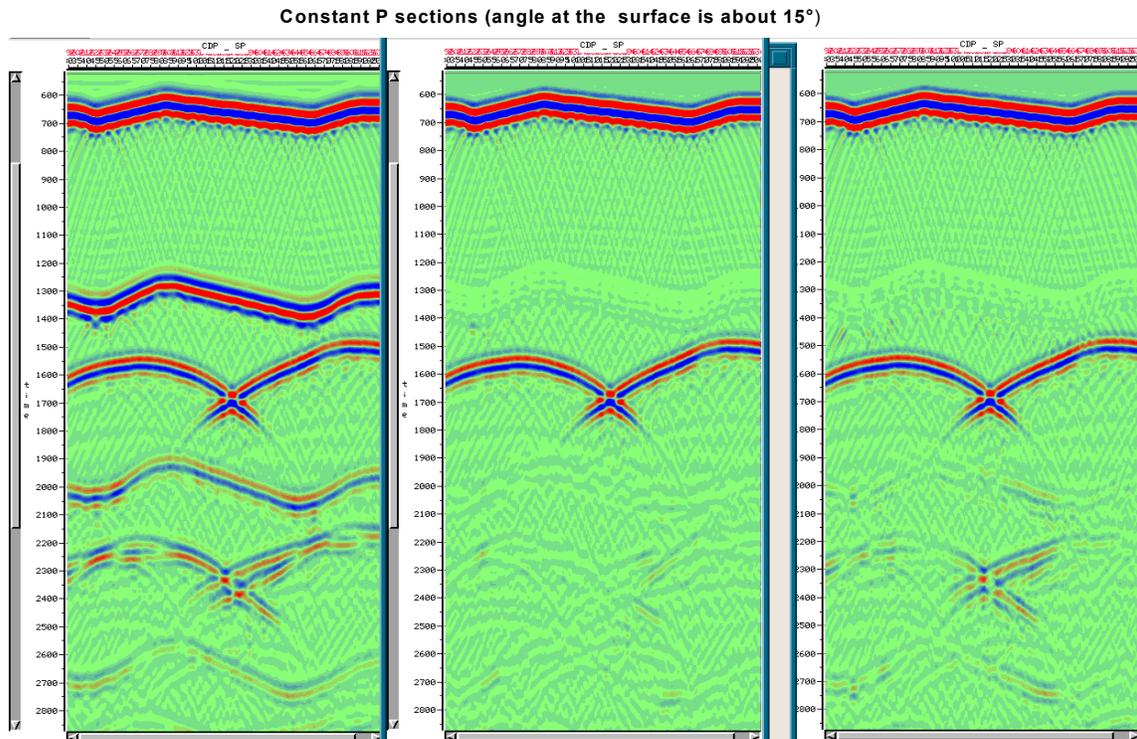
FIG. 2. Constant  $P$  –section before multiple suppression (left), after multiple suppression by the new wave-equation (WE) approach (centre) and after *Remul* (right).
