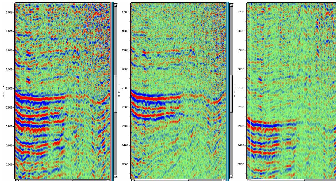
FIG. 4. Constant  $P$  sections for input data (left), after WE multiple suppression (centre) and the difference (right). The corresponding vertical angle of wave propagation at the surface is about  $8^\circ$ . Note how the weak dipping primaries are extracted from below strong multiples.
