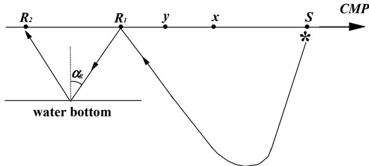
FIG. 1. Illustration of the stationary phase result:  $x$  and  $y$  are CMP positions of the primary and multiple events respectively. They are related by:  $x - y = 0.5(R_1 - R_2) = h \operatorname{tg} \alpha_g$ .
