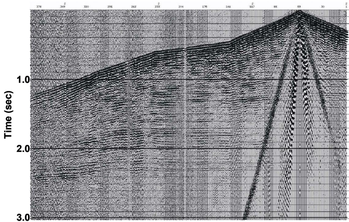
Figure 4. Raw shot gather, vertical component, after correlation and diversity stack (AGC applied).
