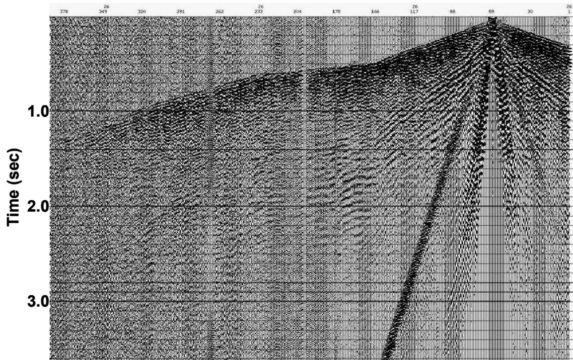
Figure 8. Raw shot gather, radial component, after correlation and diversity stack (AGC applied).
