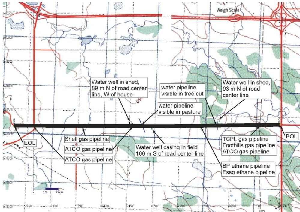
Figure 1. Multicomponent seismic line at Jumpingpound, Alberta. Line is 5 km long.
