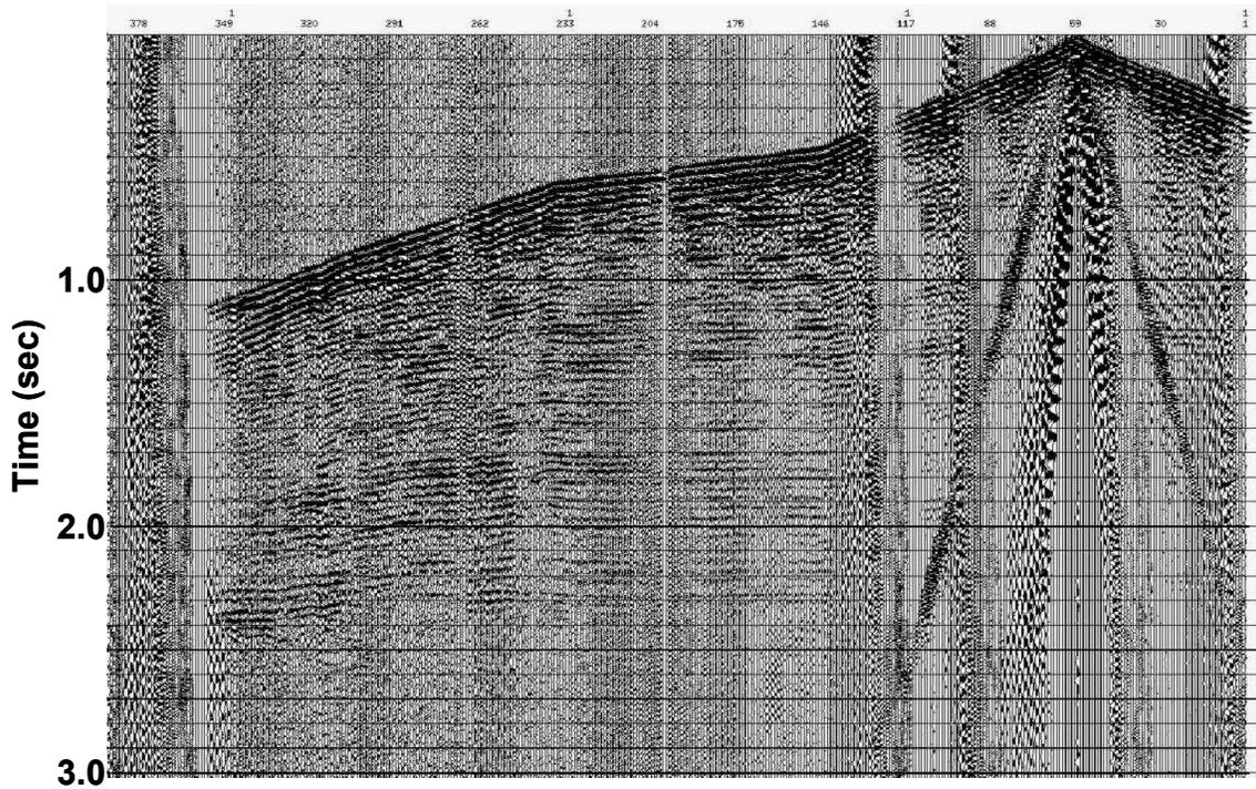
Figure 3. Raw shot gather, vertical component, after correlation and vertical stack (AGC applied).
