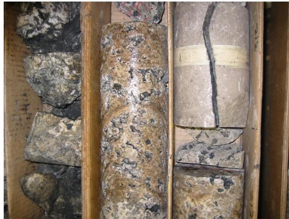
FIG. 4. Core from well 7-10. Porosity type seen here is zebroidal, mesovugs, and intercrystalline. Porosity averages 8%.
