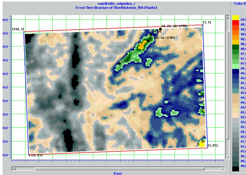
FIG. 4. PP time-thickness map from the 3C-3D seismic survey.
