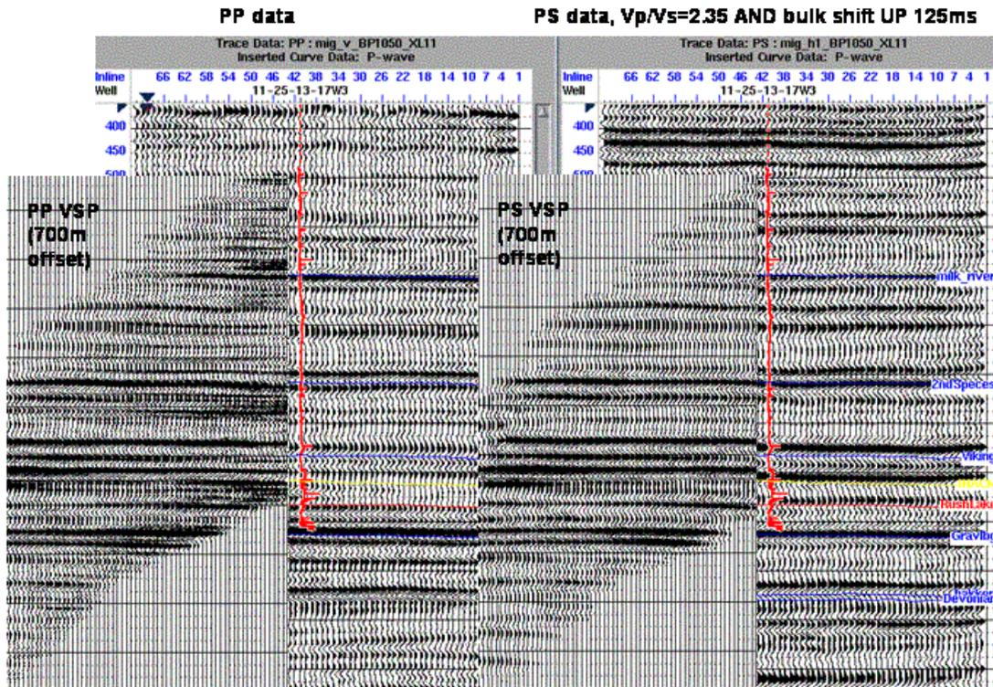
FIG. 5. The correlation between PP seismic, PS seismic, 700-m offset PP-VSP and 700-m offset PS-VSP, all plotted in PP time. Seismic data have a 5/10–50/60 Hz bandpass filter applied.
