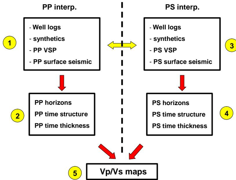
FIG. 3. Multicomponent seismic data interpretation workflow.
