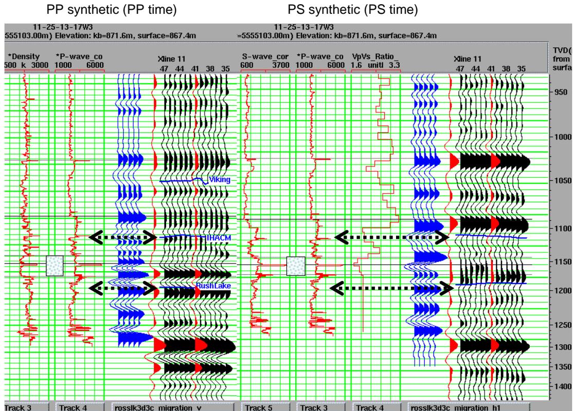
FIG. 2. Logs at well 11-25: PP synthetic and PP seismic; PS synthetic and PS seismic.
