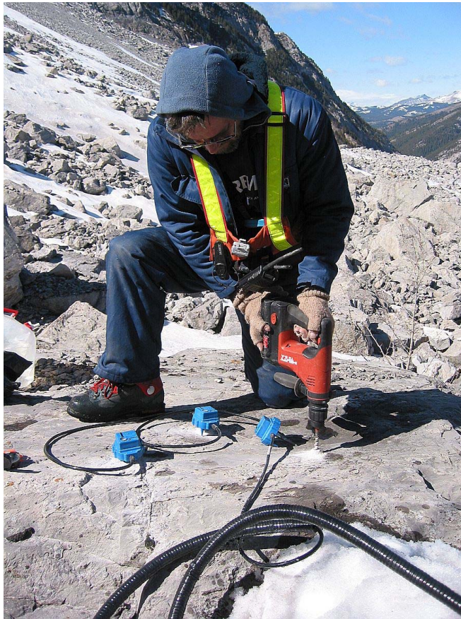
Figure 8. Three-component geophones are installed on Turtle Mountain (2003).
