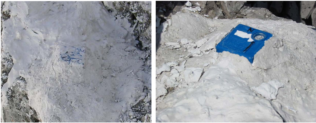
Figure 3. The northern-most geophone on South Peak is photographed on its installation date (left) and 5 months later (right). The plaster shows signs of deterioration.
