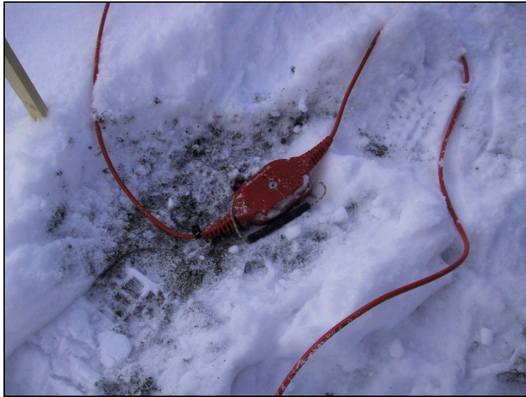
FIG. 4. Sercel DSU 3C unit after deployment
