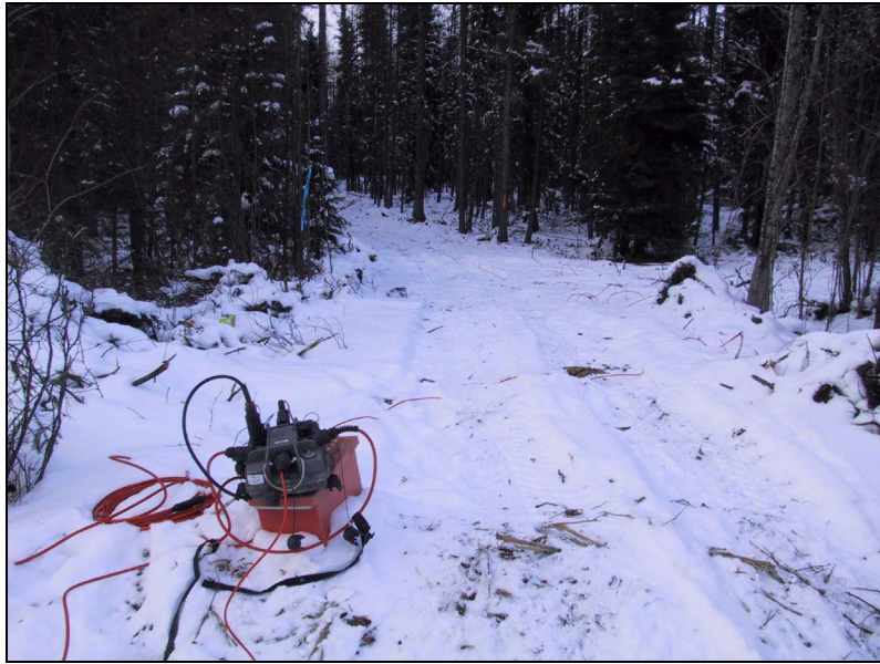
FIG. 2. Seismic recording equipment along Line 1.
