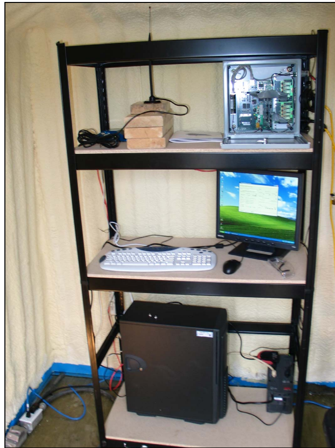
FIG. 18. The passive seismic recorder and associated equipment. The top shelf houses a cellular phone modem and antenna (now moved to an external mount) and the TAR unit. Two two yellow cables entering the TAR from the right are the signal cables coming from the sondes. The lower shelves house a PC system used to analyse and record the microseismic data.
