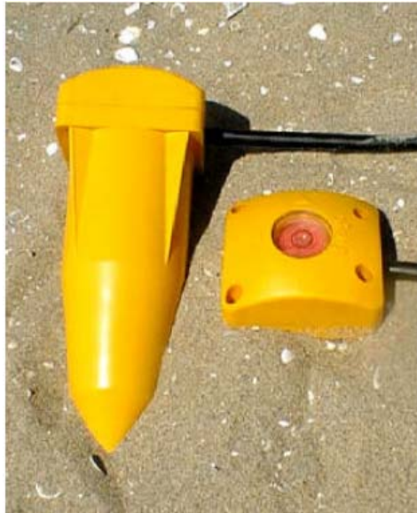
FIG. 1. Sensor SM24 Geophone elements in a PE-6/S case.
