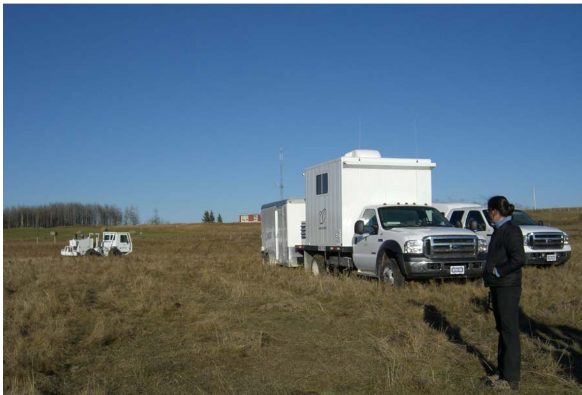
FIG. 2. Seismic equipment at the field site. The IVM Envirovibe (left) was used as the vibratory source. Data were recorded with the ARAM Aries-equipped recording truck (centre-right).
