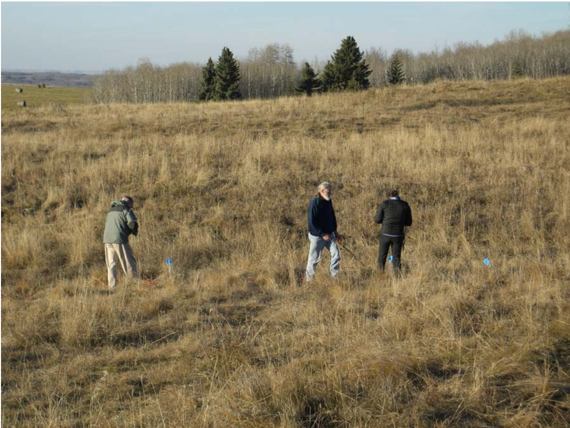
FIG. 4. The chaining crew marks out the site of the test patch. Geophones, planted using four variations of planting technique, are interspersed along three lines of geophones. The geophones are 2 m apart and the geophone lines are separated by 20 m.
