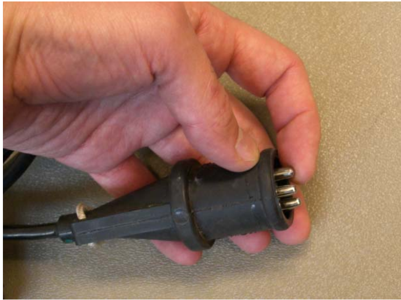
Figure 5. Oyo Geospace KCX-6F connector.
