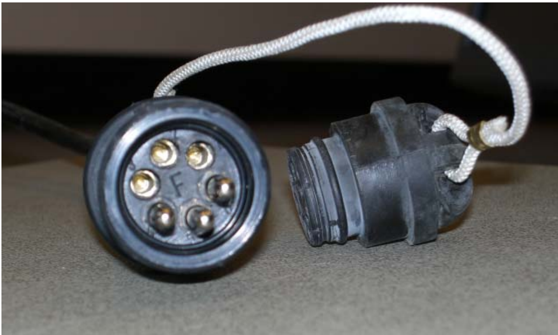
Figure 6. OYO Geospace KCX-6F connector and plug. The female connector (shown above) is connected to the geophone. The male connectors (KCX-6M) are located on the cable take-outs. Since both connectors have pins and sockets, the gender is determined by the rubber housing.
