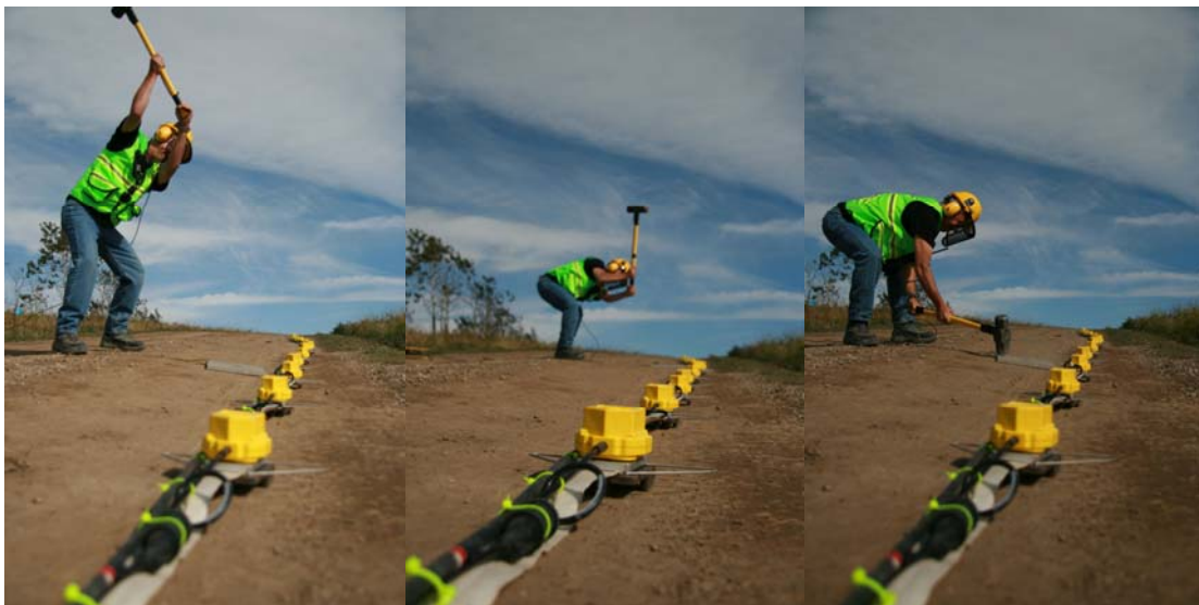
FIG. 5. Hammer seismic source used on the land streamer experiment.
