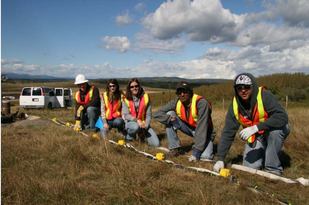
FIG. 4. Actual land streamer configuration used in the Priddis experiment .Individuals shown here with the University of Calgary’s Geophysics Field School.
