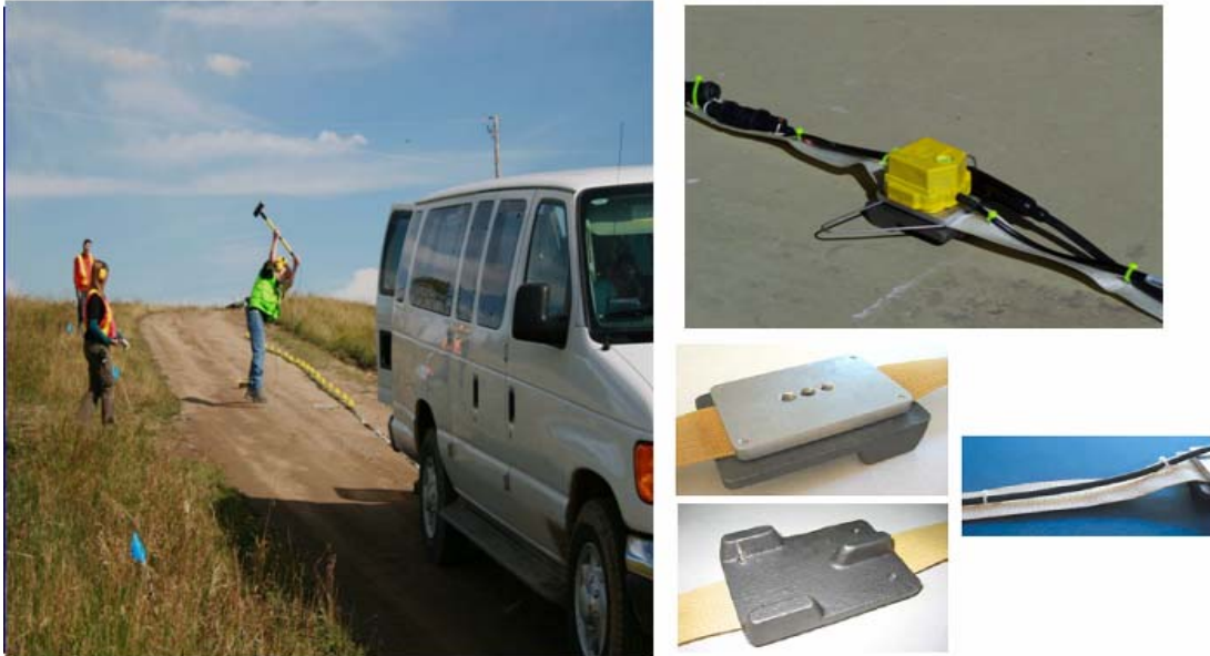
FIG. 2. Land streamer system components: land streamer basic configuration (left), geophone unit with wings to stop overturning (top right); top and bottom geophone plate and woven belt (bottom right).
