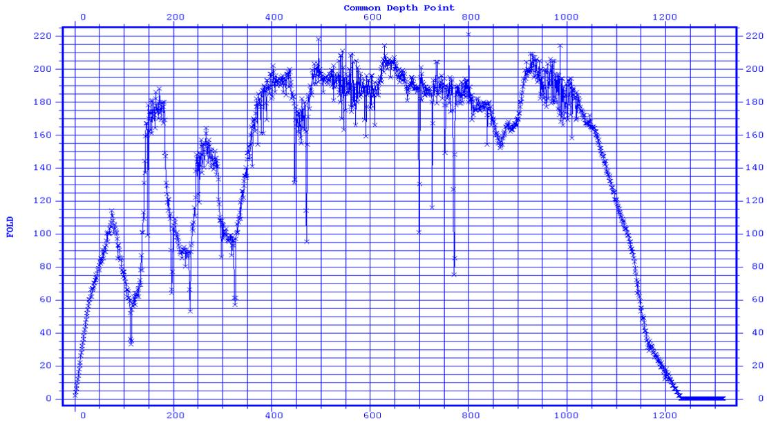
FIG. 5. CDP fold for 5x100 m bins; ARAM data.
