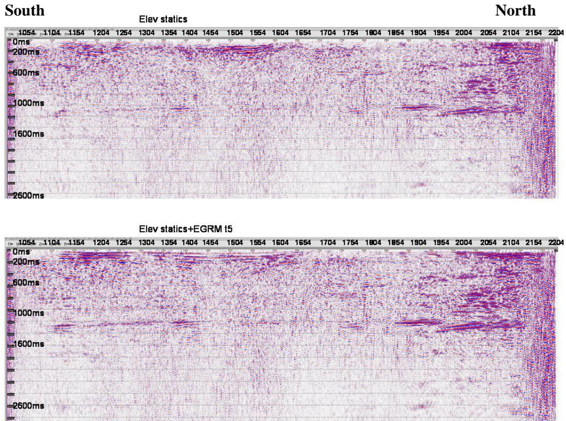
FIG. 3. Stacked section before and after refraction statics: Stack section with elevation statics (top), stacked section with elevation statics+final refraction statics (EGRM).
