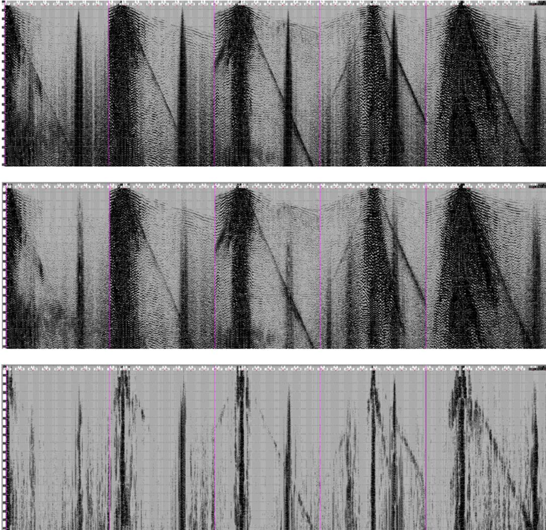
FIG. 2. First pass of signal enhancement using f-x filter: Raw shots (top), filtered shots (middle), difference between raw and filtered shots (bottom).
