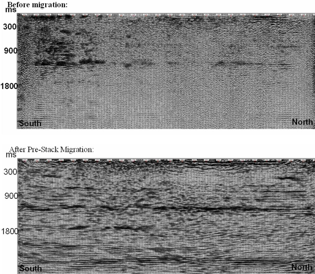
FIG. 5. Stack section before (top) and after (bottom) pre-stack migration.
