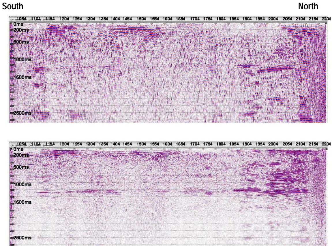
FIG. 4. Stack section before and after deconvolution : Stack section with 1<sup>st</sup> pass of noise rejection (top), stack section with 1<sup>st</sup> pass of noise rejection + surface consistent deconvolution.
