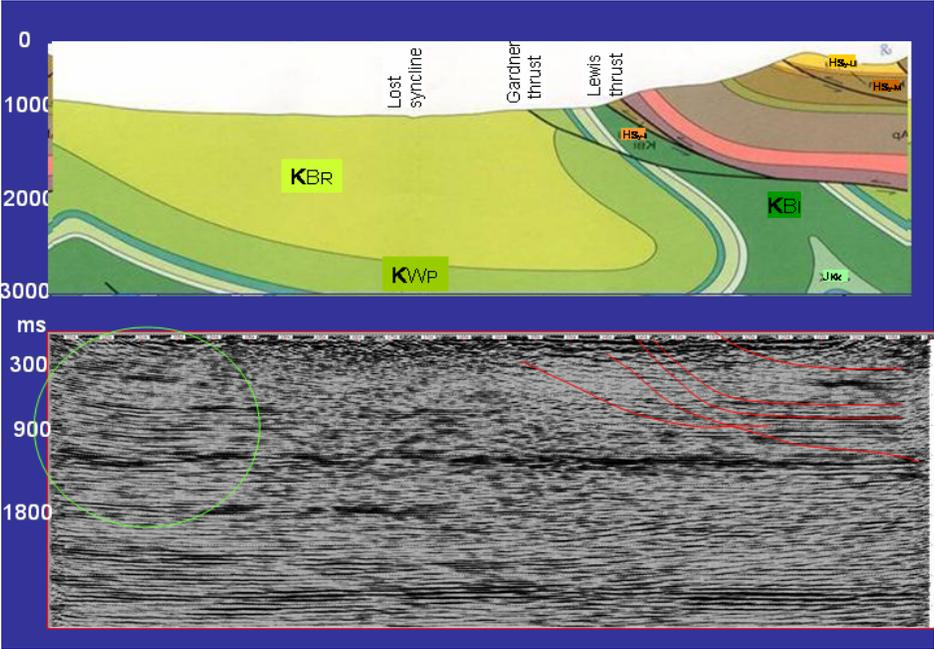
FIG. 6. Comparison of migrated image (bottom) with a geologic cross-section of the West Castle area (top) (modified from Norris, 1993).
