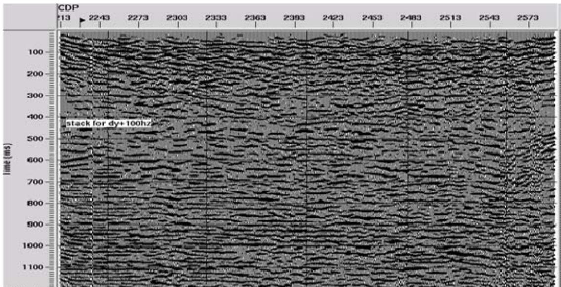
FIG. 30. CDP stack of 100 Hz pump-probe survey. Compare this with Figure 27 for any significant differences.
