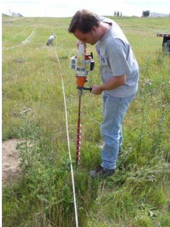
FIG. 4. Preparing the receiver line
