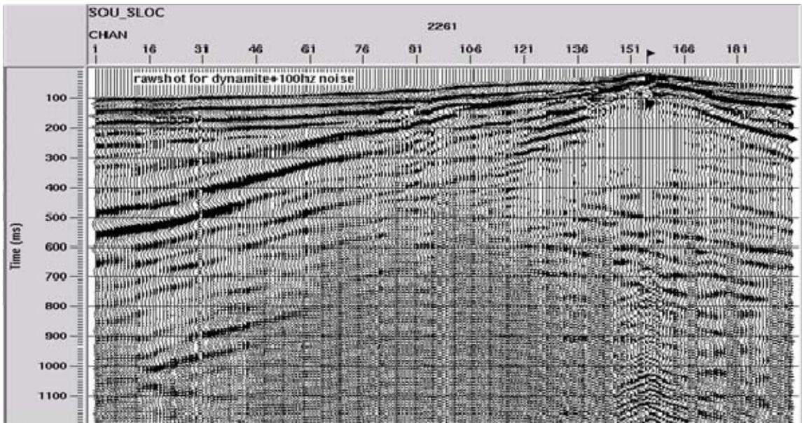
Raw shot from dynamite plus 100 Hz vibroseis
