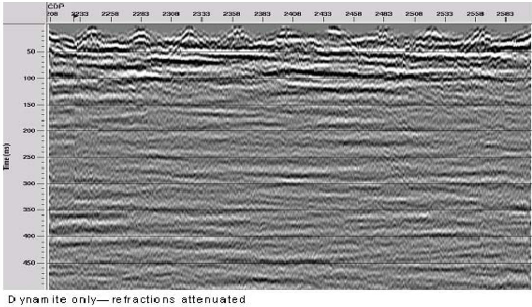
FIG. 56. CDP stack for 'dynamite only' survey after attenuation of near-surface refraction events.
