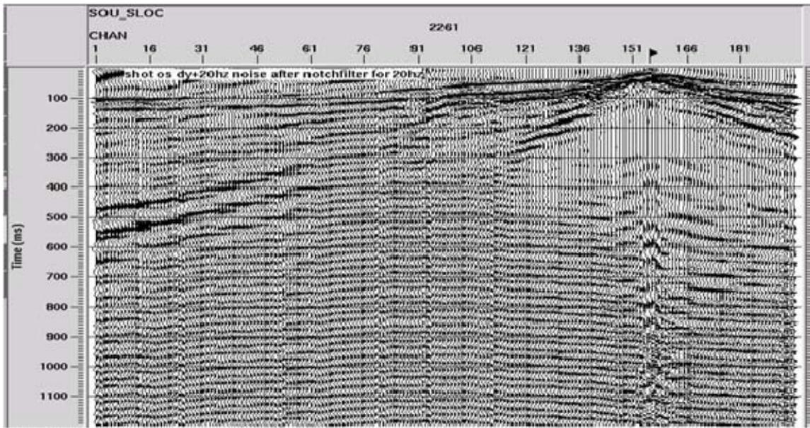
Shot from dynamite plus 20 Hz vibroseis after 20 Hz notch filter
