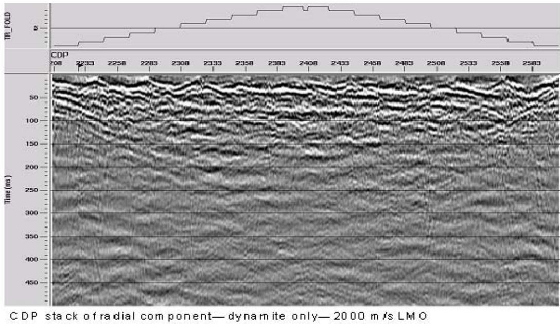
FIG. 54. CDP stack of radial component of 'dynamite only' survey with 2000 m/s LMO applied to shot gathers.
