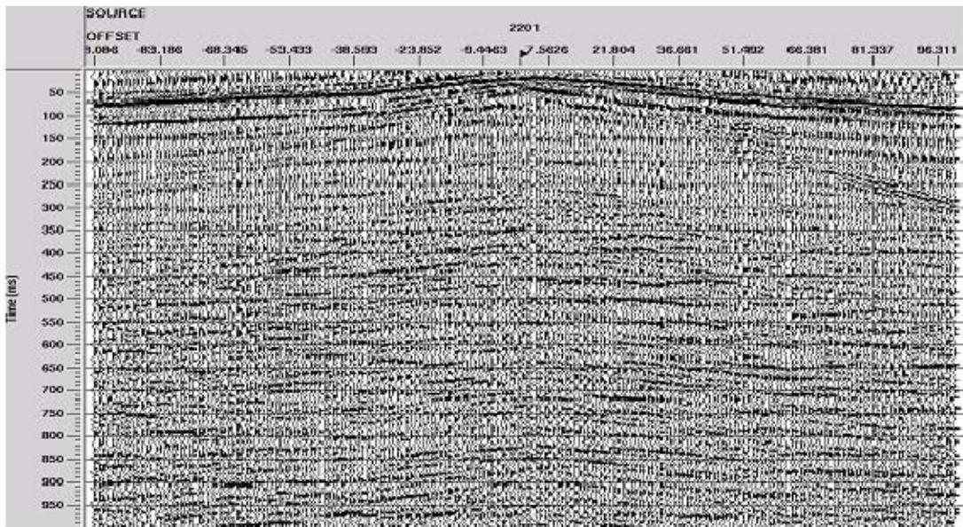
Typical shot gather—vibroseis only—after filtering and deconvolution
