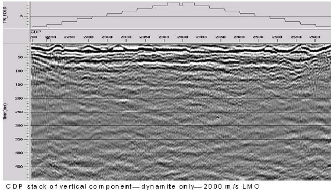
FIG. 50. CDP stack of 'dynamite only' survey with 2000 m/s LMO applied to shot gathers.
