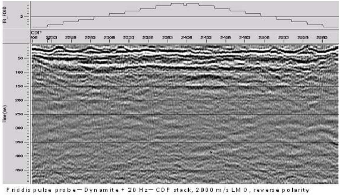
FIG. 51. CDP stack of 20 Hz pump-probe survey with 2000 m/s LMO applied to shot gathers.
