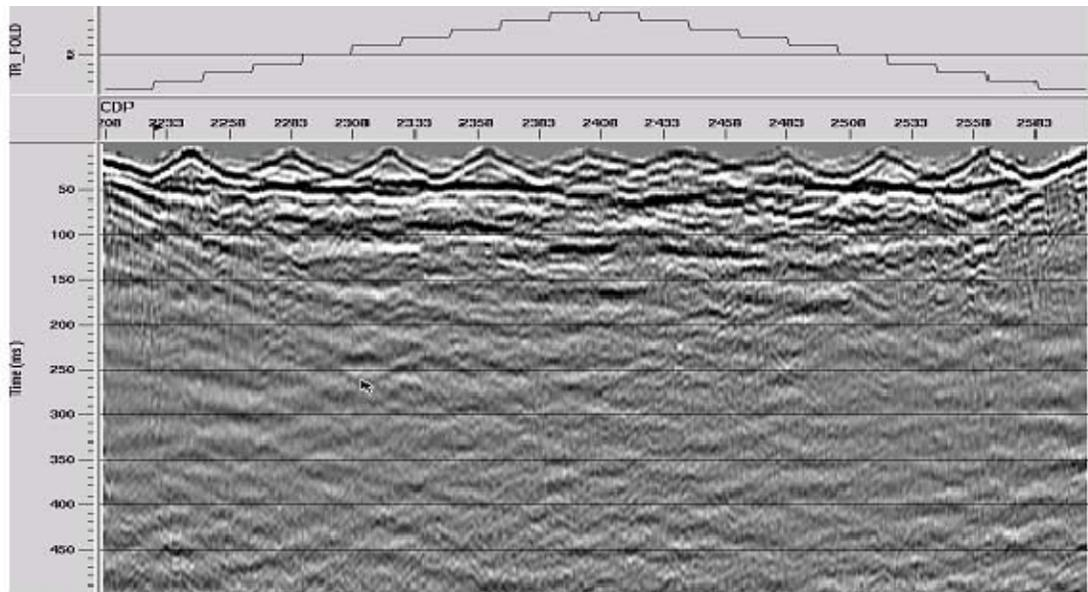
FIG. 45. CDP stack of 'dynamite only' survey with 2000 m/s NMO applied to shot gathers.
