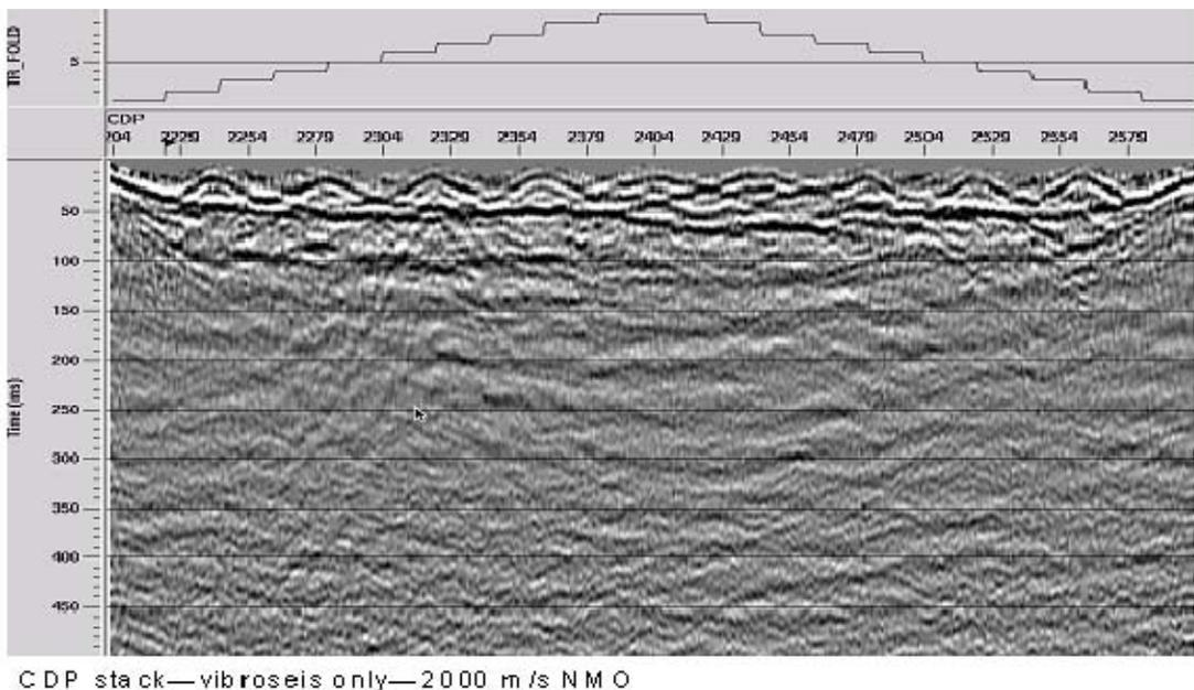
FIG. 44. CDP stack of ‘Vibroseis only’ survey with 2000 m/s NMO applied to shot gathers.
