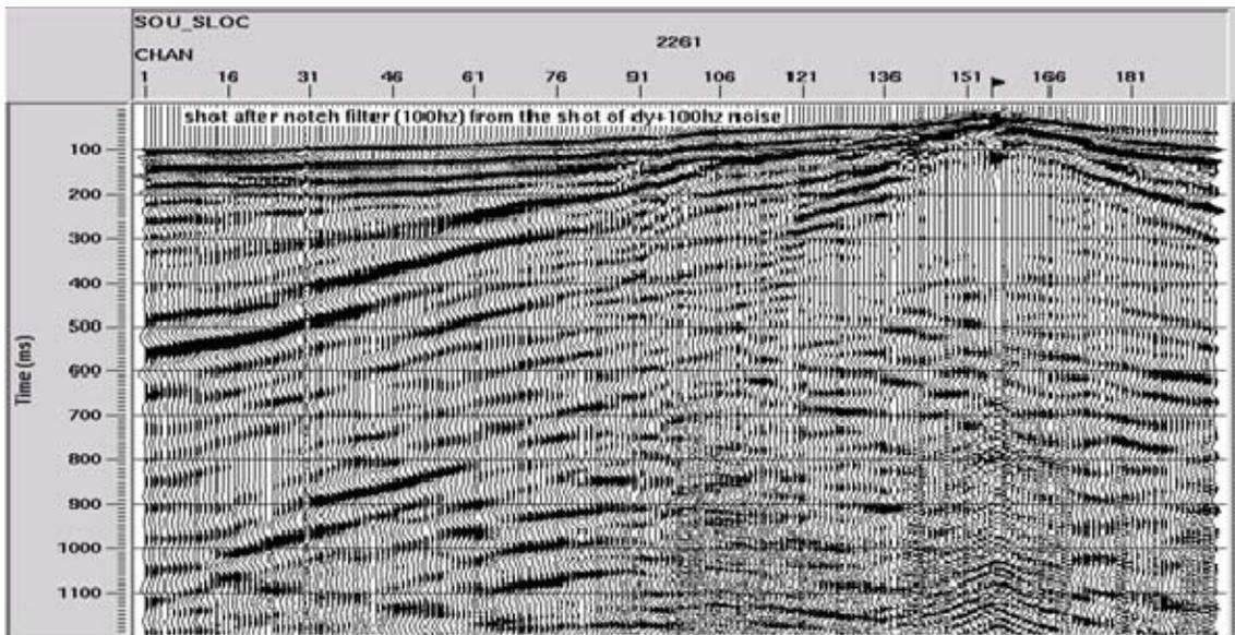
Shot for dynamite plus 100 Hz vibroseis after 100 Hz notch filter
