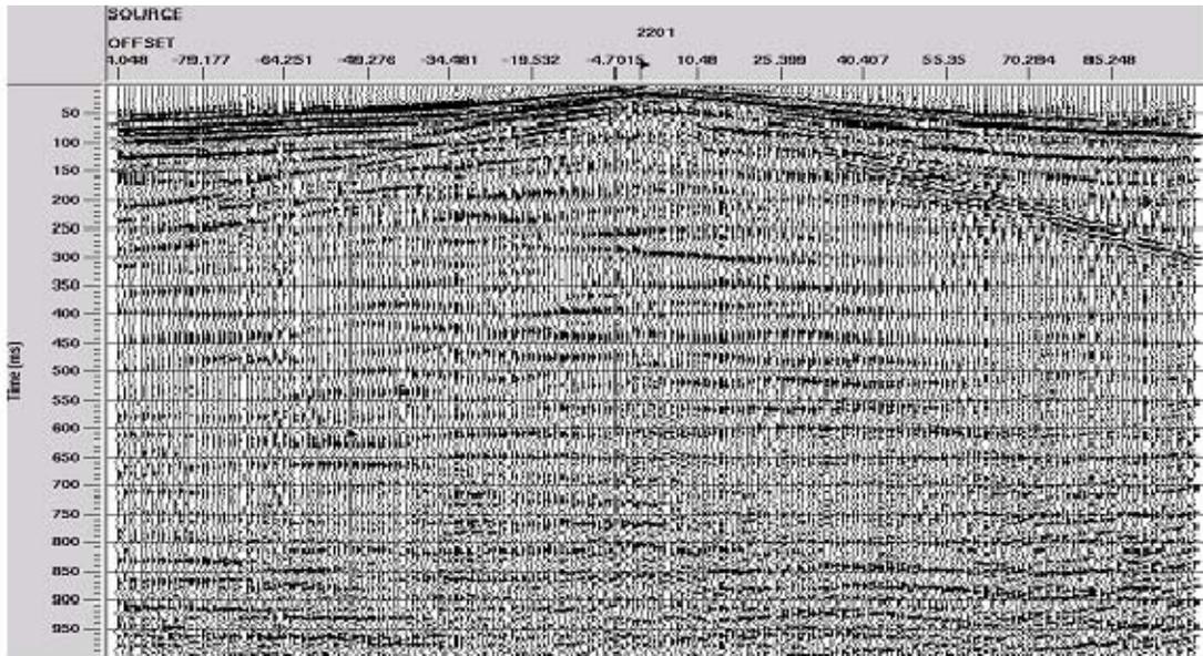
Typical shot gather for 'dynamite only' after filtering and deconvolution
