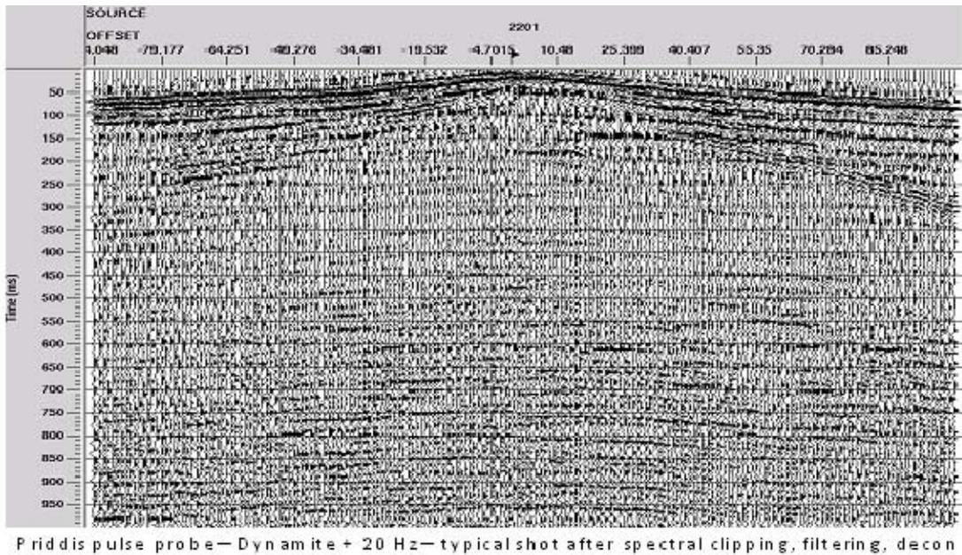
FIG. 37. Shot gather of Figure 36 after radial trace filtering and Gabor deconvolution.
