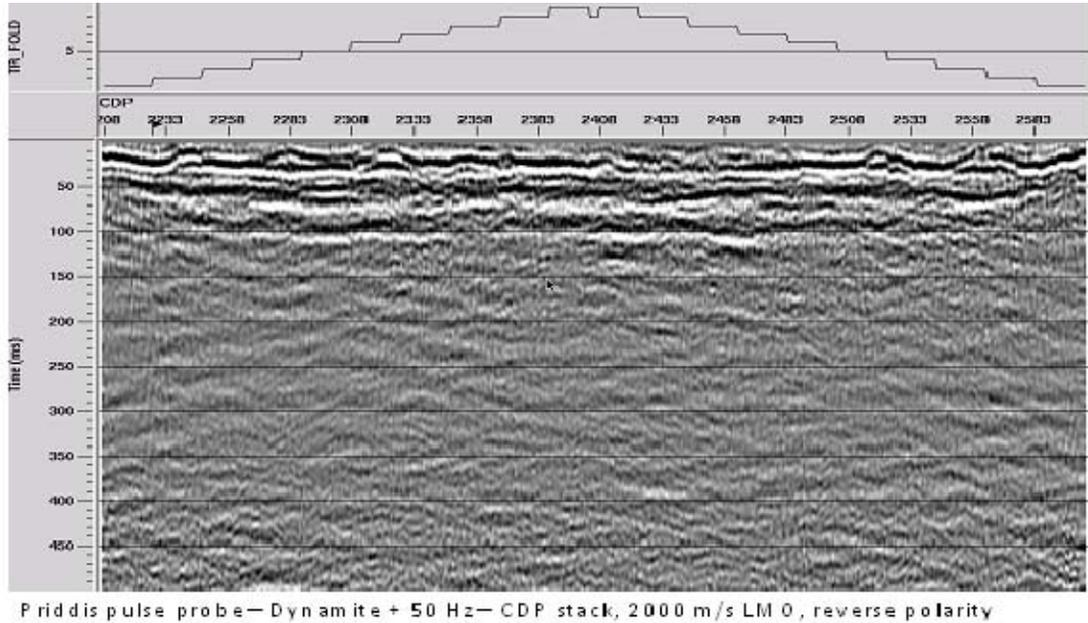
FIG. 52. CDP stack of 50 Hz pump-probe survey with 2000 m/s LMO applied to shot gathers.
