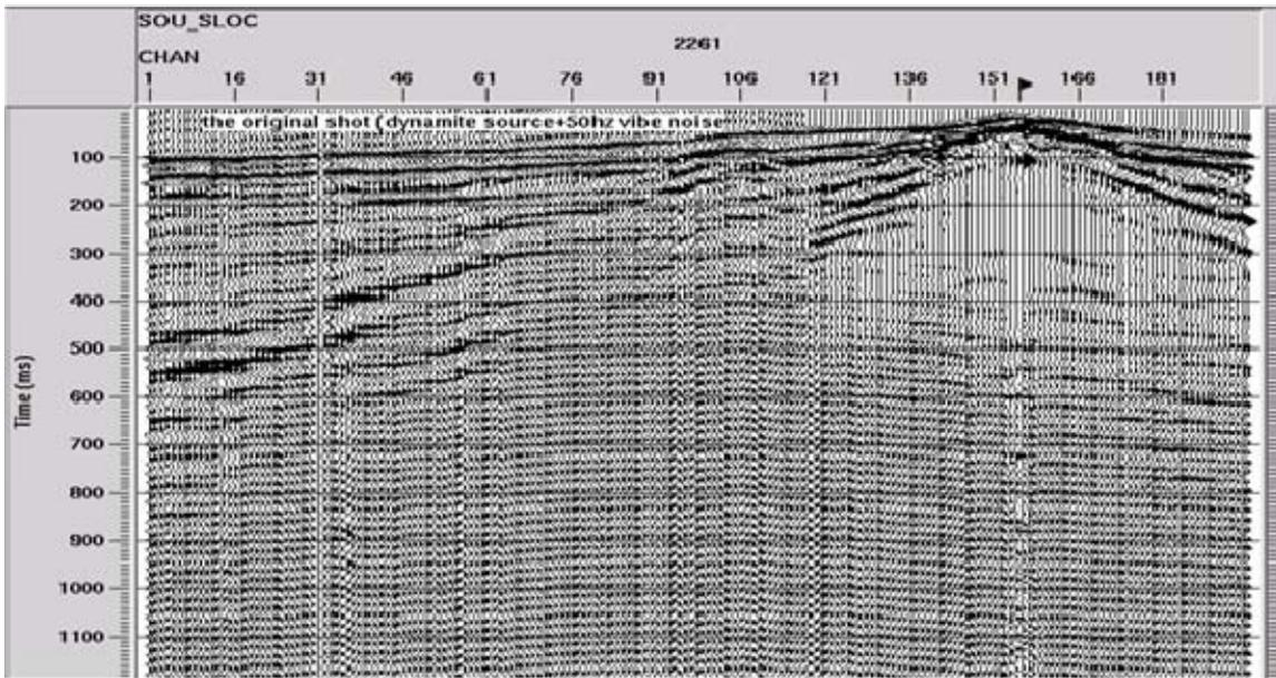
Raw shot from dynamite plus 50 Hz vibroseis
