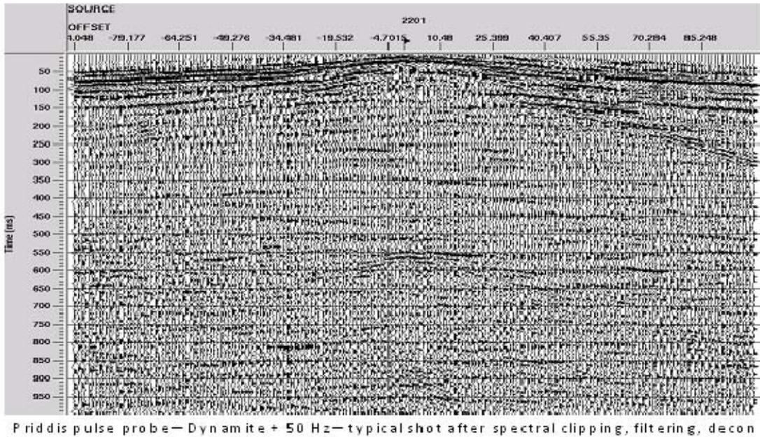
FIG. 40. Shot gather of Figure 39 after radial trace filtering and Gabor deconvolution.
