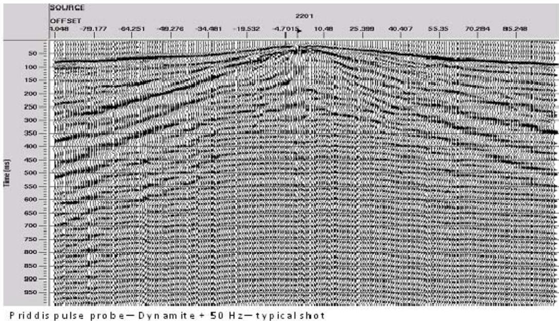
FIG. 38. Typical shot gather for 50 Hz pump-probe survey. 50 Hz Vibroseis signal dominates record.
