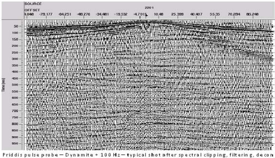
FIG. 43. Shot gather from Figure 42 after radial trace filtering and Gabor deconvolution.
