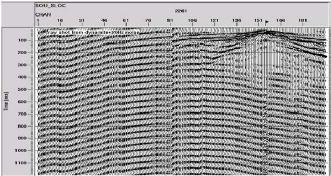
Raw shot from dynamite plus 20 Hz vibroseis
