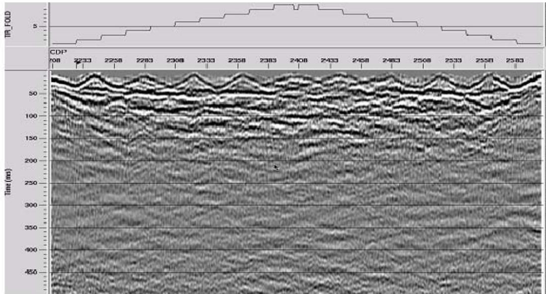
FIG. 46. CDP stack of 20 Hz pump-probe survey with 2000 m/s NMO applied to shot gathers.
