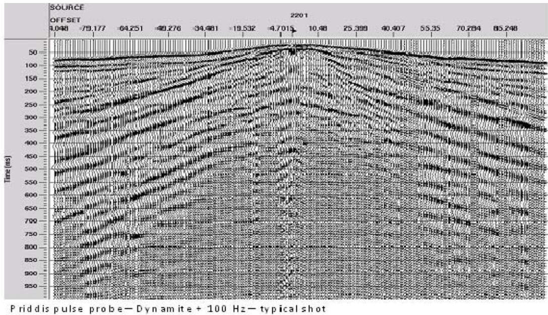
FIG. 41. Typical shot gather from 100 Hz pump-probe survey. 100 Hz Vibroseis signal is strong, but not dominant.
