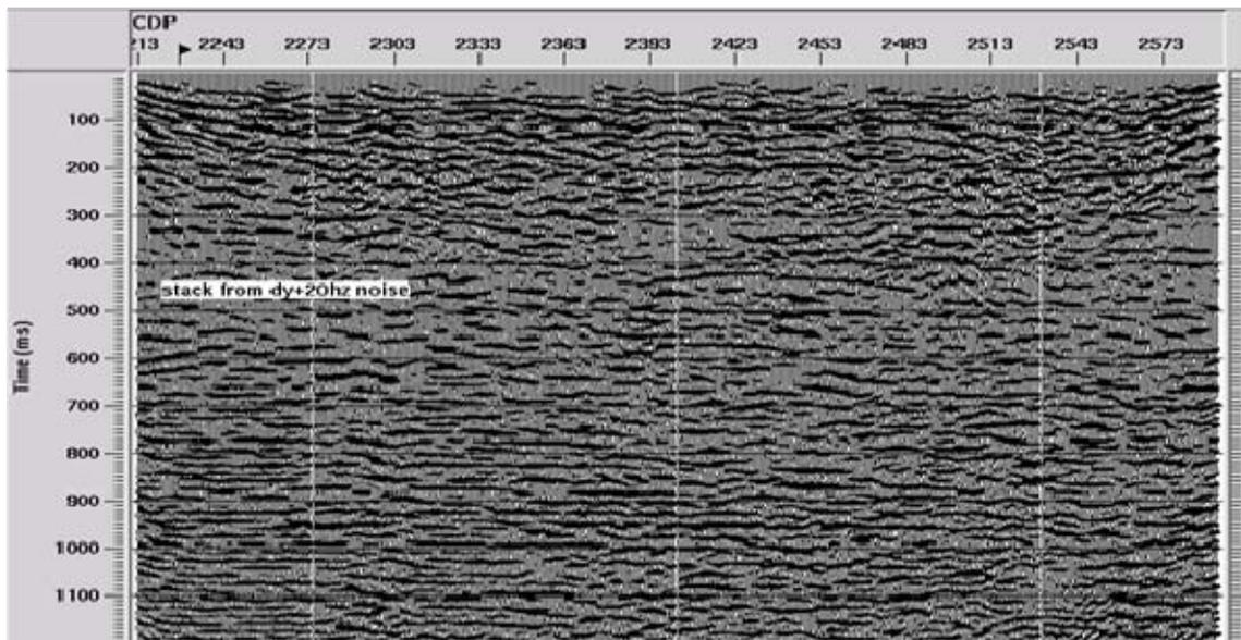
Stack of gathers for dynamite plus 20 Hz vibroseis
