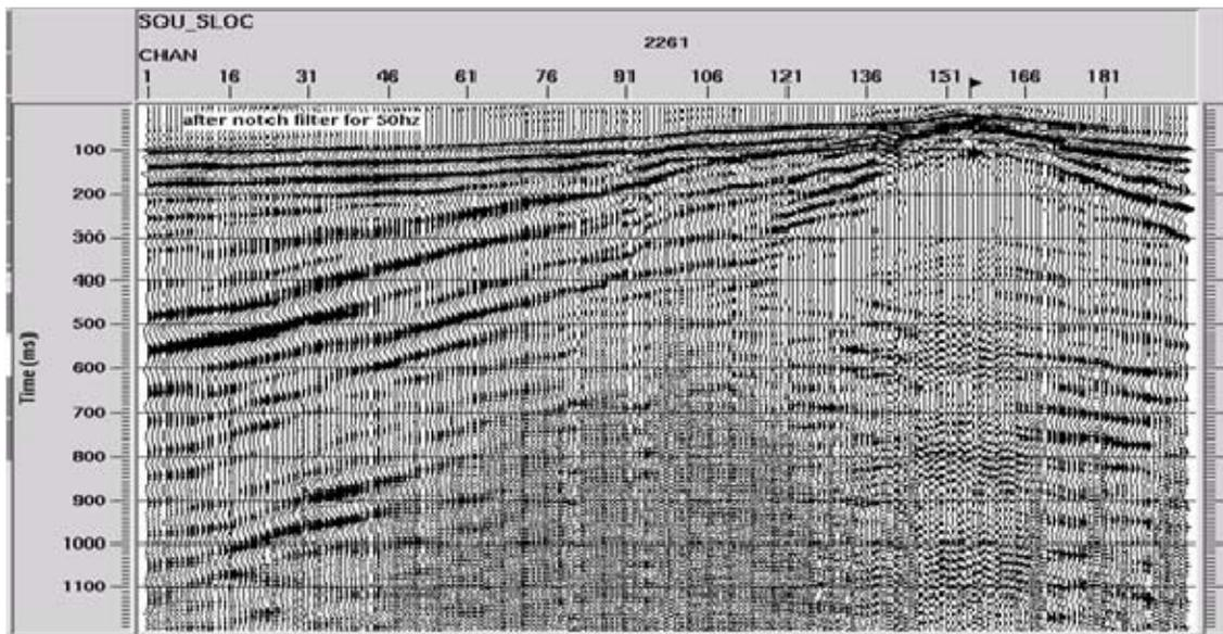
Shot for dynamite plus 50 Hz vibroseis after 50 Hz notch filter
