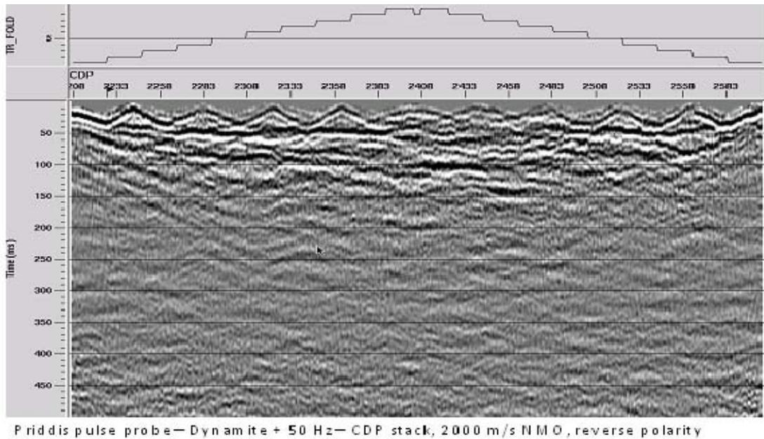
FIG. 47. CDP stack of 50 Hz pump-probe survey with 2000 m/s NMO applied to shot gathers.
