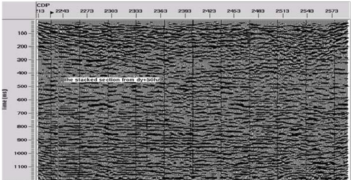
FIG. 29. CDP stack of 50 Hz pump-probe survey. Compare this with Figure 27 for any significant differences.
