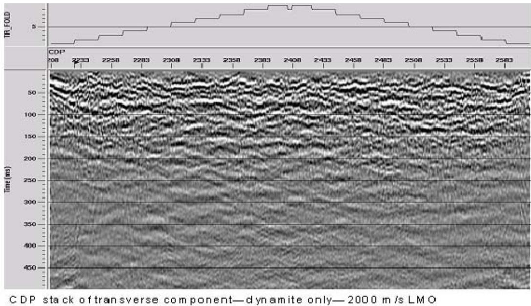
FIG. 55. CDP stack of transverse component of 'dynamite only' survey with 2000 m/s LMO applied to shot gathers.
