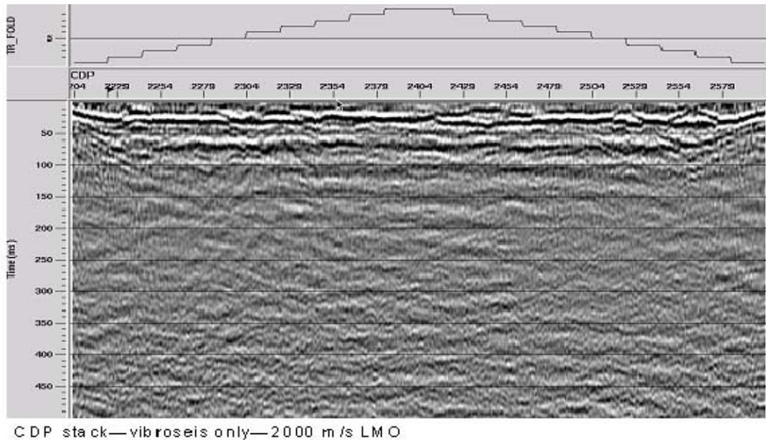
FIG. 49. CDP stack of 'vibroseis only' survey with 2000 m/s LMO applied to shot gathers.
