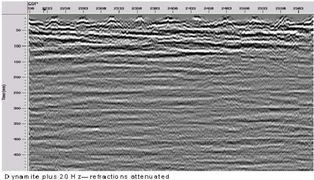
FIG. 57. CDP stack for 'dynamite plus 20 Hz' pump-probe survey after attenuation of near-surface refraction events.
