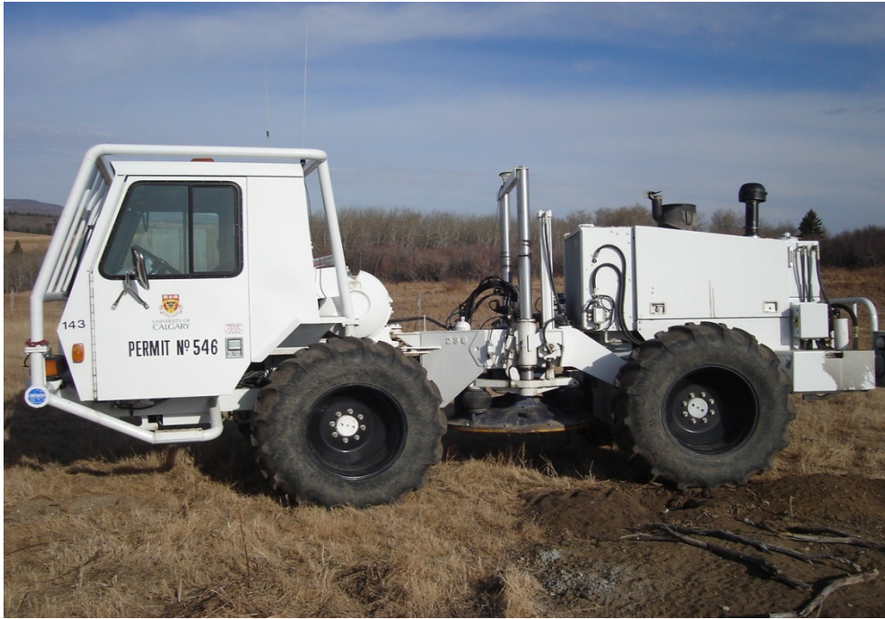
FIG. 1. The EnviroVibe vibrator source used in the VSP survey.
