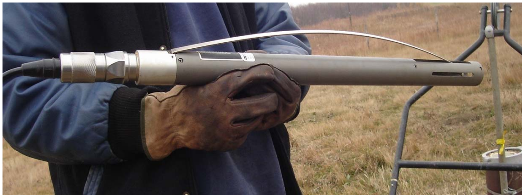
FIG. 2. The downhole 3C geophone with motor-driven, bow-spring used clamp.
