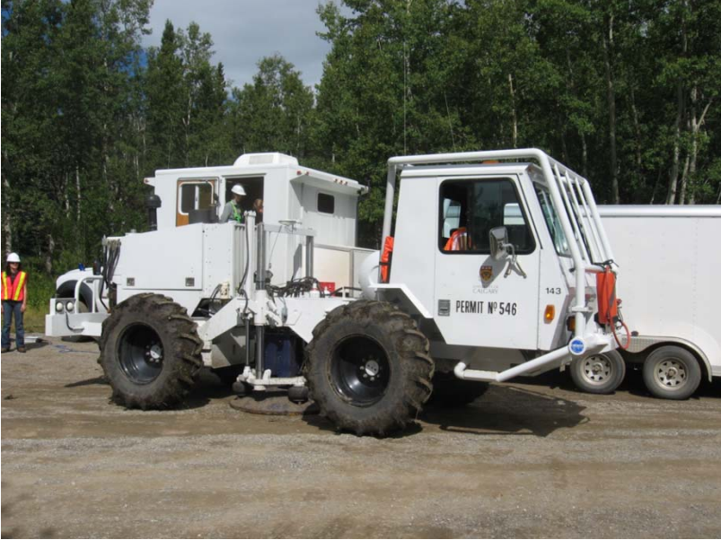
FIG. 3. Envirovibe seismic source used for the 3D survey.
