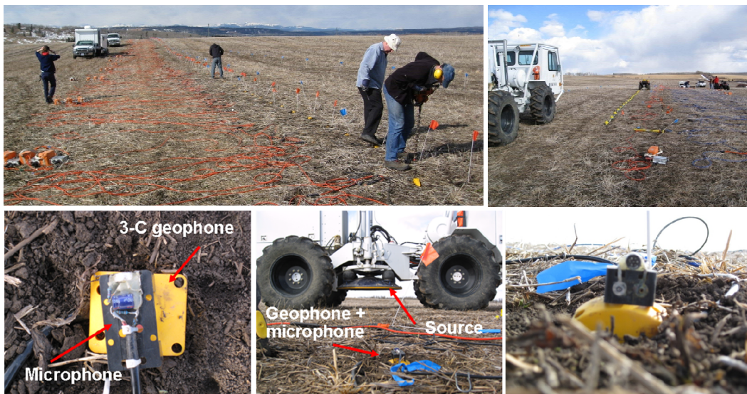
FIG. 4. CREWES students and staff provided a valuable help in the field. A small 15 cm deep by 6 cm wide hole was drilled for each geophone using a gas-powered handheld auger. Each microphone was placed beside a geophone every 5 m. An IVI EnviroVibe was used as the seismic source at 5 m spacing within the spread and 10 m for long offsets (Photos by Gabriela Suarez and first author).
