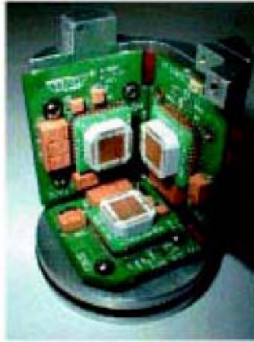
FIG 2. Cutaway of the three MEMS accelerometers mounted within a VectorSeis frame (Maxwell, 2001).
