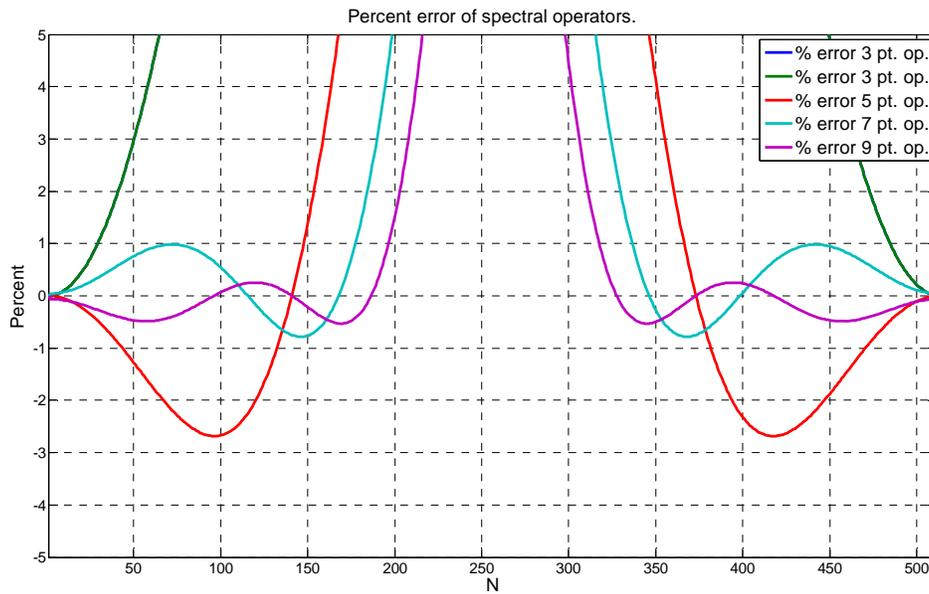
FIG. 10. Percent errors for the time domain windowing operators.
