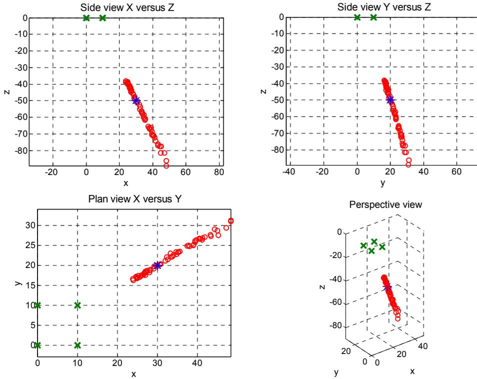
FIG. 1 Plot of source sensitivity when the x and y coordinates of the receivers are perturbed by 1% or a SD = 0.1 m.
