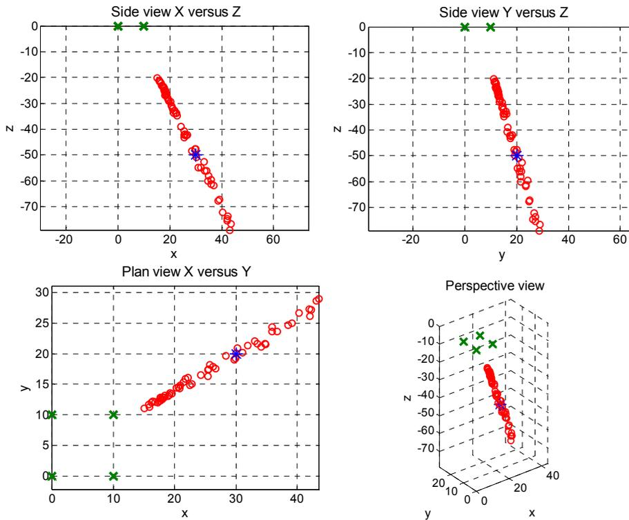
FIG. 2 Plot of source sensitivity when the z coordinate of the receivers is perturbed by 1% or a SD = 0.1 m.
