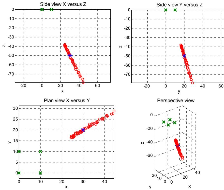
FIG. 3 Plot of source sensitivity when the traveltime from the source to the receivers is perturbed with a jitter that has a SD = 0.025 ms.
