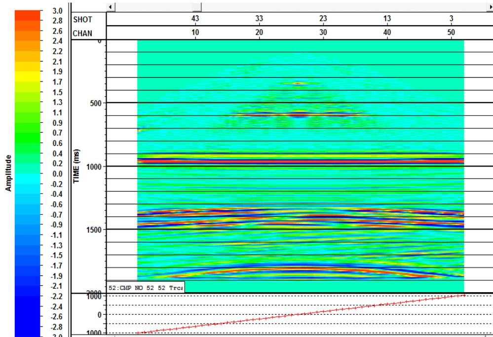
FIG 15. This figure shows a common midpoint gather for 510m and has been normal move out corrected. The area of interest is from 0.9 seconds to 1.0 seconds as this is the channel interval.
