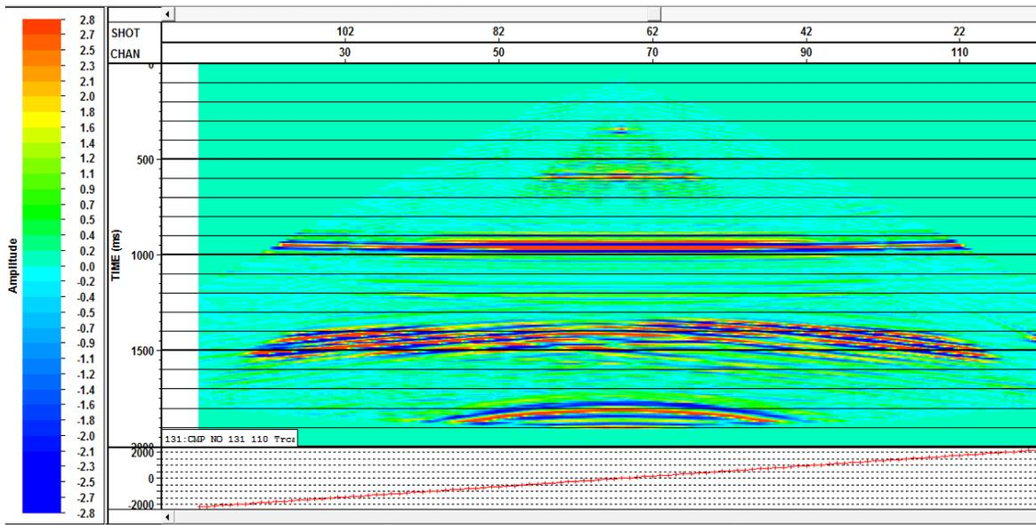
FIG 17. This figure shows a common midpoint gather for 1300m and has been normal move out corrected. The Trough that was picked for the amplitude variation with offset study is at about 0.9 seconds.
