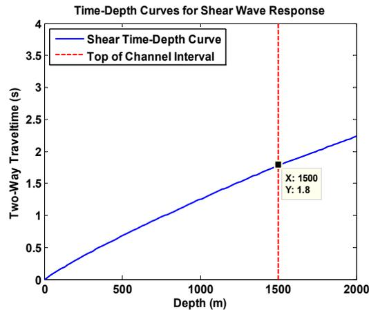
FIG 7c. This figure shows the time-depth curve for the shear waves. The first reflection of the shear wave off the top of the channel interval would arrive at about 1.8 seconds.
