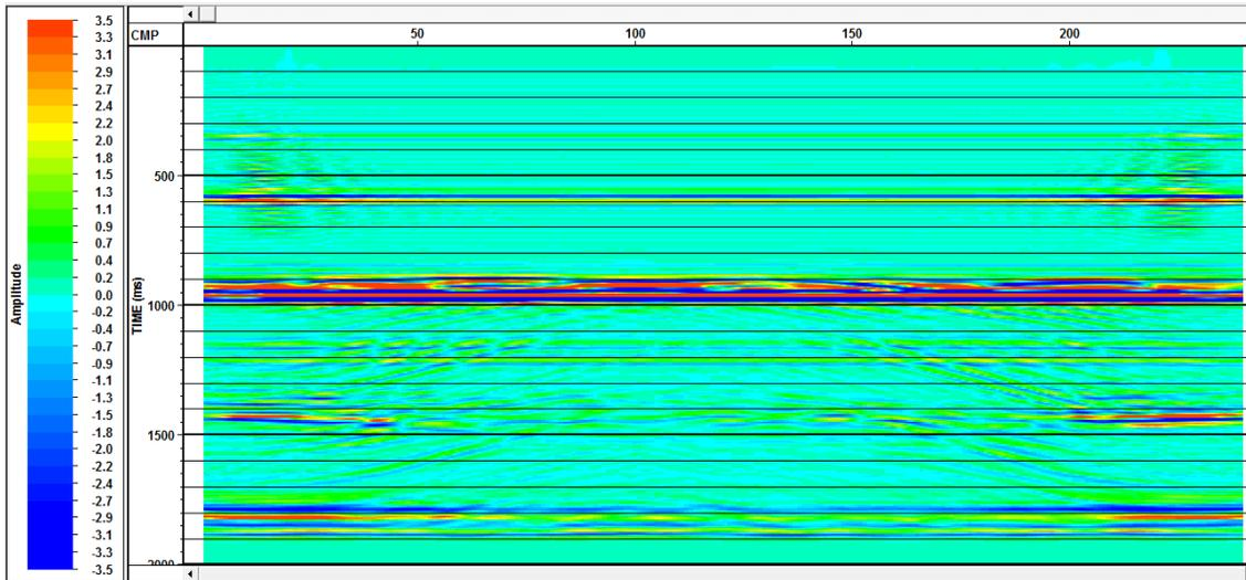
FIG 14. This figure shows a post-stack Kirchhoff migration. The channel interval is at about 0.9 seconds and shows undulations that can be attributed to the varying channel sands.
