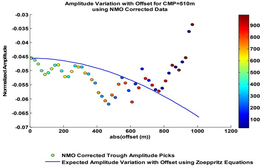
FIG 16. This figure shows the amplitude variation with offset for a common midpoint gather at 520m using normal move out corrected data. The impedance contrast at the 520m gather was negative resulting in a trough being picked. This point in the model also had a low  $V_p/V_s$  ratio. The blue line is the theoretical, expected result where as the coloured dots are measured. The color of the dots indicates the y-coordinate of the geophone that recorded the data.
