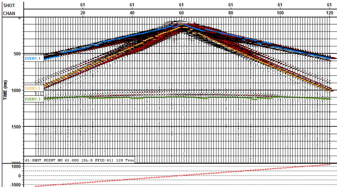
FIG 10. This figure shows the raw shot 61. Event 1 is the first breaks, indicated by blue. Event 2 is ground roll and is indicated with orange.
