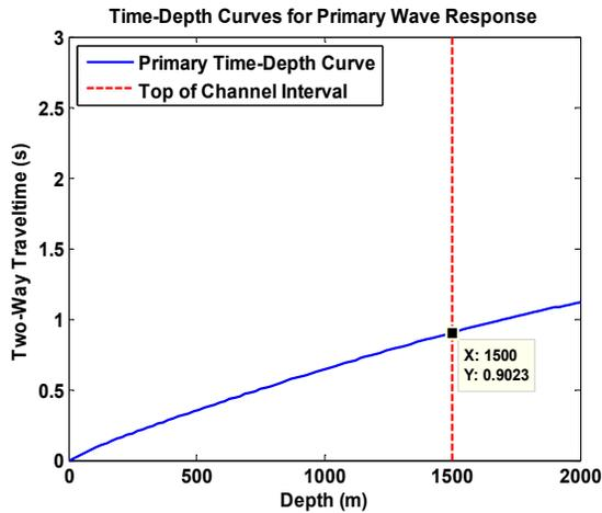
FIG 7a. This figure shows the time-depth curve for the primary waves. Using this it should take about 0.9023 seconds to the top of the channel (indicated by the intersection of the blue and red lines).
