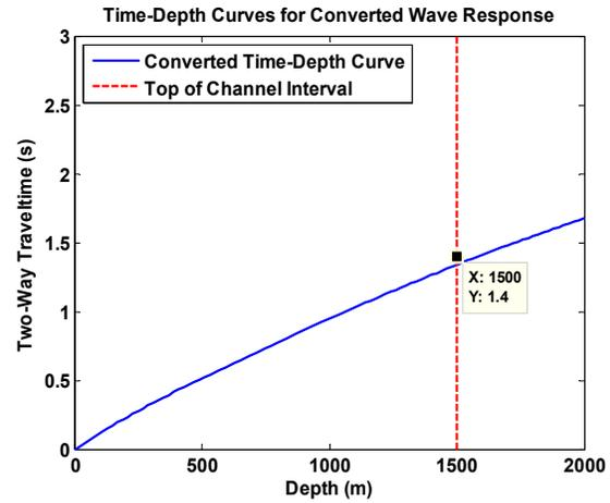
FIG 7b. The converted wave time-depth curve is represented in this figure. The first converted wave reflection of the top of the channel should arrive at about 1.4 seconds.
