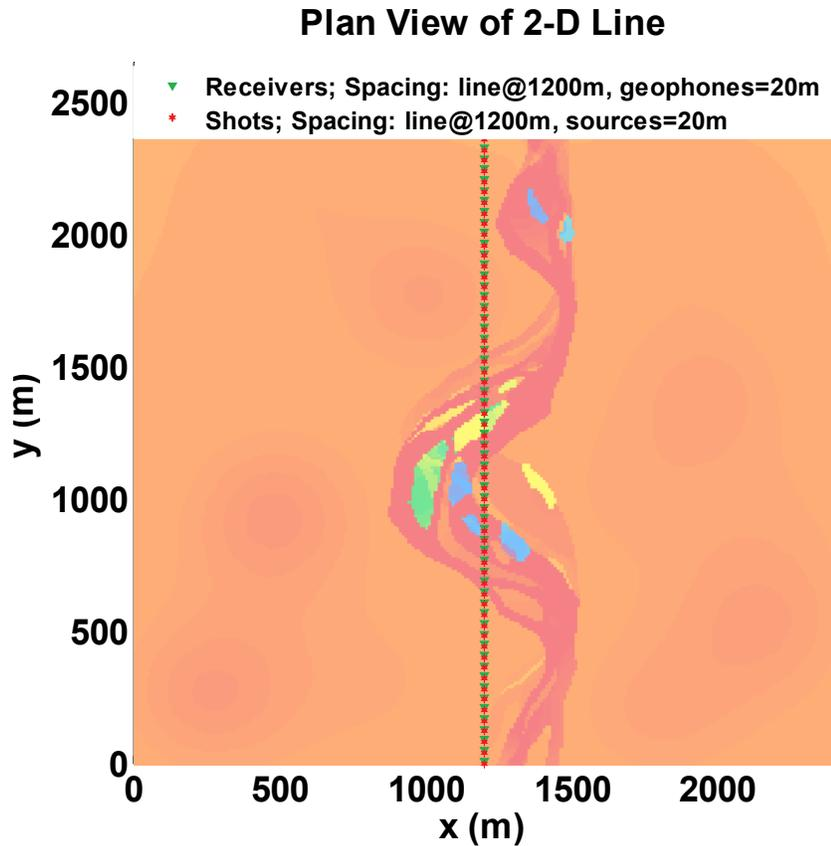
FIG 8. This figure shows the location of the 2-D line with respect to the channel. The receivers and shots are spaced every 20m, with the shots starting at 0m and the receivers starting at 10m.
