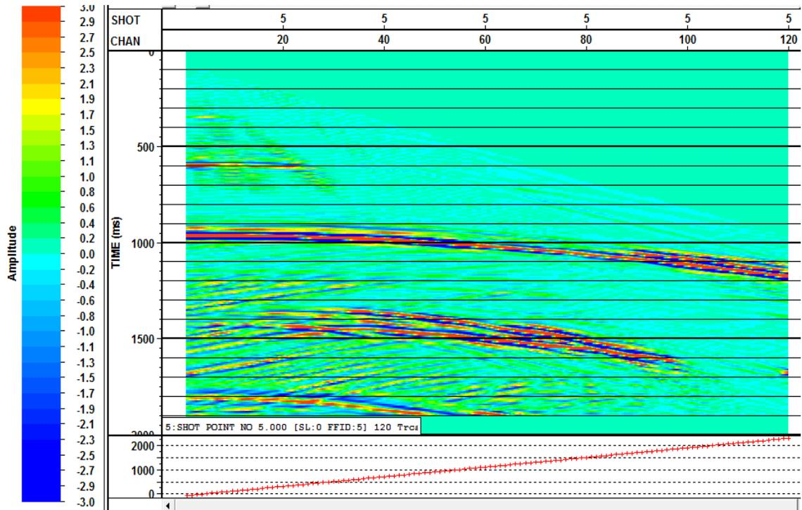
FIG 13. This figure shows the 5<sup>th</sup> shot record that has had a mute to kill the first breaks and an F-K filter to remove the ground roll. Using an F-K filter to remove the ground roll allowed the data on the channel interval to remain
