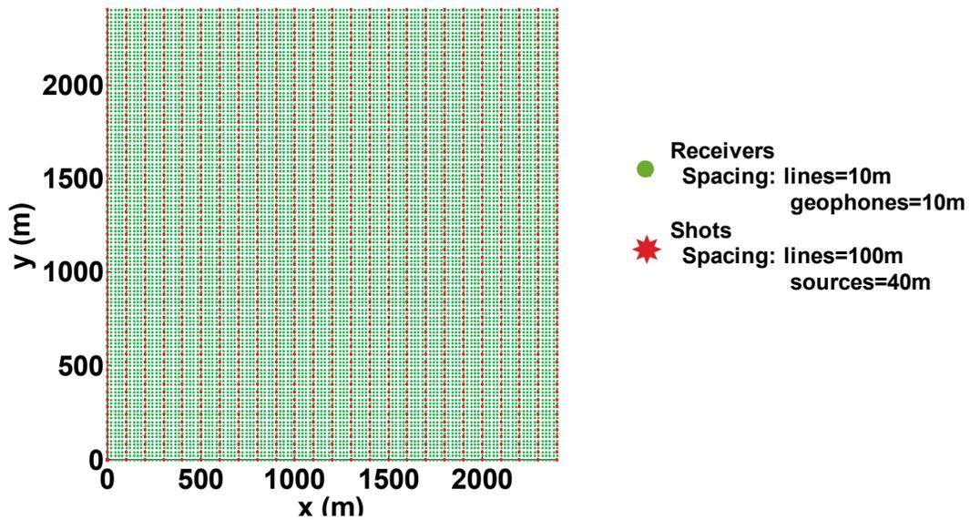
FIG 5. This figure shows the geometry of the synthetic survey. The geophones were laid on a 10m by 10m grid, these are represented by the green dots. The shots were laid in lines
