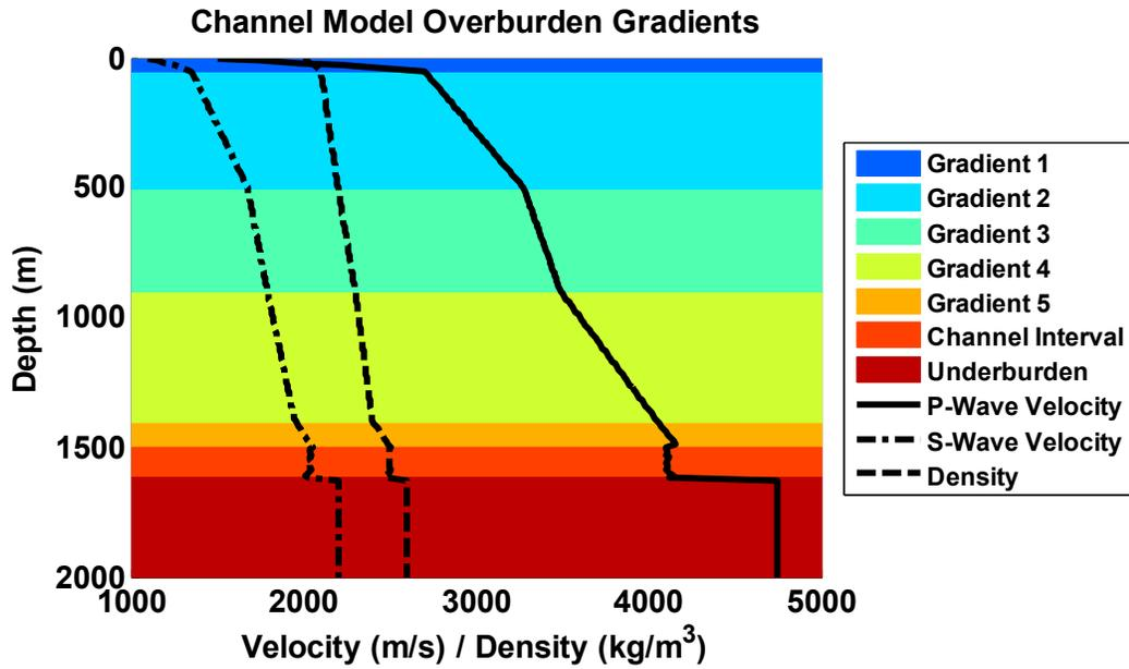
FIG 2. This figure shows the gradient overburden profile, based on the Blackfoot Field area in Alberta.
