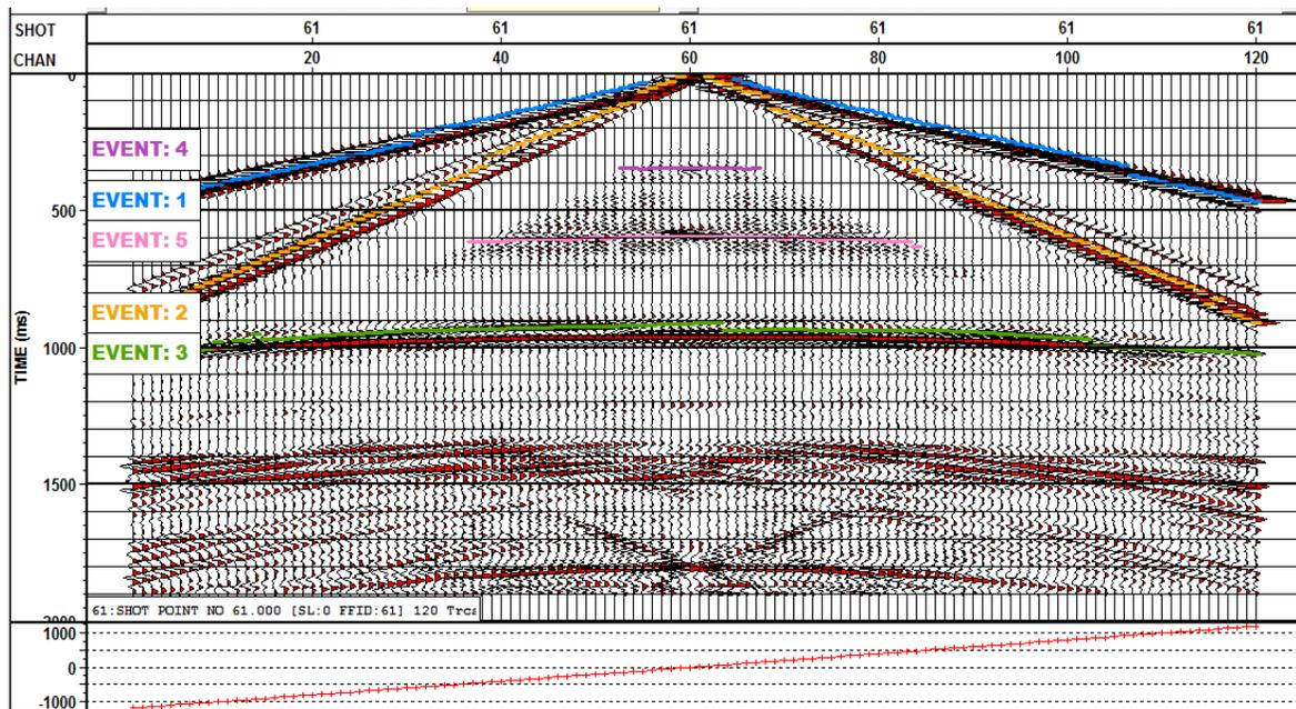
FIG 11. Shot 61 with 0.1 second bulk time shift, gain and AGC applied. Event 3 is the channel interval, indicated in green. Event 4, indicated in purple is an event created by the change in gradient 2 to 3. Event 5 is the gradient change between gradient 3 and 4; this event is indicated by pink.
