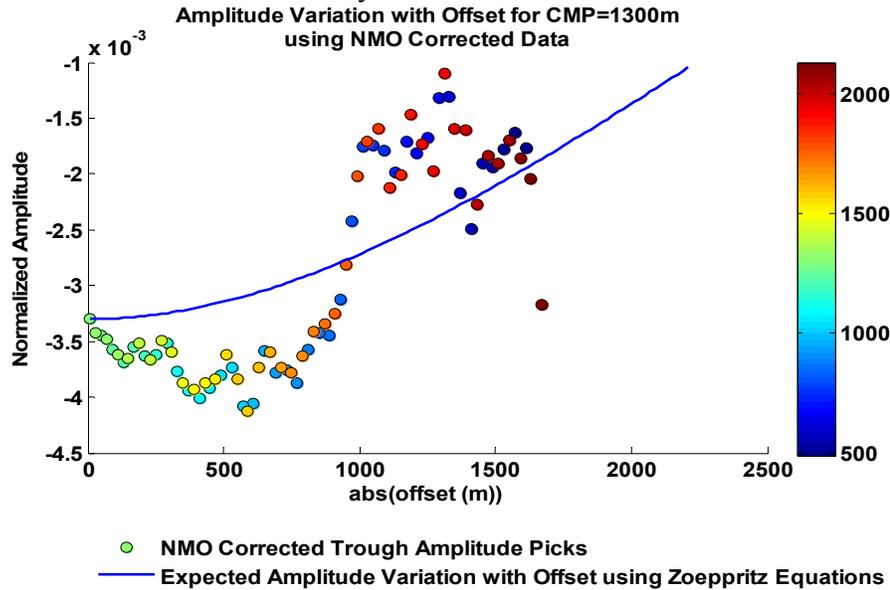
FIG 18. This figure shows the amplitude variation with offset for a common midpoint gather at 1300m using normal move out corrected data. At this common midpoint in the model there is another negative impedance contrast and a low  $V_p$ - $V_s$  ratio creating a possible target. The blue line is the theoretical, expected result where as the coloured dots are measured. The color of the dots indicates the y-coordinate of the geophone that recorded the data.
