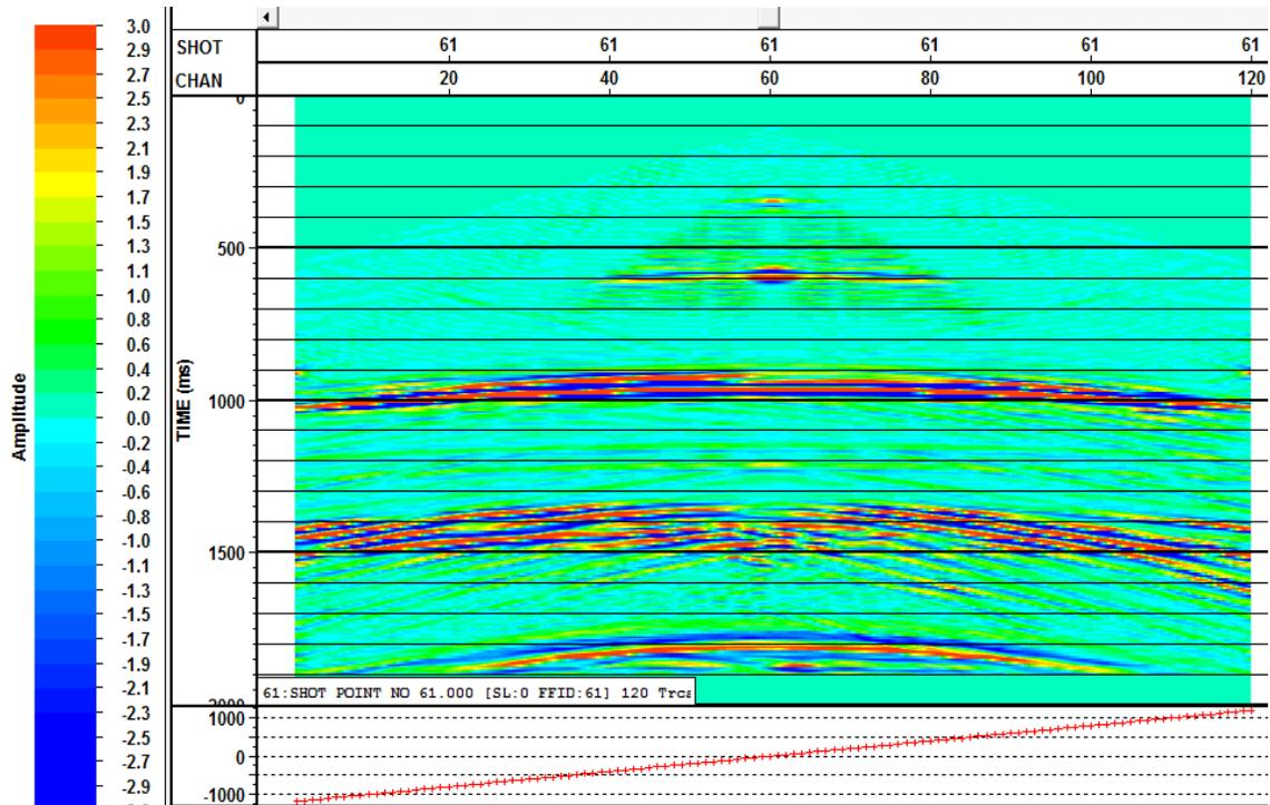
FIG 12. This figure shows the 61<sup>st</sup> shot record that has had a mute to kill the first breaks and an F-K filter to remove the ground roll.
