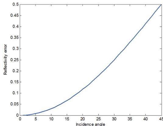
FIG. 3. Reflectivity error as a function of incidence angle.
