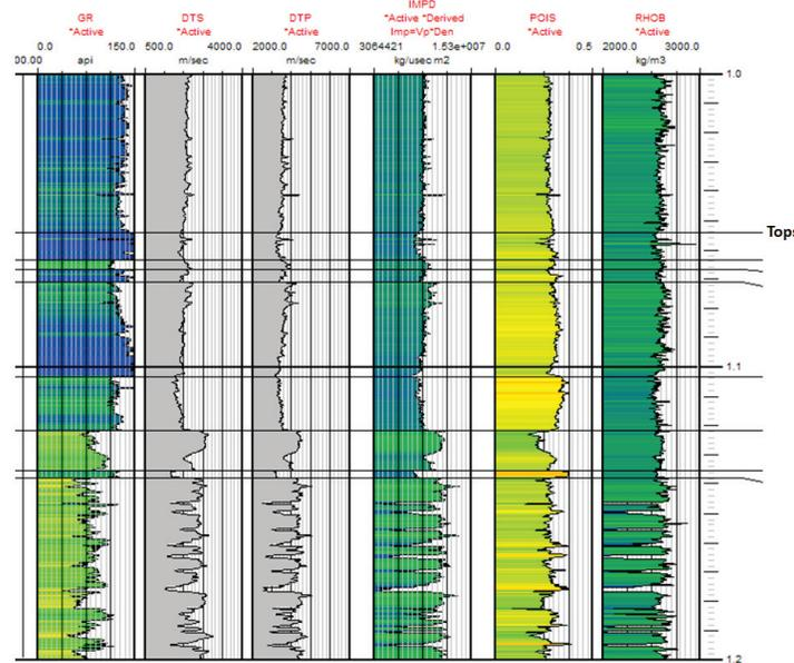
FIG. 1. Defined lithologies using a suite of well log measurements.
