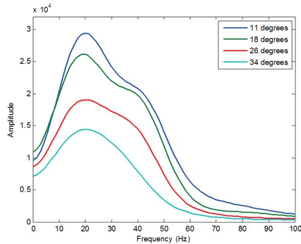
FIG. 4. Smoothed amplitude spectrum of four angle stacks used in an AVO inversion.
