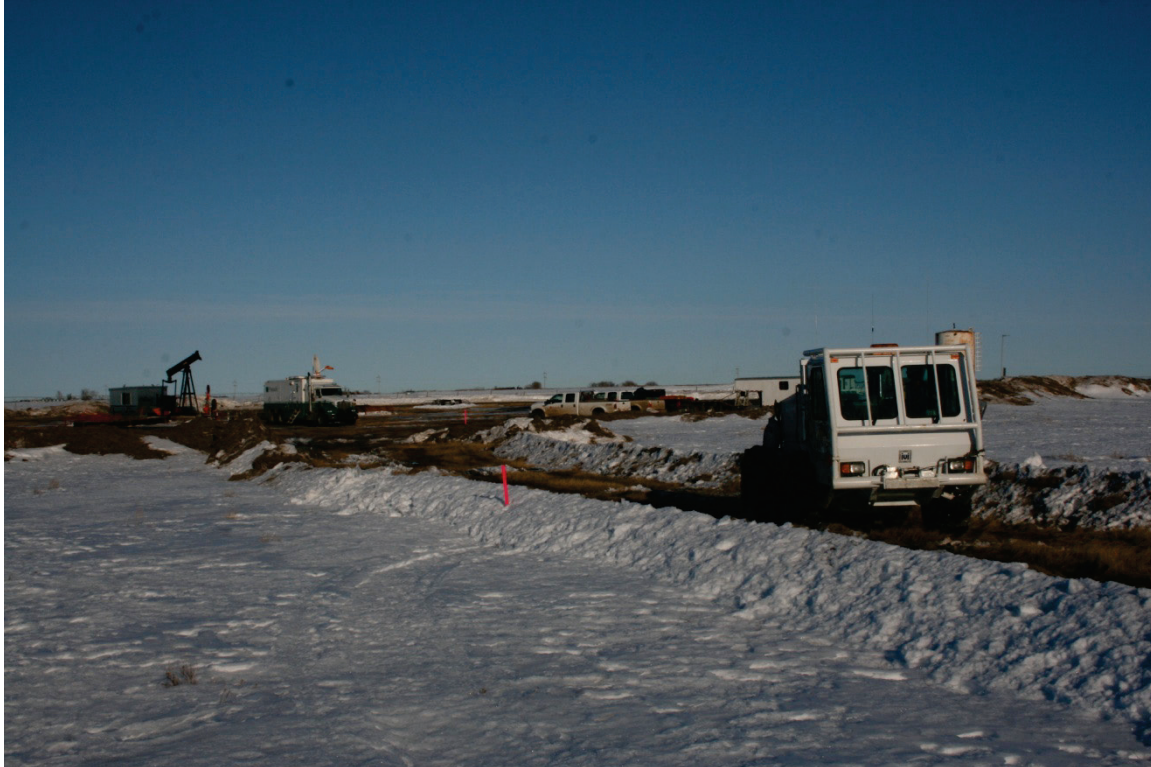
FIG. 1. Picture taken at field site, showing the surface conditions during seismic acquisition. The right side of the picture shows the CREWES EnviroVibe.
