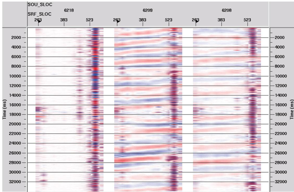
FIG. 12. Uncorrelated data from 4.5 Hz 1-C geophones one flag east of seismometer stations for VPs 218, 209, and 208. Trace length is 34 seconds. ProMAX trace display scaling: entire screen with gain set to one. Vertical fold is one.
