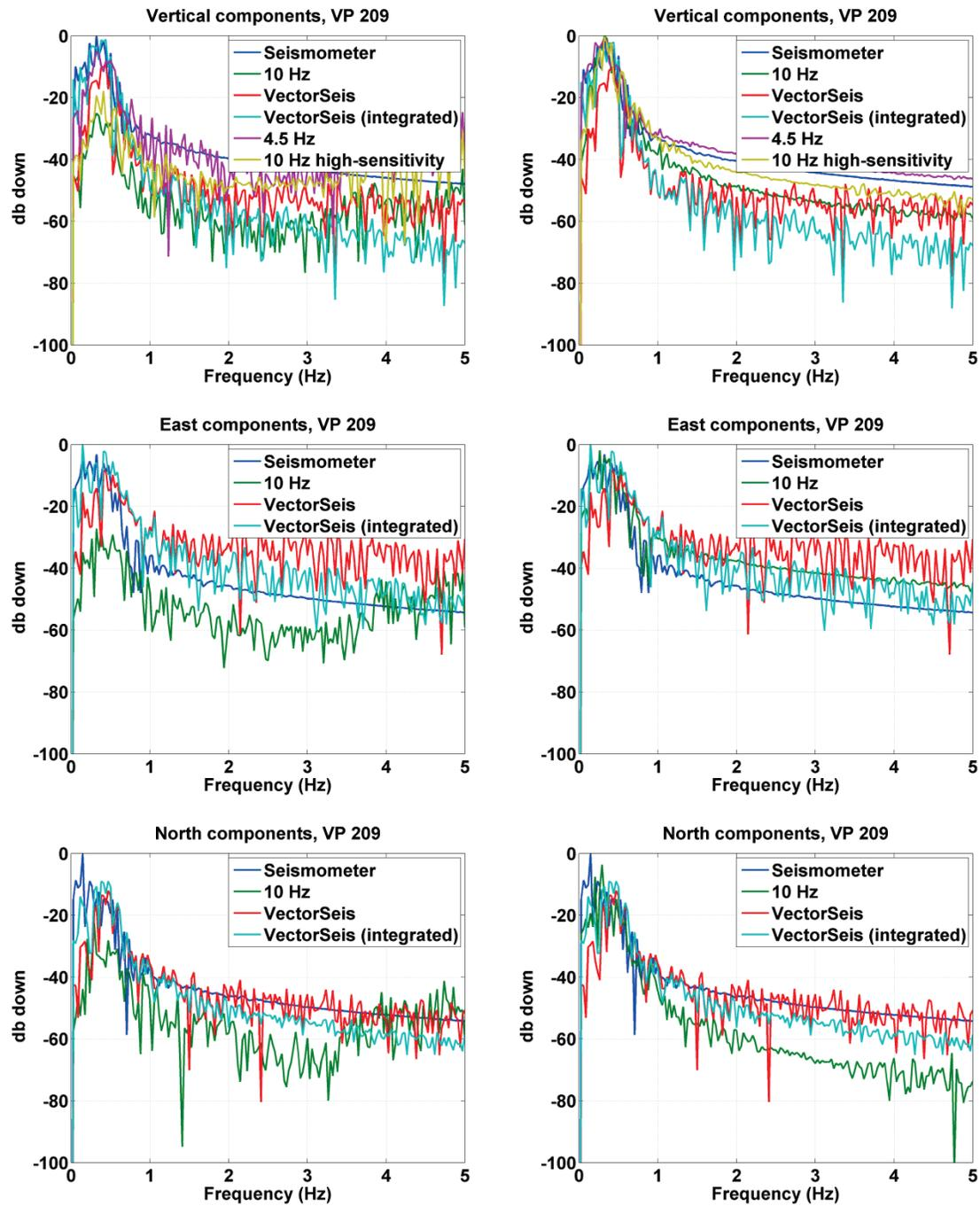
FIG. 18. The first five Hertz of amplitude spectra for uncorrelated data from VP 209, during high-amplitude secondary arrivals from the Vancouver Island earthquake. Left; Before correcting for geophone response. Right; After correcting for geophone response.
