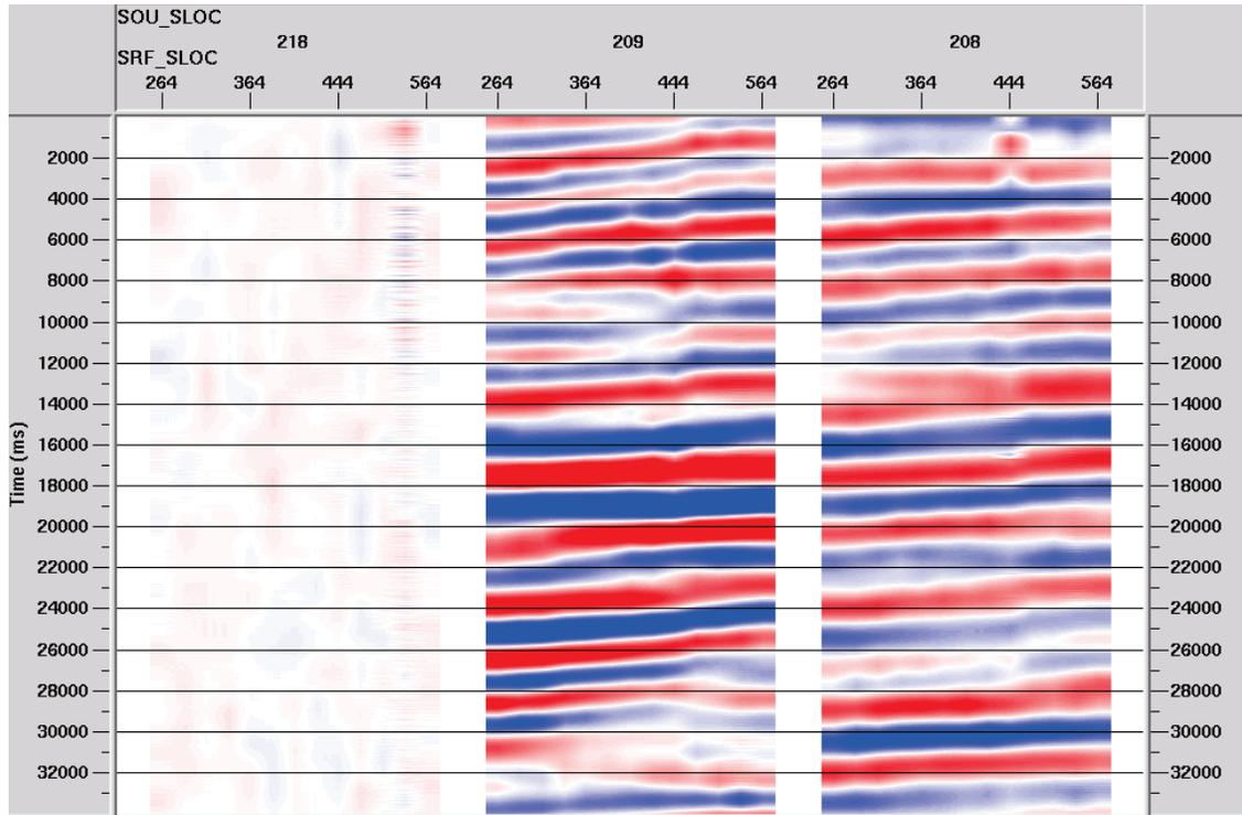
FIG. 9. Figure 8 after correcting for geophone response below 10 Hz. Trace length is 34 seconds. ProMAX trace display scaling: entire screen with gain set to one. Vertical fold is one.
