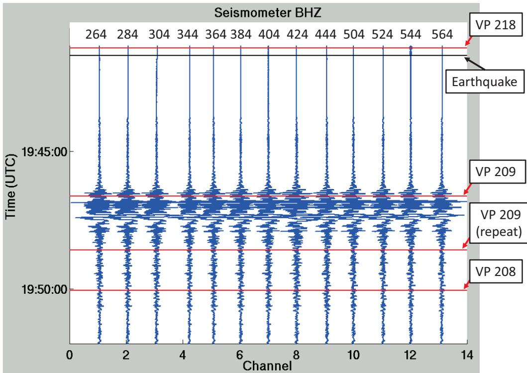
FIG. 2. Vertical component of uncorrelated data from seismometers. Trace length is 11.5 minutes. The time of the first sweep (of two sweeps per vibe point) is shown as red lines. The time of the earthquake is shown as a black line (see Appendix A).
