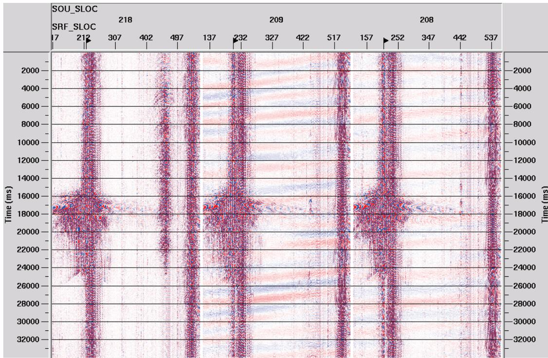
FIG. 4. Vertical component of uncorrelated data from 10 Hz 3-C geophones for VPs 218, 209, and 208. Trace length is 34 seconds. ProMAX trace display scaling: entire screen with gain set to fifteen. Vertical fold is one.
