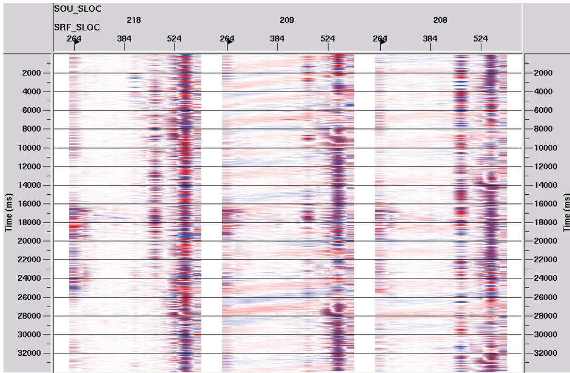
FIG. 8. Vertical component of uncorrelated data from 10 Hz 3-C geophones at thirteen seismometer stations for VPs 218, 209, and 208. Trace length is 34 seconds. ProMAX trace display scaling: entire screen with gain set to one. Vertical fold is one.
