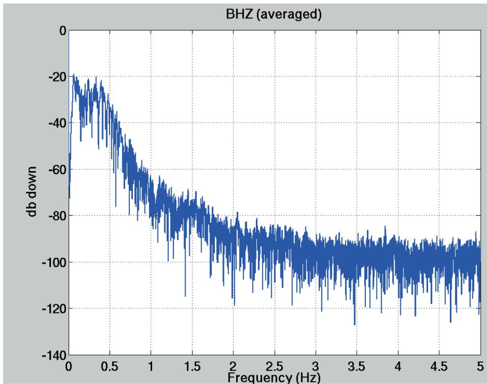
FIG. 3. First 5 Hz of the amplitude spectra for the traces shown in Figure 1. There is an apparent DC bias in this figure. Earthquake energy is primarily below 2 Hertz.
