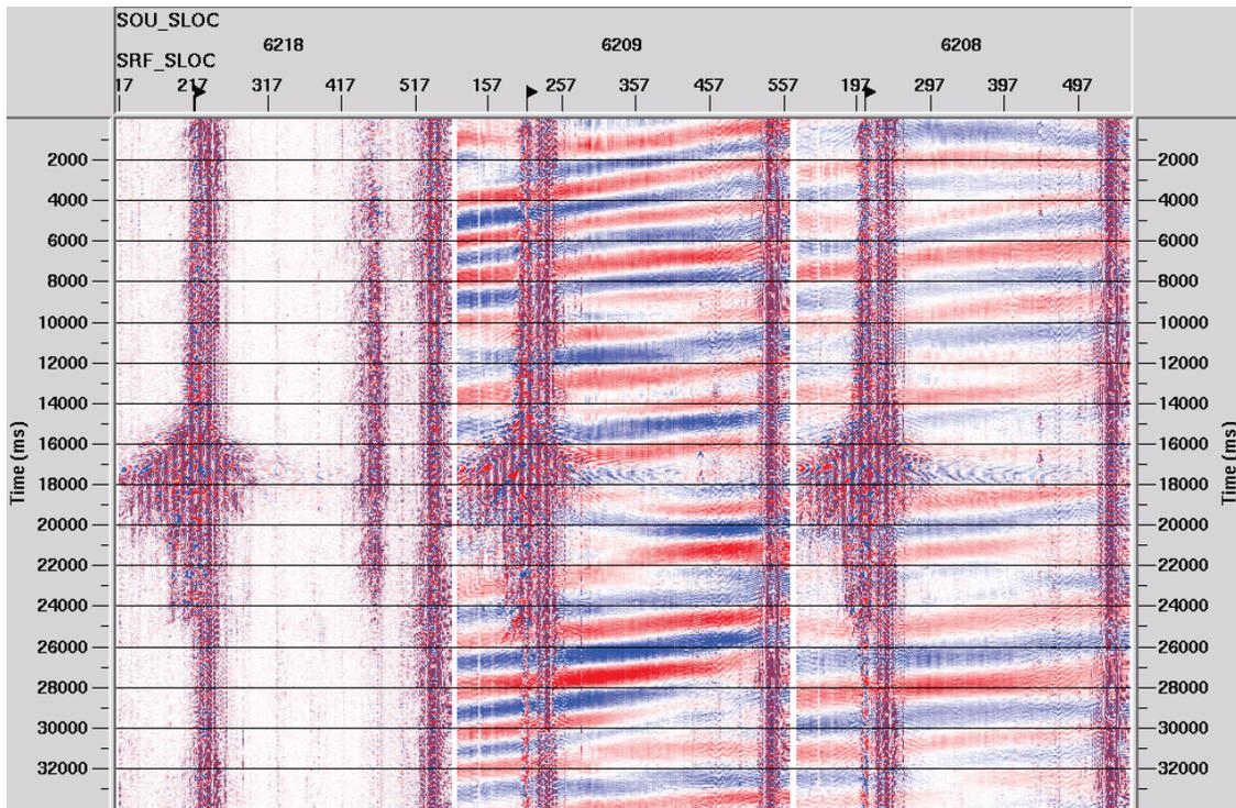
FIG. 6. Uncorrelated data from 4.5 Hz 1-C geophones for VPs 218, 209, and 208. Trace length is 34 seconds. ProMAX trace display scaling: entire screen with gain set to fifteen. Vertical fold is one.
