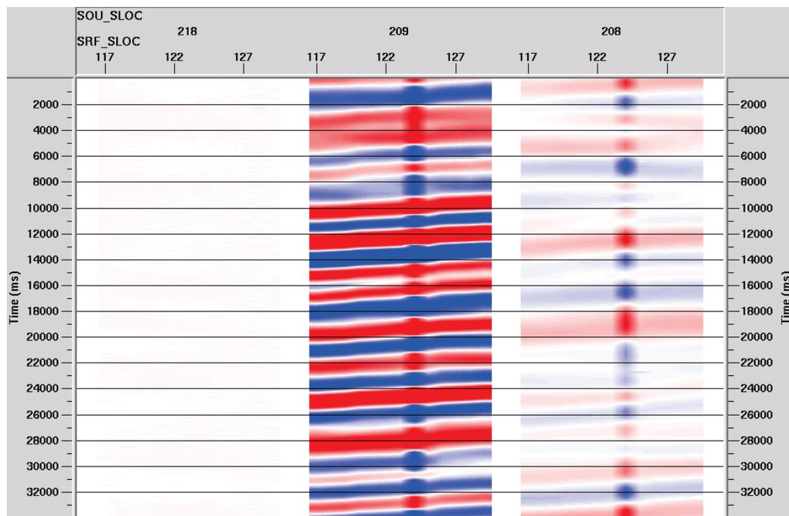
FIG. 16. Uncorrelated data from the vertical component of seismometers for VPs 218, 209, and 208. Trace length is 34 seconds. ProMAX trace display scaling: entire screen with gain set to one. Trace fold is one.
