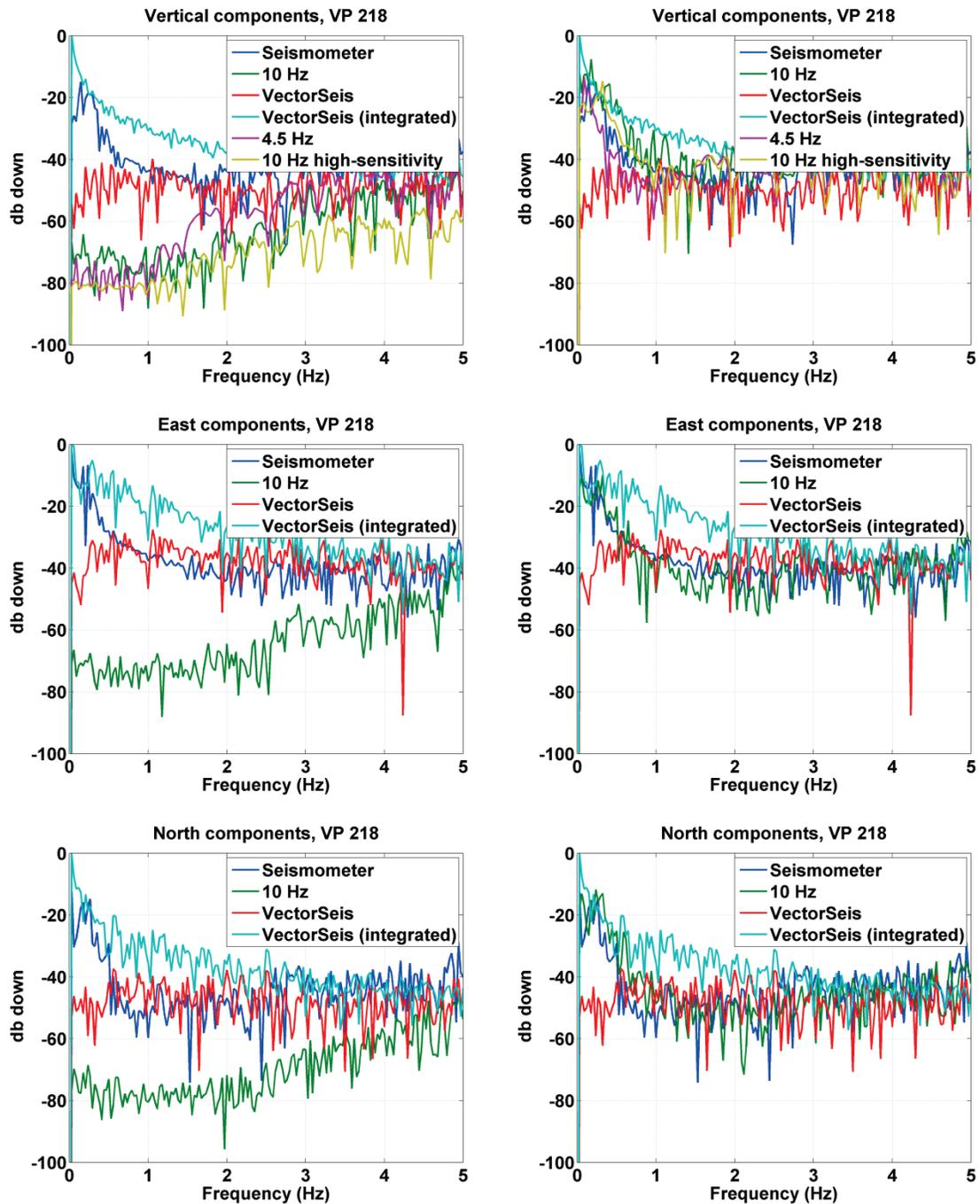
FIG. 17. The first five Hertz of amplitude spectra for uncorrelated data from VP 218, prior to any arrivals from the Vancouver Island earthquake. Left; Before correcting for geophone response. Right; After correcting for geophone response.
