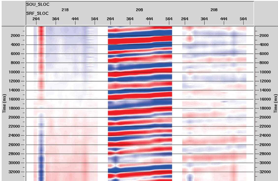
FIG. 15. Figure 14 integrated, Apparent trace dc bias removed for display. Integration has introduced low-frequency noise (eg. VP 218, left-hand side), as expected.
