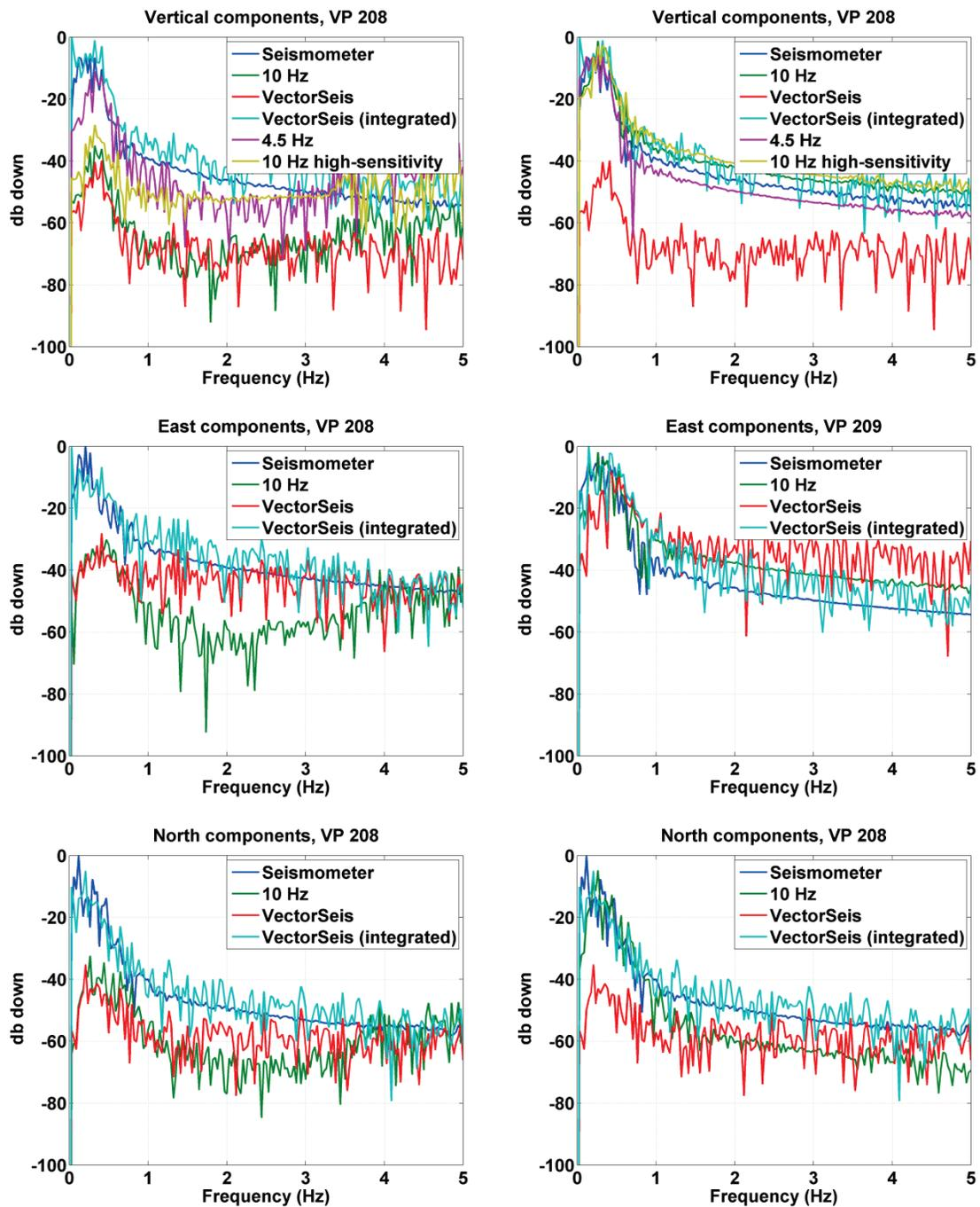
FIG. 19. The first five Hertz of amplitude spectra for uncorrelated data from VP 208, during secondary arrivals from the Vancouver Island earthquake. Left; Before correcting for geophone response. Right; After correcting for geophone response.
