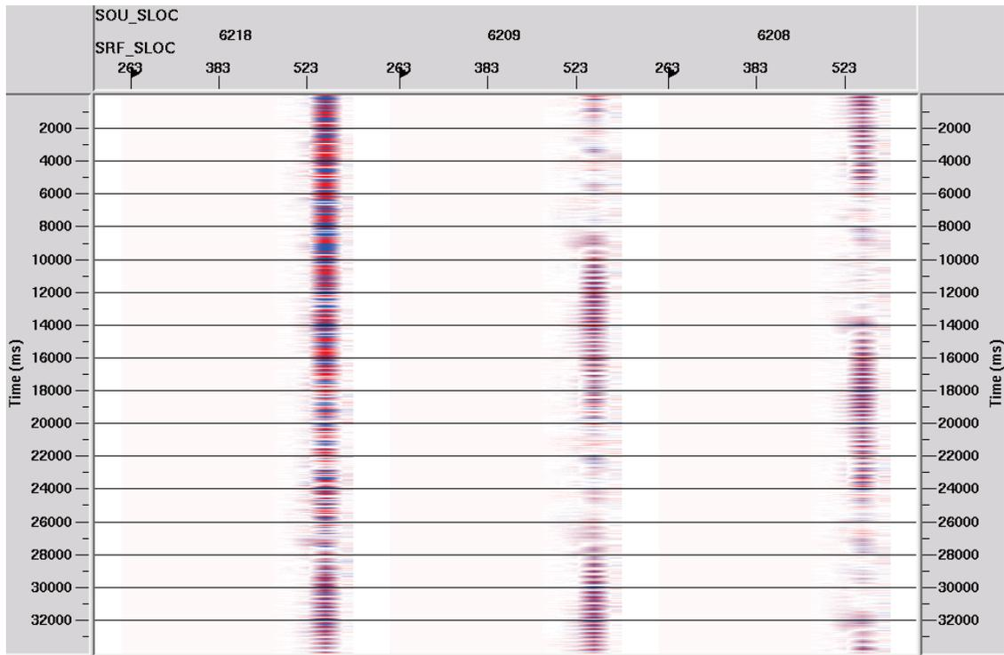
FIG. 10. Uncorrelated data from four 10 Hz high-sensitivity geophones one flag east of seismometer stations for VPs 218, 209, and 208. Trace length is 34 seconds. ProMAX trace display scaling: entire screen with gain set to one. Vertical fold is one.
