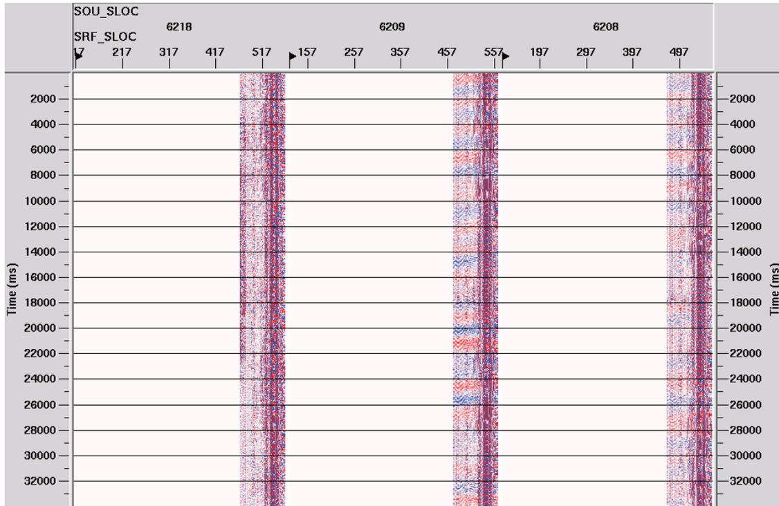
FIG. 5. Uncorrelated data from 10 Hz high-sensitivity geophones for VPs 218, 209, and 208. Trace length is 34 seconds. ProMAX trace display scaling: entire screen with gain set to five. Vertical fold is one.
