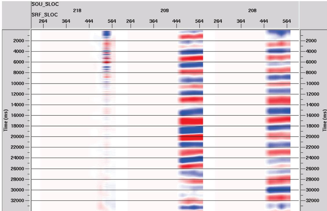
FIG. 11. Figure 10 after correcting for geophone response below 10 Hz. Trace length is 34 seconds. ProMAX trace display scaling: entire screen with gain set to one. Vertical fold is one.
