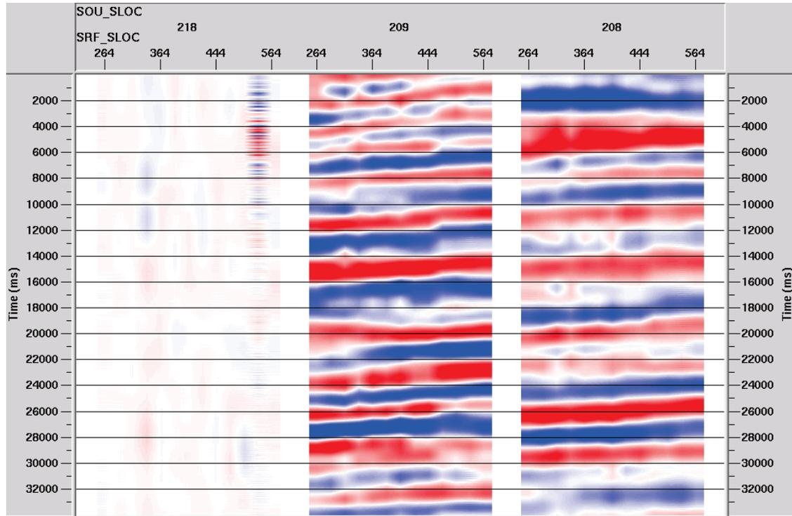
FIG. 13. Figure 12 after correcting for geophone response below 4.5 Hz. Trace length is 34 seconds. ProMAX trace display scaling: entire screen with gain set to one. Vertical fold is one.
