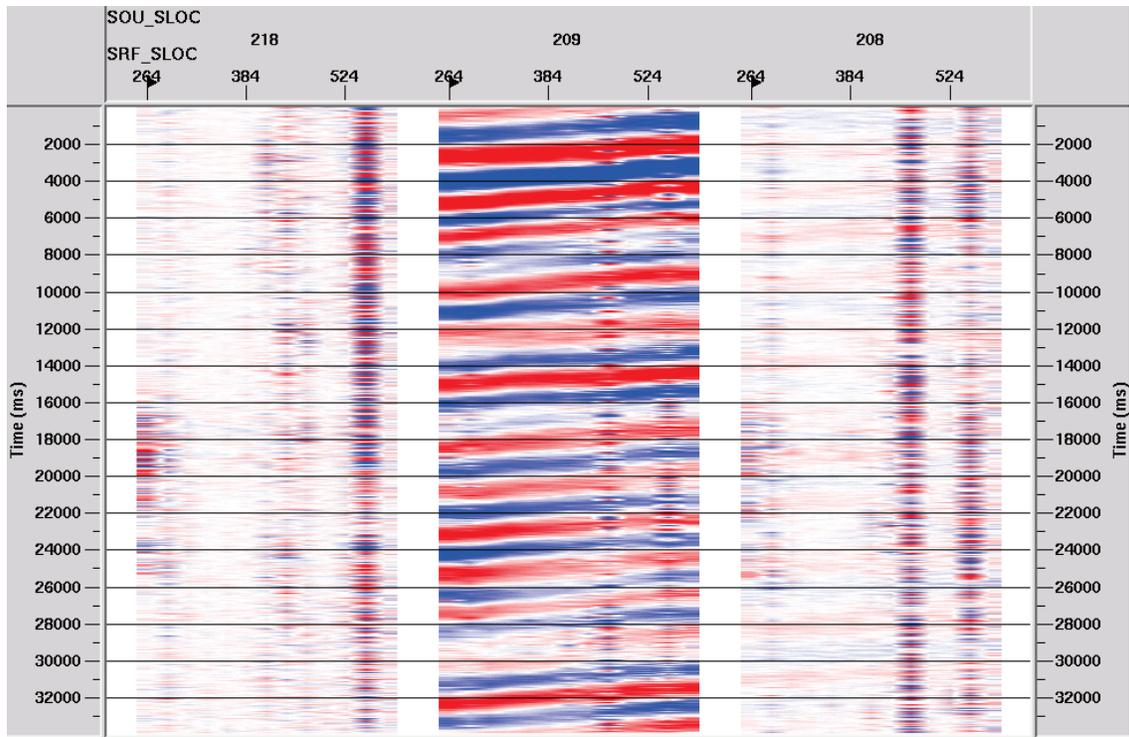
FIG. 14. Uncorrelated data from the vertical component of VectorSeis accelerometers at thirteen seismometer stations for VPs 218, 209, and 208. Trace length is 34 seconds. ProMAX trace display scaling: entire screen with gain set to one. Vertical fold is two.
