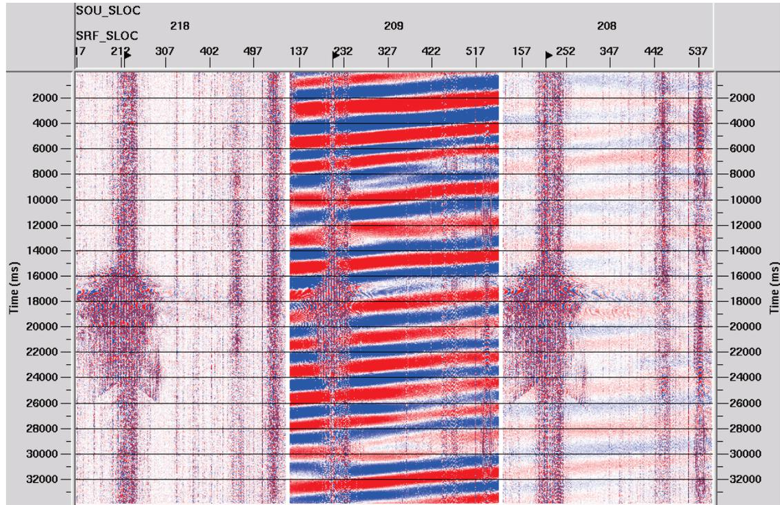
FIG. 7. Uncorrelated data from the vertical component of VectorSeis accelerometers for VPs 218, 209, and 208. Trace length is 34 seconds. ProMAX trace display scaling: entire screen with gain set to fifteen. Vertical fold is two.
