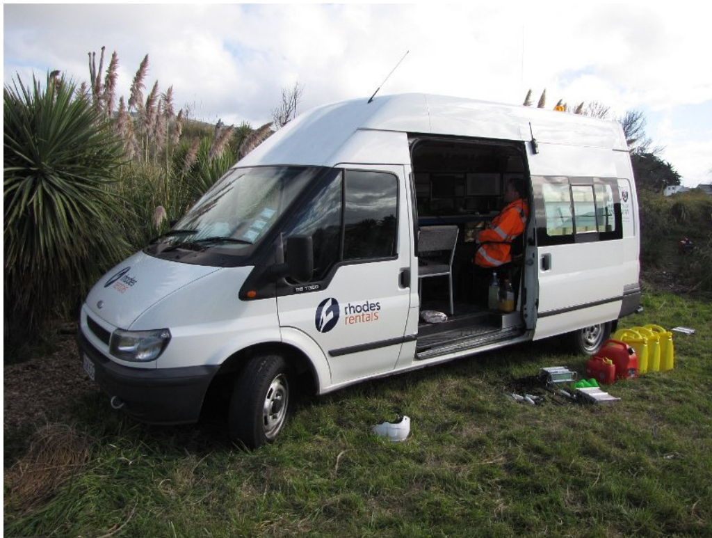
FIG. 7. Ford Transit van as seismic recorder.
