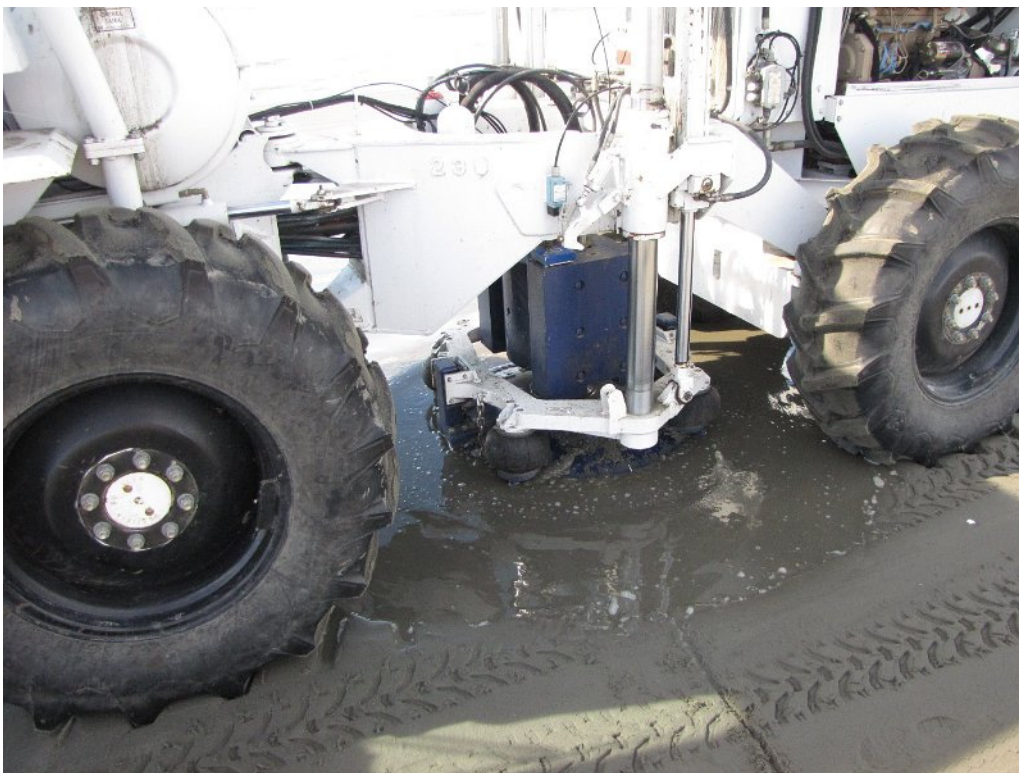
FIG. 12. Beach sand liquefied during Vibe sweep if sand was too wet. Solution: move vibe point higher up the beach, away from the ocean.
