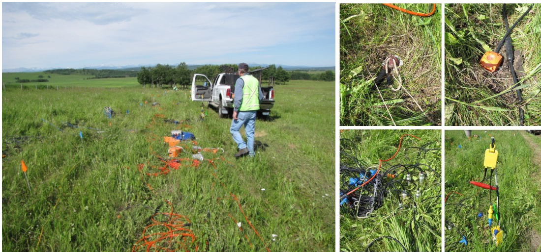
FIG. 2. The receiver line looking west and the four sensors used. Top left: vectorseis, top right: SM7 3C, bottom left: GS-32CT pods, bottom right: Autoseis with SM24.
