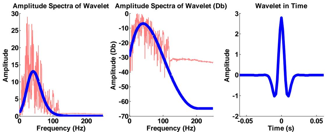
FIG 4: The wavelet used to create synthetic seismograms. The average trace spectra is shown in red where the wavelet estimate is shown in blue (bold). The wavelet was determined to be a zero phase fourth order polynomial approximation in decibels.
