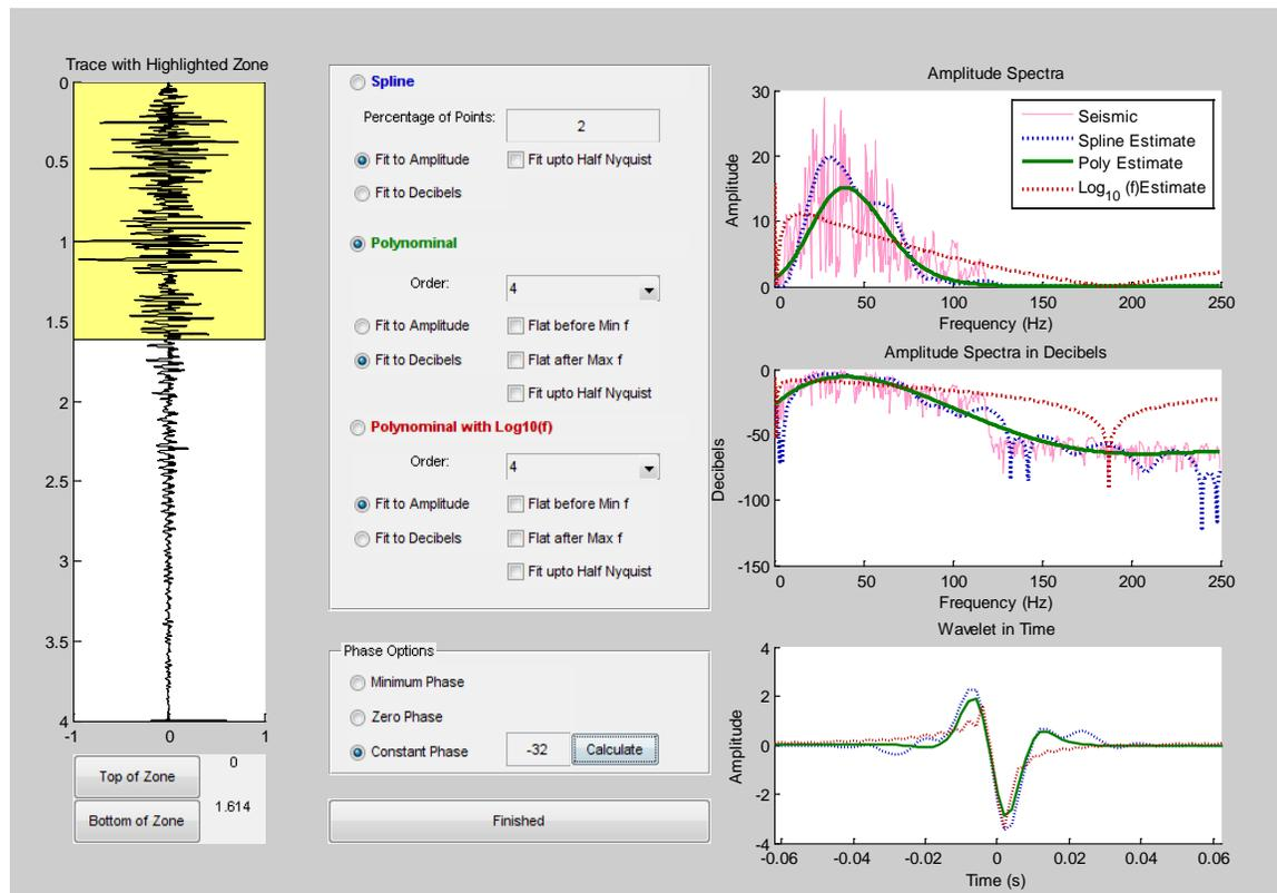
FIG 9: The interface for WaveletEstimator. The zone that is used in calculating the amplitude spectra from the trace is indicated in yellow on the left hand side. The amplitude spectra of the seismic trace and the estimated wavelet are shown in top right hand corner, and in decibels just below. The wavelet is shown in bottom hand corner in time. In the center are the wavelet options. Each wavelet type is identified by a separate color which can be seen in each of the displays.
