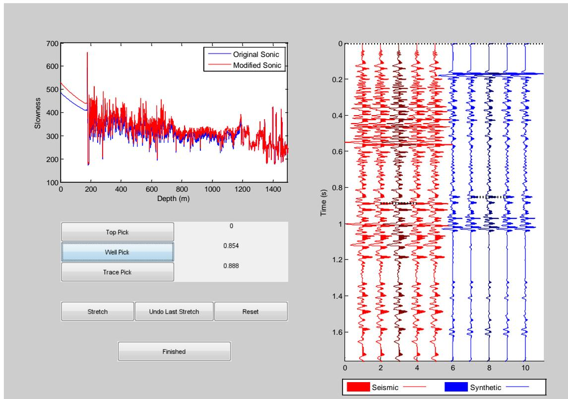
FIG 10: The interface of Stretchwell. The synthetic seismogram is shown in blue and the seismic data is shown in red. The two sonic curves are shown in the upper left hand corner of the display.
