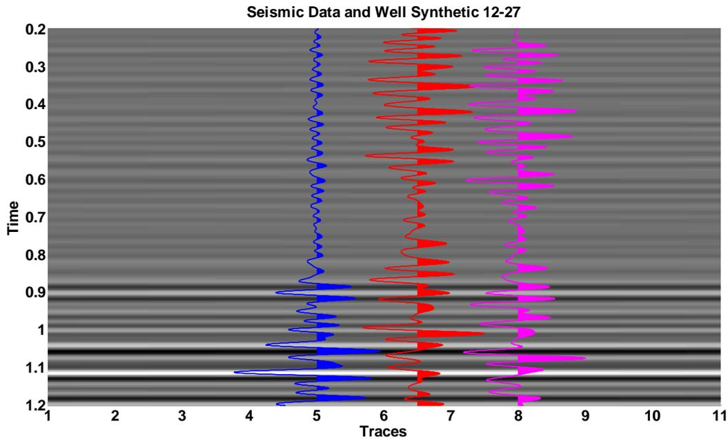
FIG 5 : Well tie for well 12-27. The trace located at the well location is shown in blue, the non static shifted synthetic trace is shown in red and the static shifted synthetic is shown in pink.
