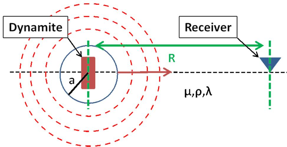
FIG. 1. Graphical depiction of the Sharpe Hollow Cavity Model. The source and receiver are assumed to be at zero depth in an infinite half space with parameters  $\mu$ ,  $\rho$ , and  $\lambda$ . The emitted waves (shown in red) propagate directly from the walls of the cavity.
