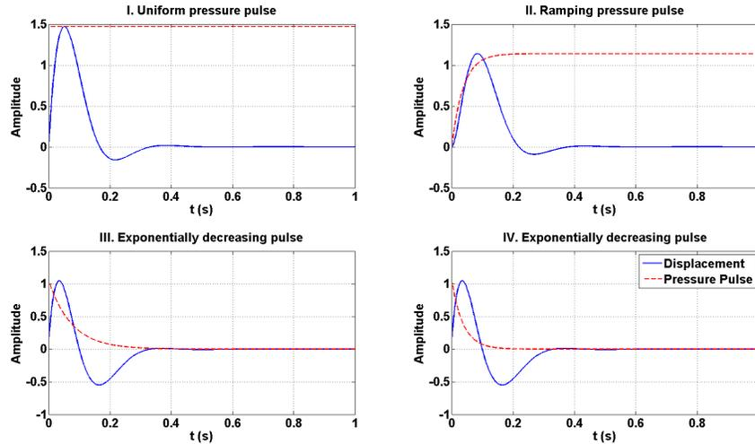
FIG. 2. Particle displacements resulting from applications of arbitrary pressure pulses. I)  $p(t) = p_o$ . II)  $p(t) = p_o(1 - e^{-\sqrt{2}\omega\tau})$ . III)  $p(t) = p_o e^{-\omega\tau/\sqrt{2}}$ . IV)  $p(t) = p_o e^{-\sqrt{2}\omega\tau}$ . The decreasing exponential shown in III most is the the pulse that is most likely to resemble that of an explosion since the application of pressure is approximately an impulse, which rapidly deteriorates or "burns out" in a short amount of time.
