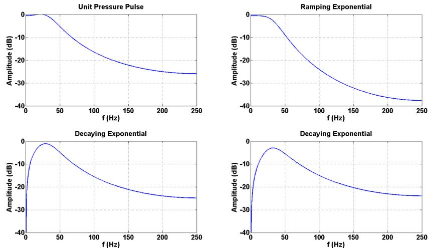
FIG. 3. A series of frequency spectra that result from the pressure pulses shown in Figure 2. The choice of pressure pulse for this model alters the frequency spectra significantly in both the high and low frequencies.
