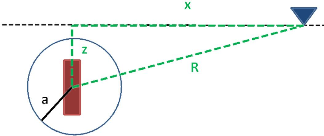
FIG. 4. Graphical depiction of a buried charge using the SHCM. The charge is buried at a depth of  $z$  to the center of the source at a distance  $x$  from the receiver.
