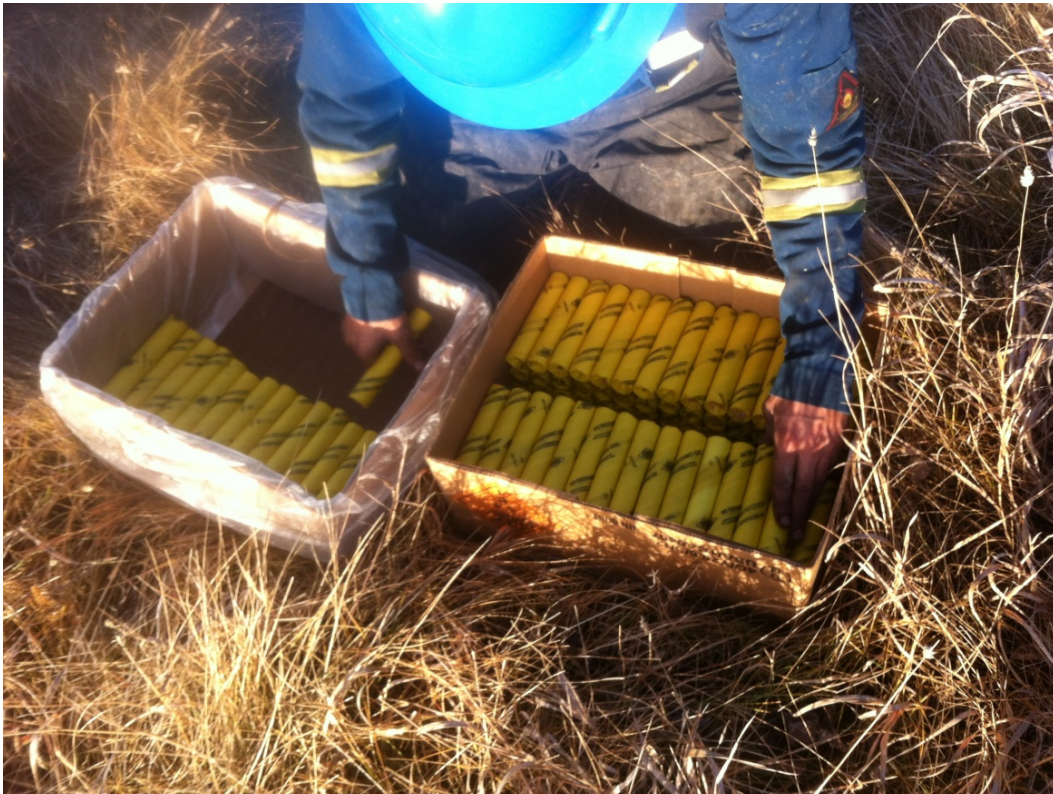
FIG. 7. One hundred and fifty 0.125 kg dynamite charges.
