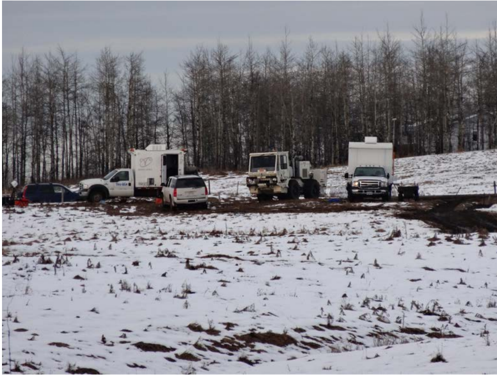
FIG. 5. G3i recording truck (left), UNIVIB, and Aries recording truck (right) parked 270 m from the closest geophone.
