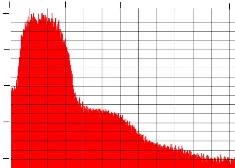
FIG. 4. Scaled source spectrum for the piezopin transducers used in the source array for surveying the physical model.
