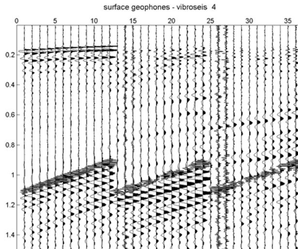
Figure 6: Vibroseis data recorded from conventional surface three-component geophones with identical elements for comparison.
