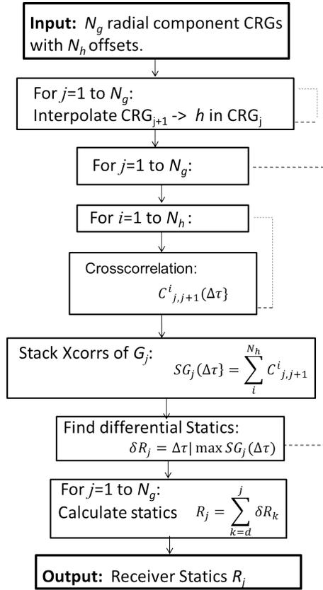
FIG. 2. Flow diagram of the method for PS-wave receiver statics correction.
