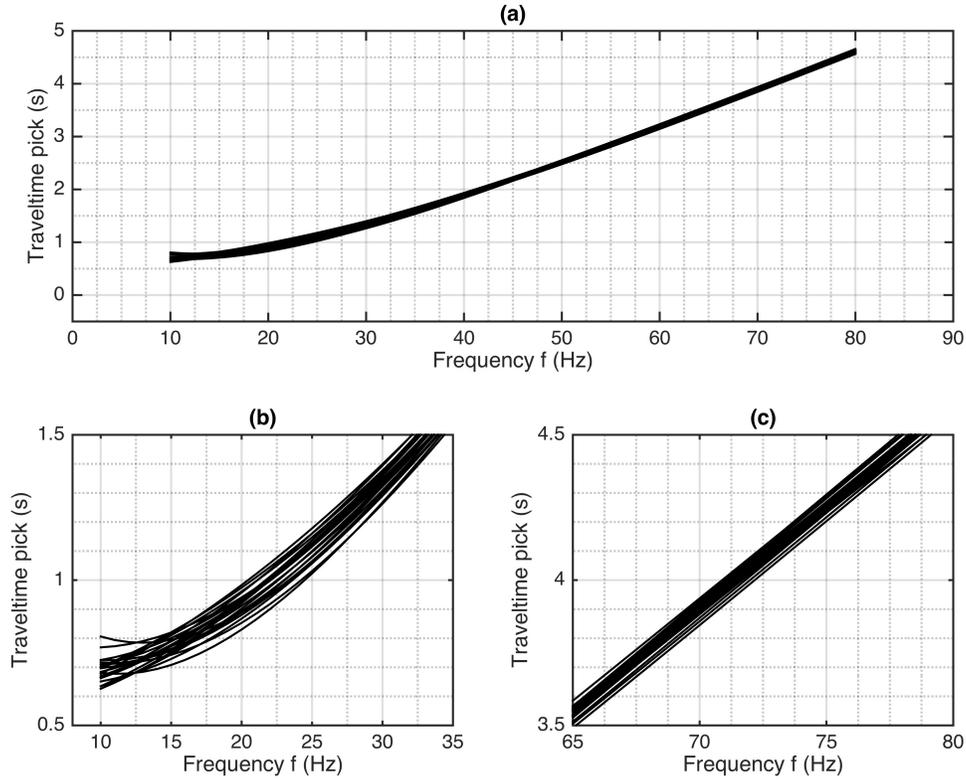
FIG. 8. Summary of 20 travel time vs. frequency curves. (a) Full picks between 10Hz and 80Hz. Note the departure from linear at low frequencies. (b)-(c) Details at low and high frequency ranges.
