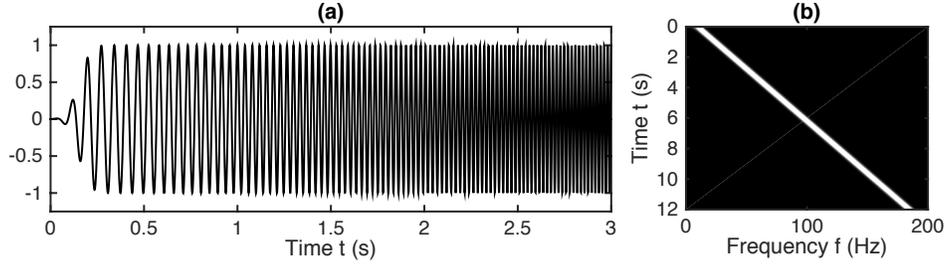
FIG. 4. The programmed sweep used in the VSP survey. (a) The first 3.0s of the sweep in the time domain, with cosine taper at early times. (b) The first 12.0s of the sweep in the time-frequency domain via the Gabor transform.
