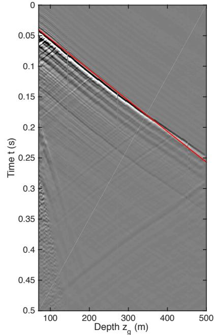
FIG. 2. Near offset shot record, with direct arrival in the upper 150m picked and illustrated with a solid red line.
