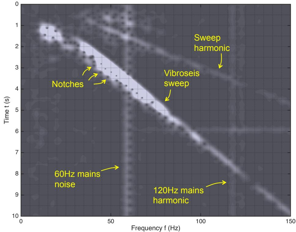
FIG. 6. Gabor spectrum of a single uncorrelated trace (depth  $z_g = 76\text{m}$ , offset  $x_s = 320\text{m}$ ). Notches, mains noise and harmonics, and sweep and harmonic are labelled. Event labelled “vibroseis sweep” is analyzed in this study.
