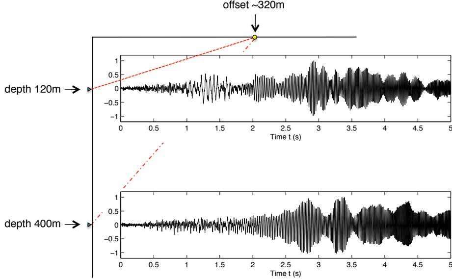
FIG. 5. Uncorrelated signals arriving from a source offset 320m from the borehole at geophones at depths of 120m and 400m deep.
