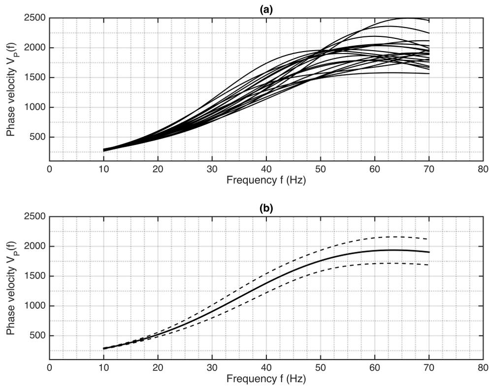
FIG. 10. (a) Phase velocity curves calibrated using the space-time and spectral analysis results illustrated in Figures 2 and 3. (b) Mean (solid line) and  $\pm$  one standard deviation (dashed line).
