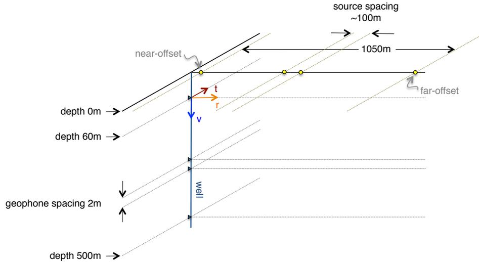
FIG. 1. Geometry and scale of the VSP experiment.
