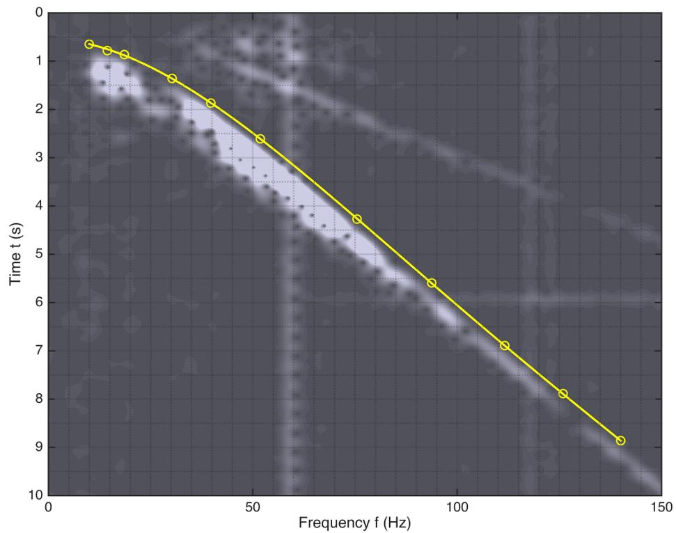
FIG. 7. Example of arrival time picking procedure. A smooth variation of arrival time with frequency is assumed, such that 10-15 picks can be fit with a low (4<sup>th</sup>) order polynomial.
