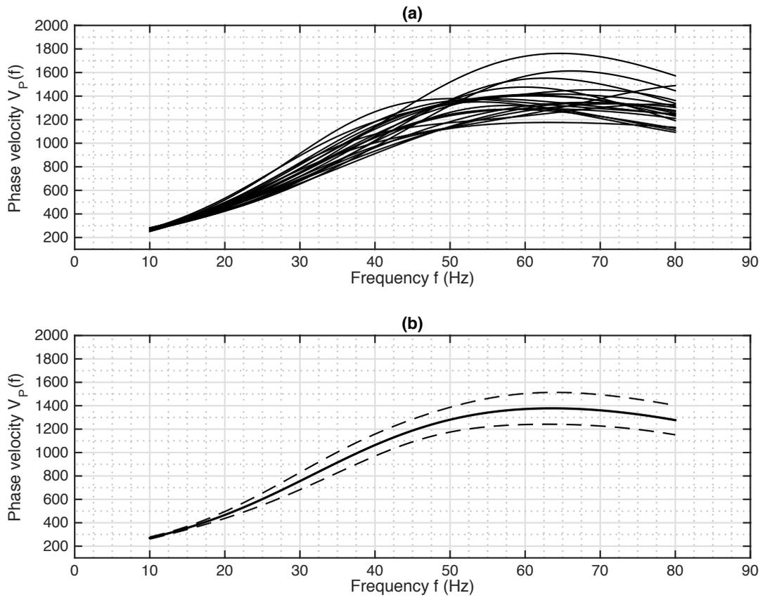
FIG. 9. Raw phase velocity estimation results: (a) for each of twenty geophone responses; (b) the mean (solid line) and  $\pm$  one standard deviation (dashed line).
