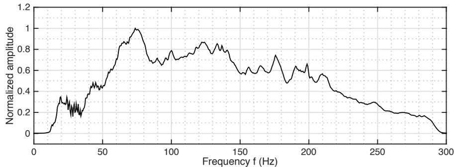
FIG. 3. Average amplitude spectrum of the zero offset traces illustrated in Figure 2.
