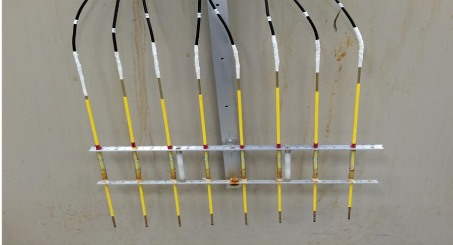
Figure 6: Array of eight piezopin receiver transducers. The receiver real spacing is 40mm; the scaled spacing is 400m.
