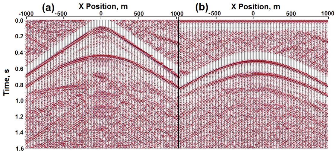
Figure 8: Common source gathers for two receiver lines, recorded using single-source shooting. Receiver line offset = (a) 140m; (b) 740m.
