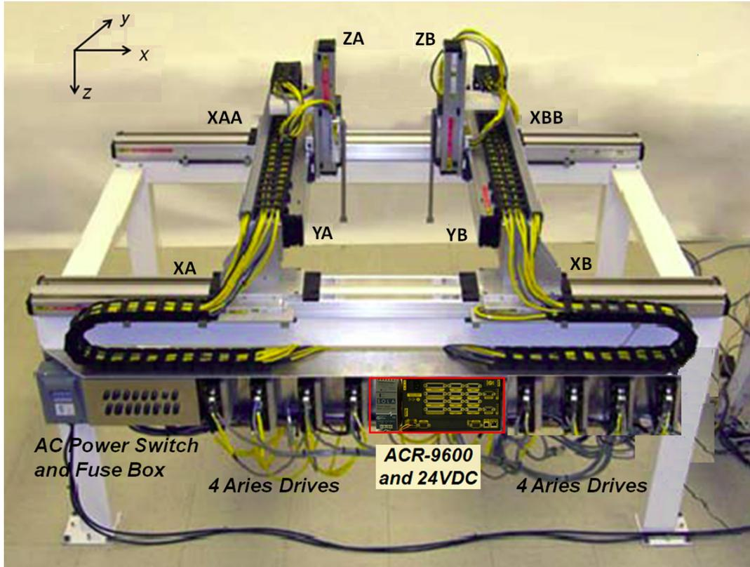
Figure 2: CREWES 3D Positioning System, with the upgraded motor drive controller ACR-9600 and its 24 VDC power supply. The Z1 and Z2 404LXR linear motors are mounted in a way that enables their forcers/carriers to approach each other as closely as possible in the X-direction.
