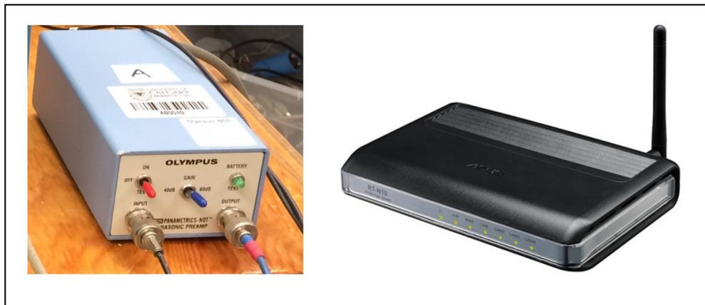
Figure 5: Left - Olympus 5660B Ultrasonic preamplifier. Right - ASUS RT-N10 LAN router
