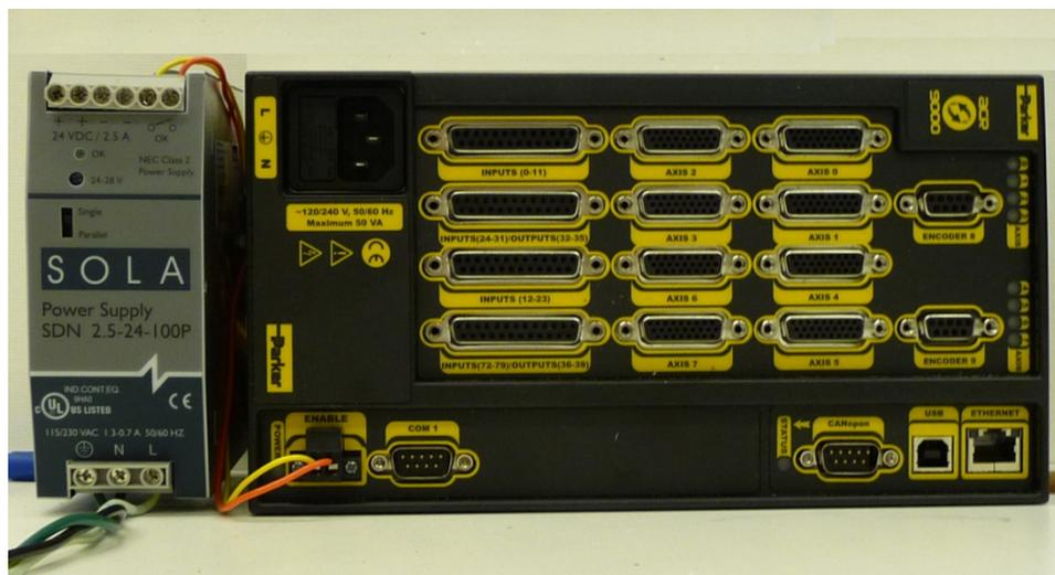
Figure 3: The Sola 24 VDC power supply and the front panel of the Parker-Hannifin ACR-9600 motor controller (Model No. ACR9000-P3-U8-B0).
