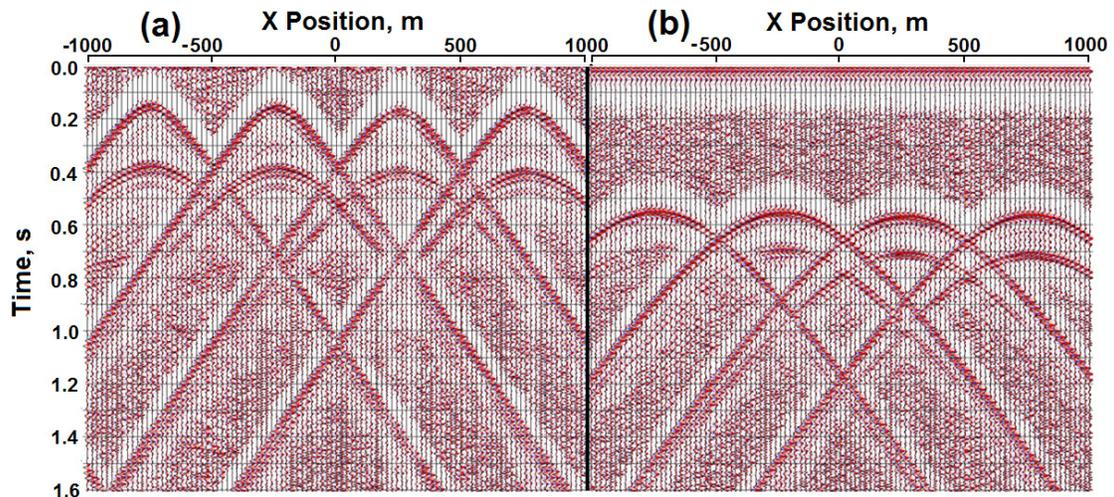
Figure 9: Common source gathers for two receiver lines, acquired using simultaneous shooting of four sources. Receiver line offset = (a) 200m; (b) 800m.
