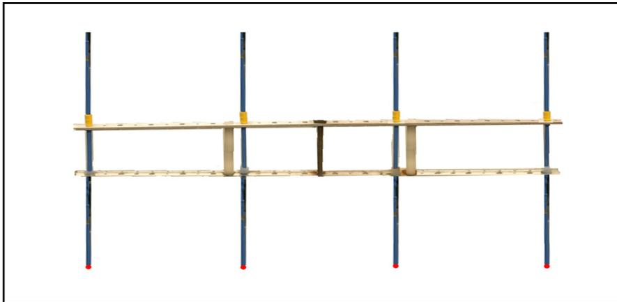
Figure 7: Array of four piezopin source transducers for simultaneous shooting. The source real spacing is 100mm; the scaled spacing is 1000m.
