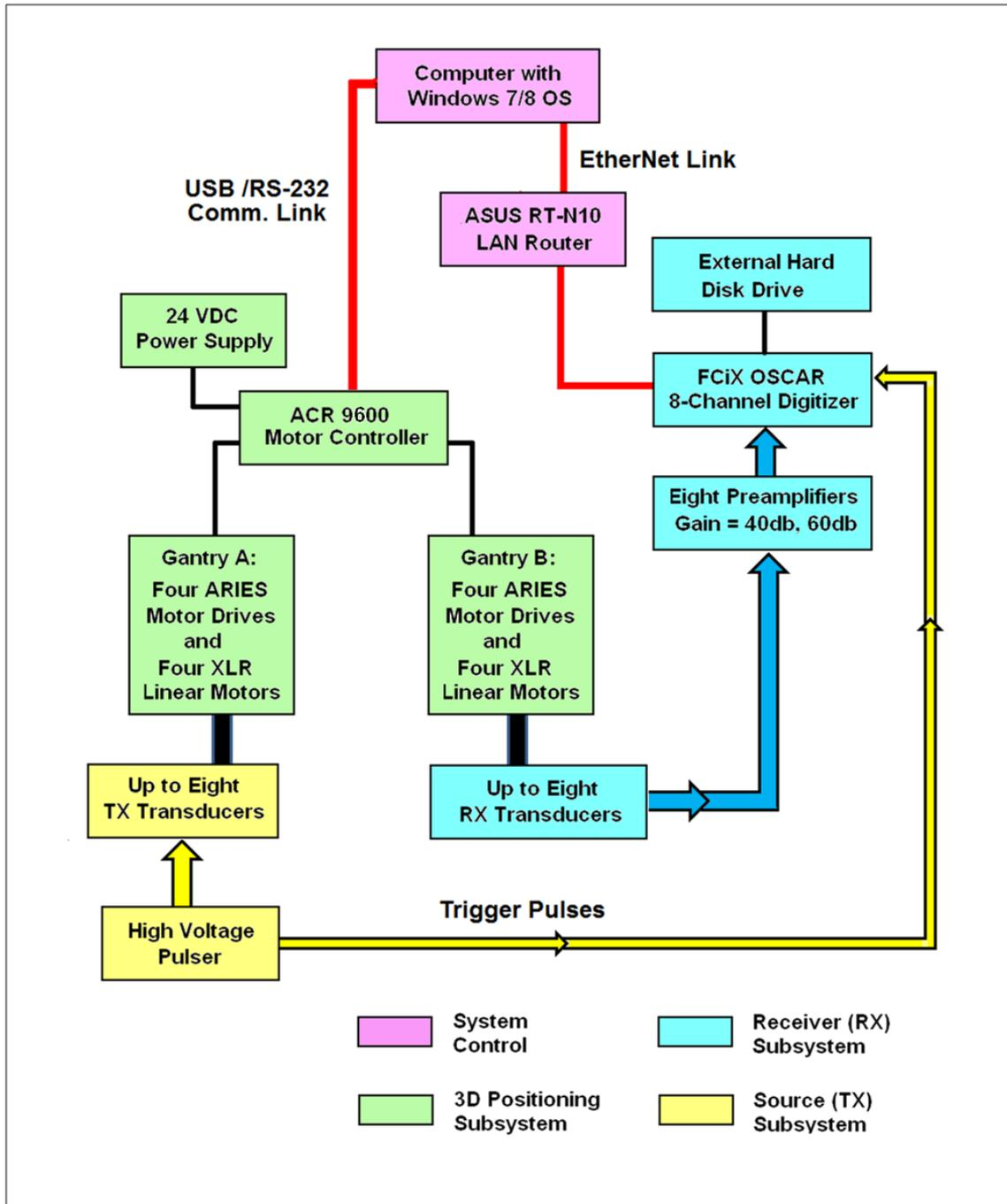
Figure 1: Block diagram of upgraded CREWES Seismic Physical Modeling Facility.
