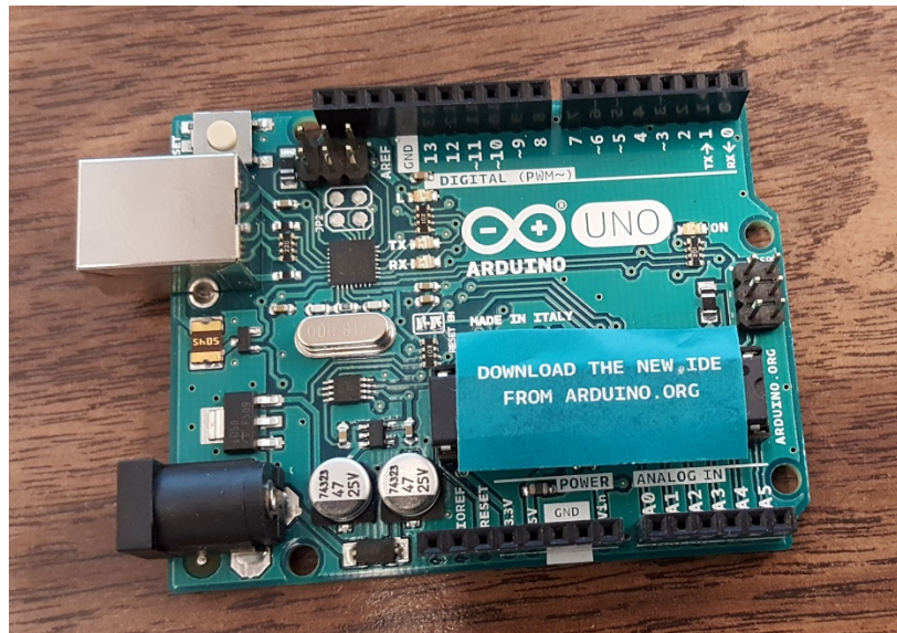
FIG. 3. An Arduino Uno. This unit comes ready to be programmed with female header pins for easy connection to any project.
