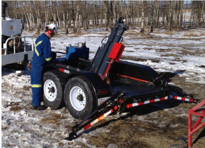
FIG. 1. Where the operator has to stand to run the thumper from the built in switch panel.
