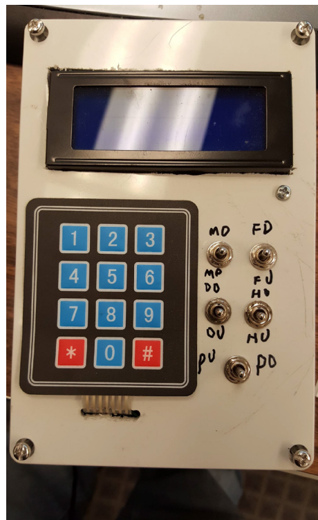
FIG. 7. The controller for the thumper. Each of the switches controls two of the hydraulic valves. The number pad is for entering shot information to be loaded on to the SD card and the screen give real time feedback.
