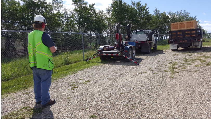
FIG. 8. The thumper being controlled from several metres away.
