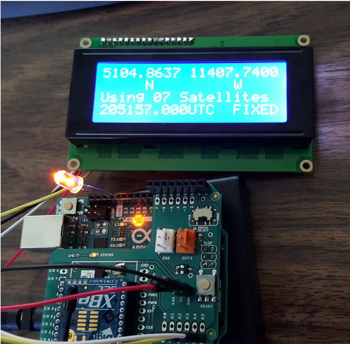
FIG. 5. All the data being displayed on the screen is being transmitted wirelessly from the other microcontroller which is in another room. The LED in this picture is an indication that the GPS has fixed data.
