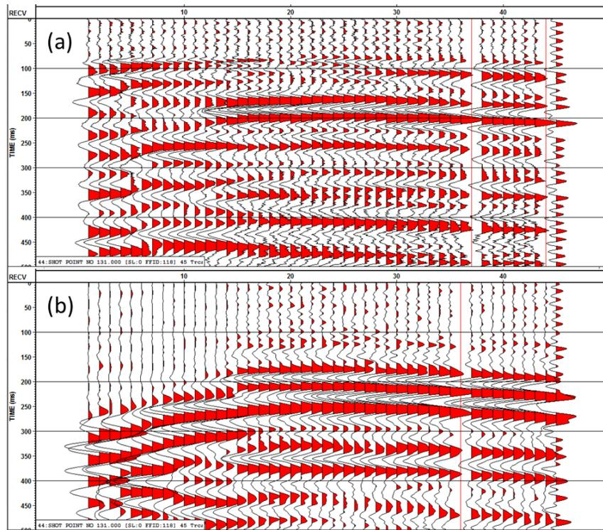
FIG 10. 155 m offset VSP data from the Priddis Geophysical Observatory well. (a) Vertical component data {P-wave}. (b) Cross-line horizontal component data {SH-wave}.
