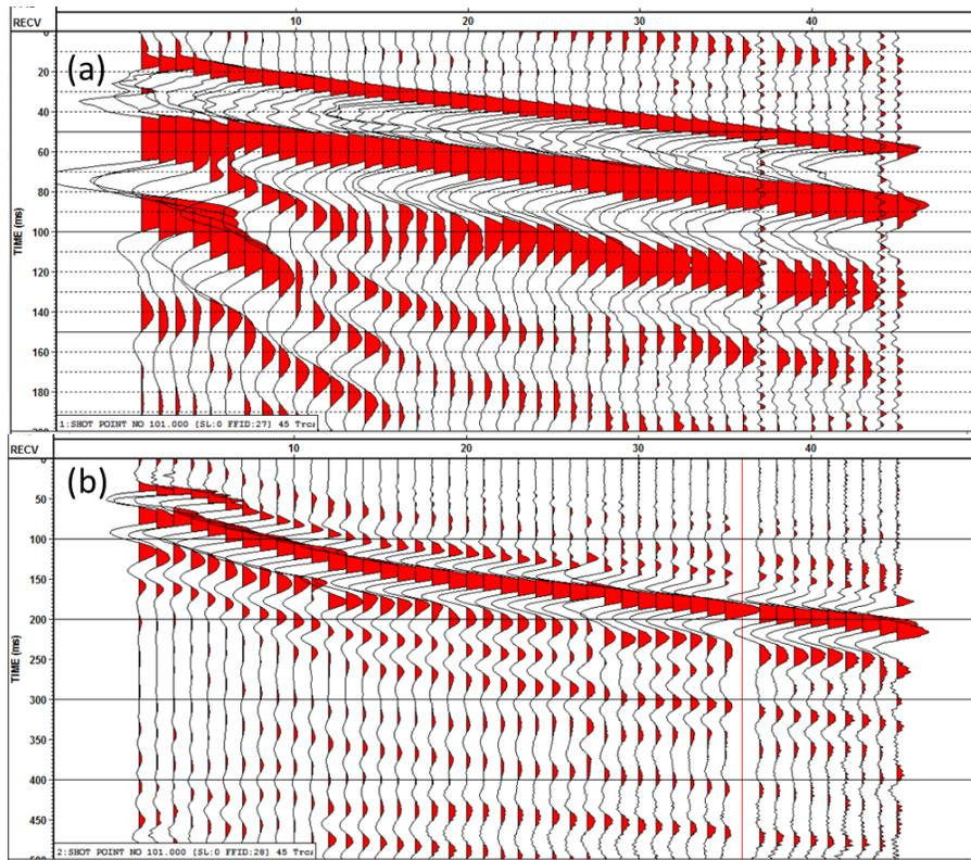
FIG 7. Zero offset VSP data from the Priddis Geophysical Observatory well. (a) Vertical component data {P-wave}. (b) Cross-line horizontal component data {SH-wave}.
