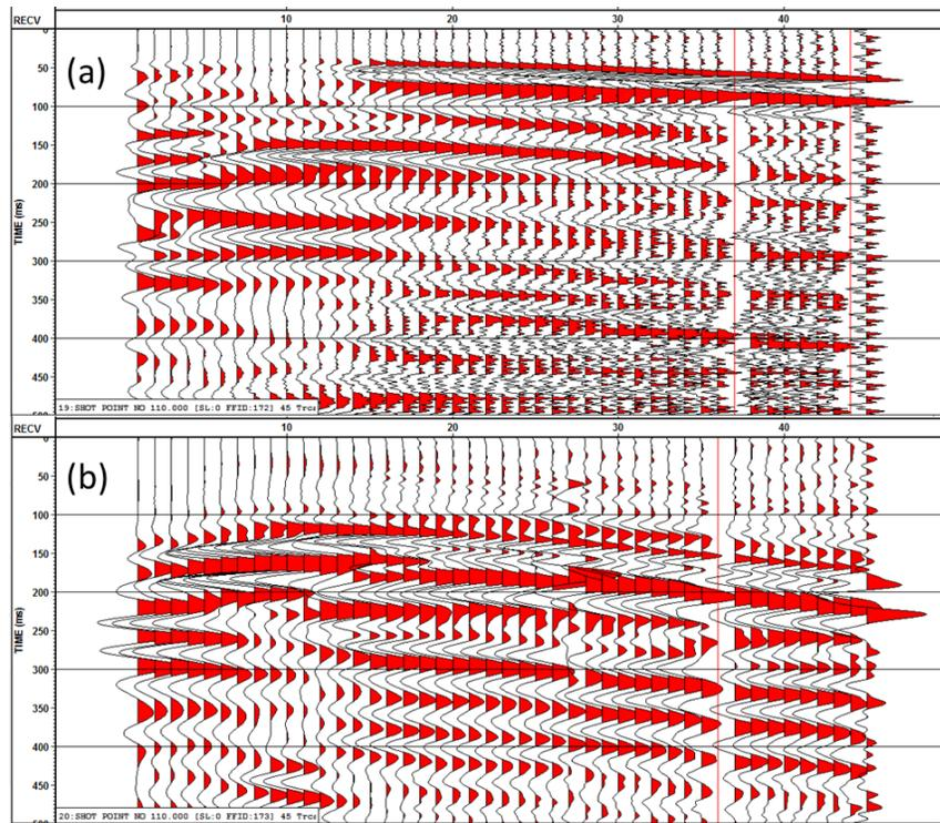
FIG 8. 50 m offset VSP data from the Priddis Geophysical Observatory well. (a) Vertical component data {P-wave}. (b) Cross-line horizontal component data {SH-wave}.
