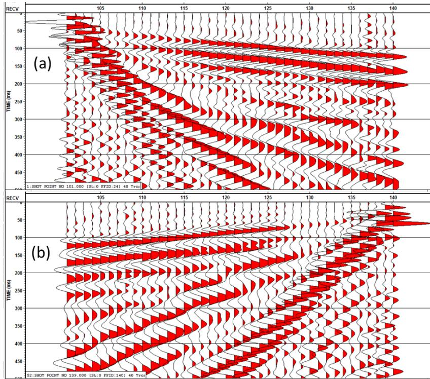
FIG. 5. P-wave end-shots from the surface 3C receiver line.
