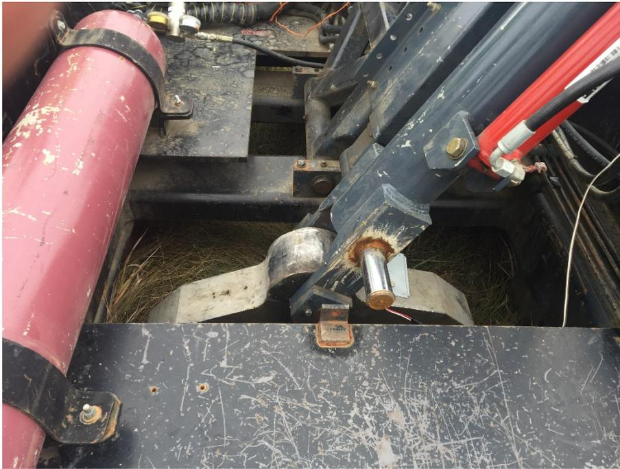
FIG. 3. Source hammer operating in S-wave mode.
