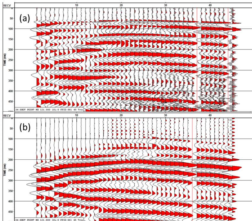
FIG 9. 105 m offset VSP data from the Priddis Geophysical Observatory well. (a) Vertical component data {P-wave}. (b) Cross-line horizontal component data {SH-wave}.
