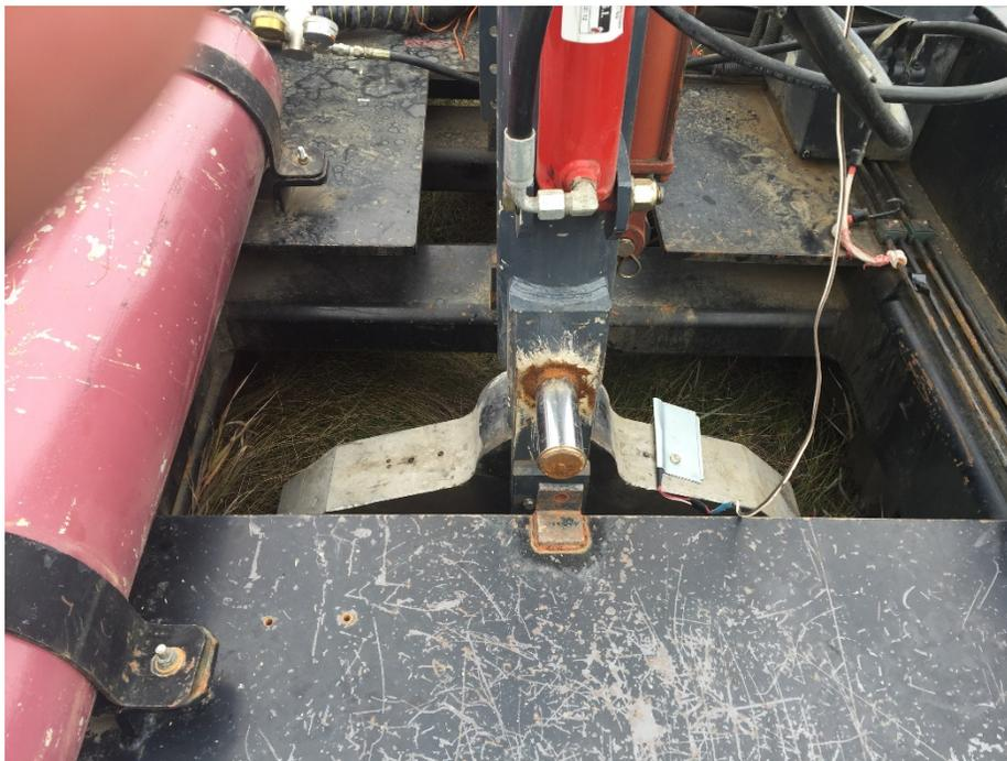
FIG. 4. Source hammer operating in S-wave mode
