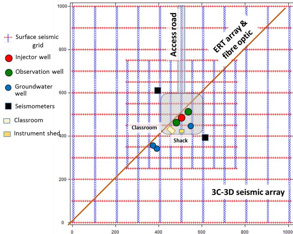
FIG 12. Layout of the CaMI Field Research Station near Brooks, Alberta.
