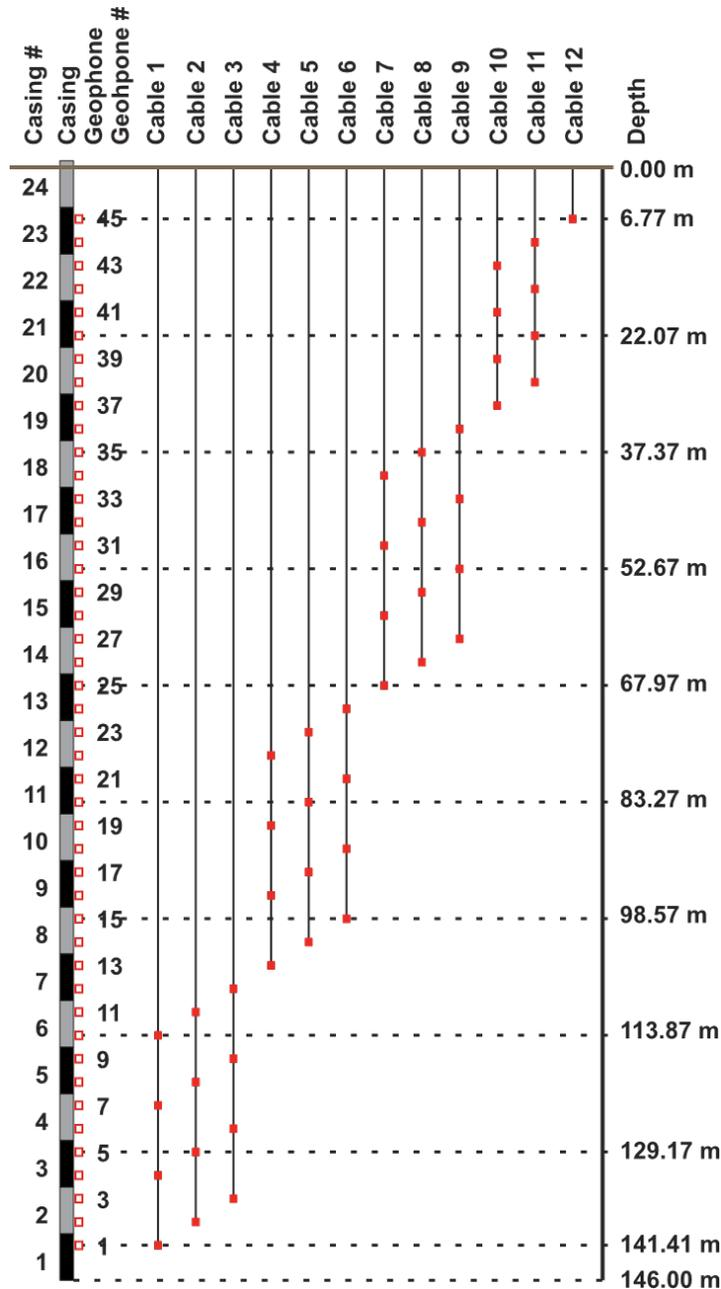
FIG 1. Layout of VSP cable and geophones (from Hall et al., 2013)
