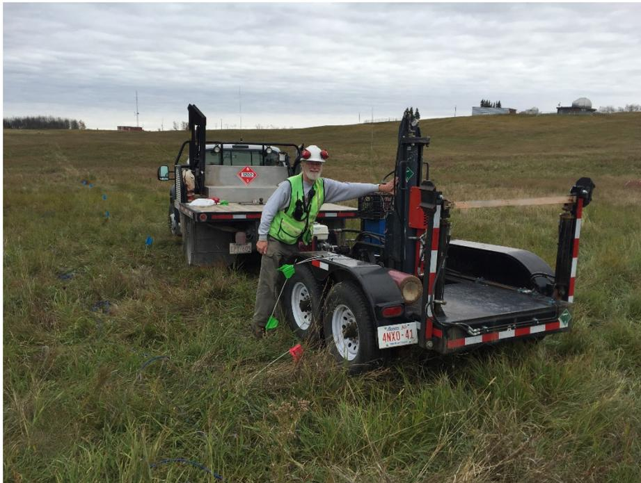
FIG 2. Thumper seismic source in vertical force mode. Malcolm Bertram operating.
