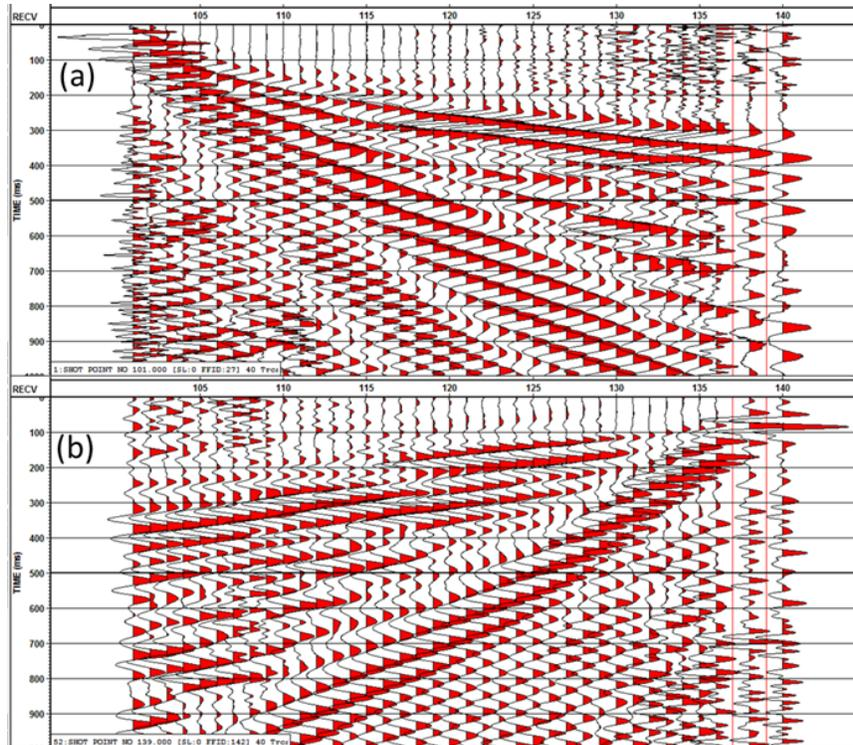
FIG. 6. SH-wave end-shots from the surface 3C receiver line.
