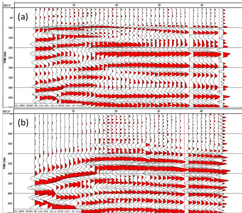
FIG 11. 195 m offset VSP data from the Priddis Geophysical Observatory well. (a) Vertical component data {P-wave}. (b) Cross-line horizontal component data {SH-wave}.
