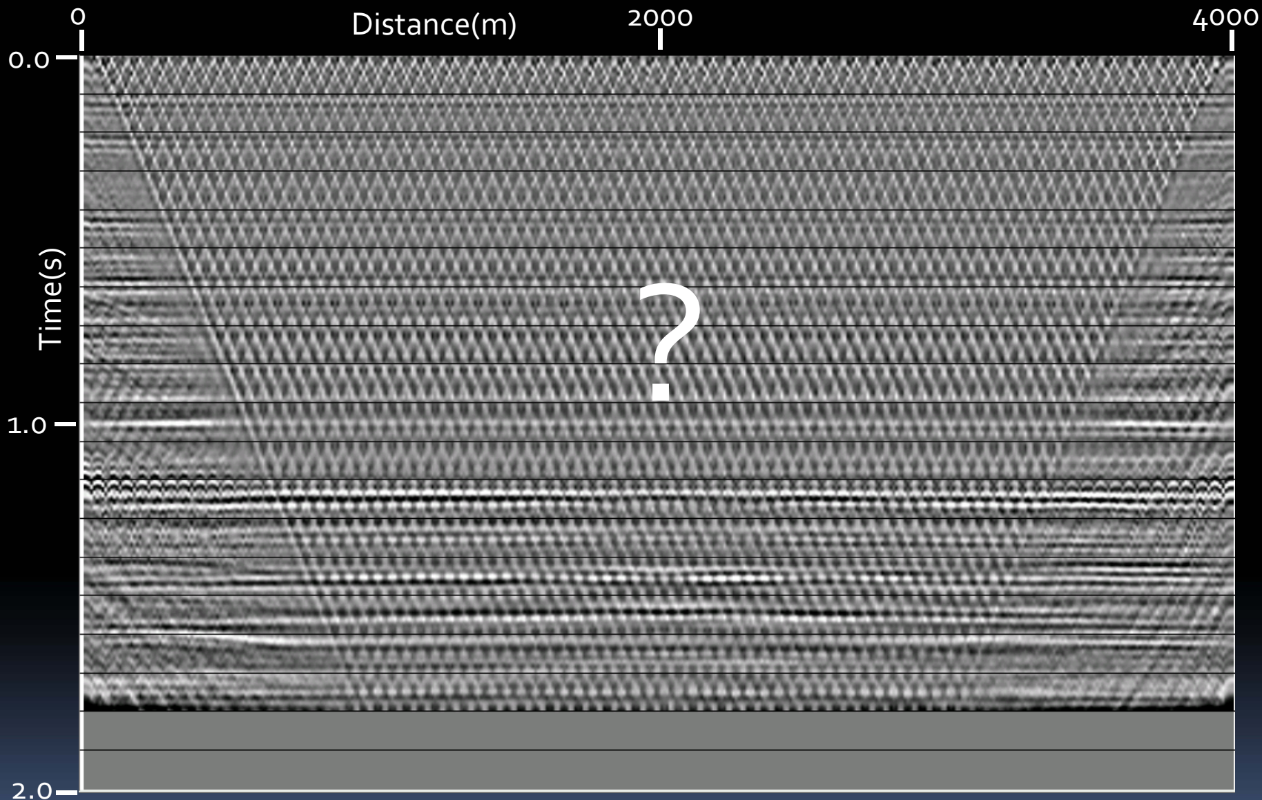
CMP stack for 'E'— surface waves dominant
