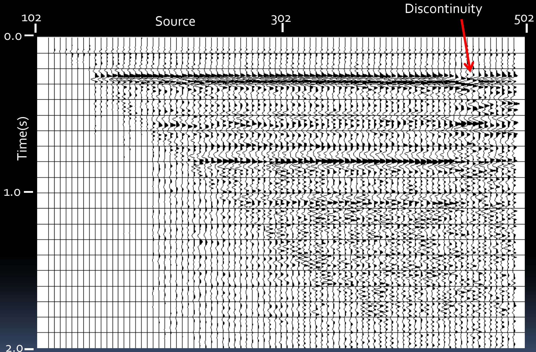
'B' common ray-parameter panel at -1504m/s after two passes of spiking decon
