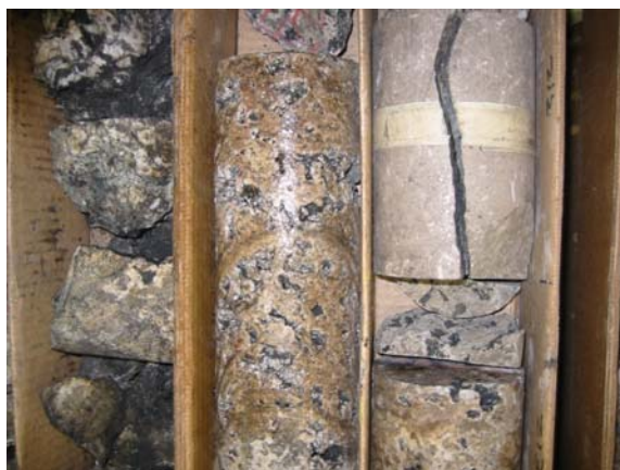
Figure 6. Photograph of core from well 7-10. Porosity type seen here, from left to right, is zebroidal, vuggy, and intercrystalline. Average porosity is 8%.
